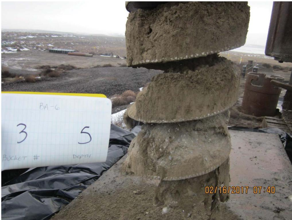
IMG\_5967: Recovery 4 to 5 ft bgs. Piece of Geotextile recovered on bottom flight of auger.
