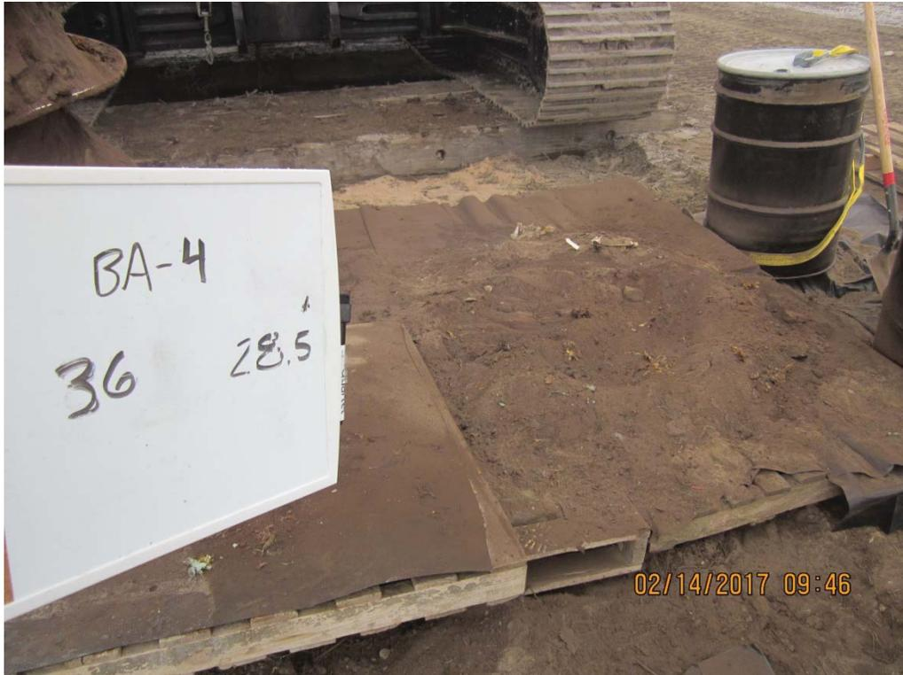
IMG\_5747: Recovery 26 to 28.5 ft bgs. Pass No. 1. (5/15)
