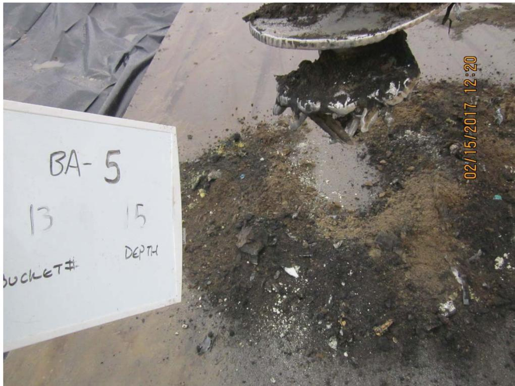
IMG\_5938: Recovery 14 to 15 ft bgs. Spread by Driller's assistant for inspection. (3/3)
