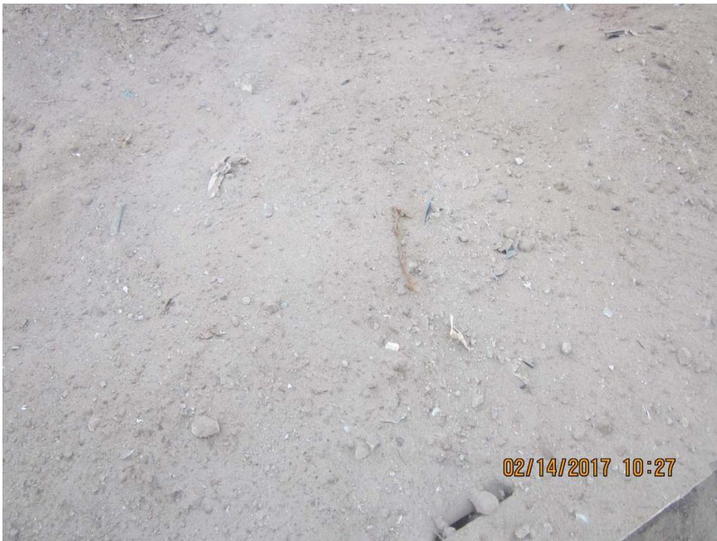
IMG\_5764: Recovery 26 to 28.5 ft bgs. Pass No. 2. (14/15)
