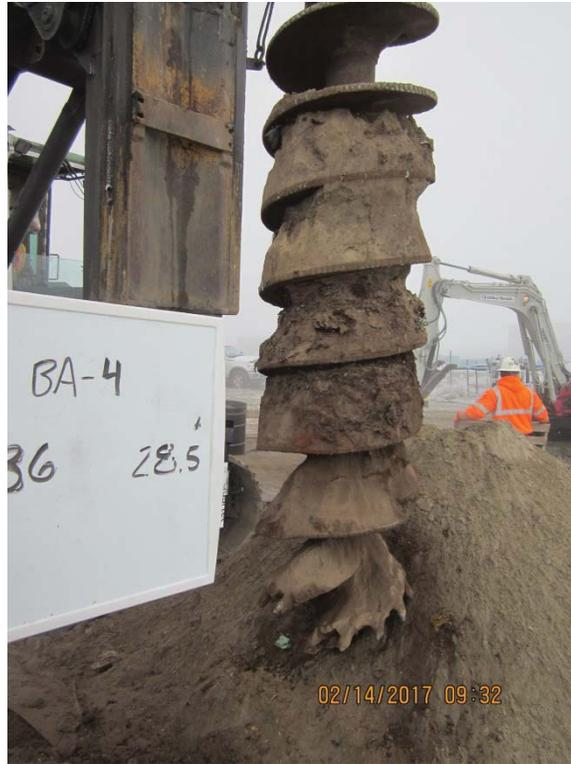
**IMG\_5743:** Recovery 26 to 28.5 ft bgs. Pass No. 1. (1/15)
