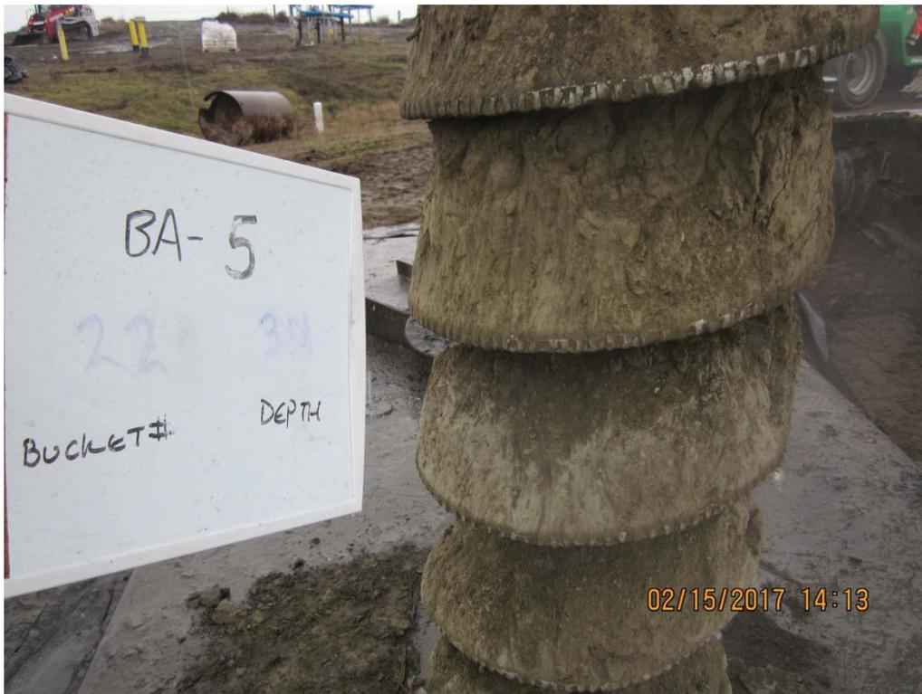
IMG\_5959: Recovery 32 to 34 ft bgs. Bottom of boring.
