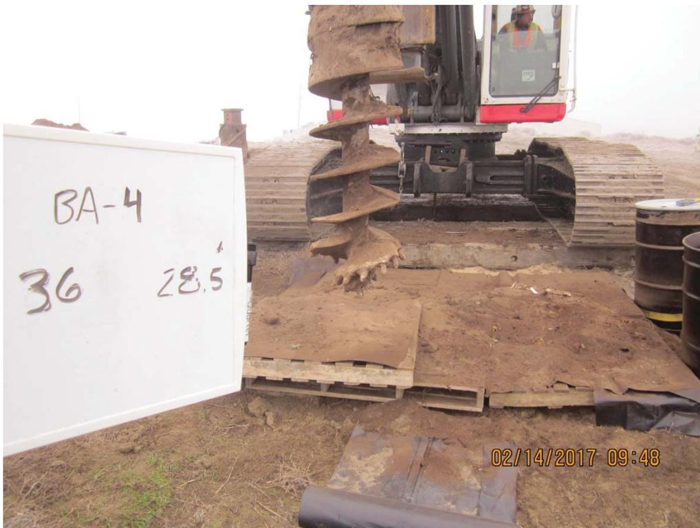
IMG\_5748: Recovery 26 to 28.5 ft bgs. Pass No. 1. (6/15)
