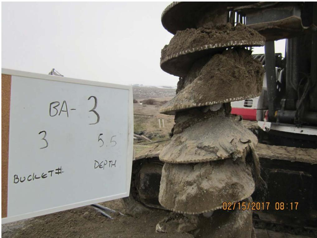
IMG\_5883: Recovery 3.5 to 5.5 ft bgs. Piece of Geotextile recovered on auger.
