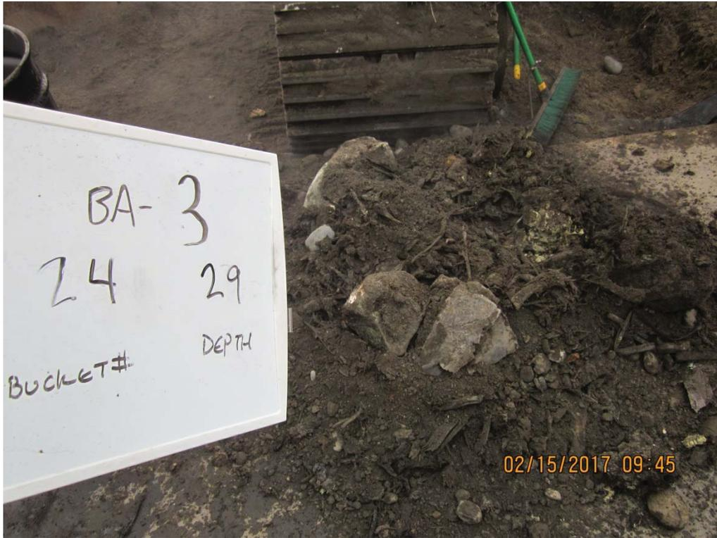
IMG\_5907: Recovery 27.5 to 29 ft bgs. Fragments of boulder and wood debris encountered. (2/2)
