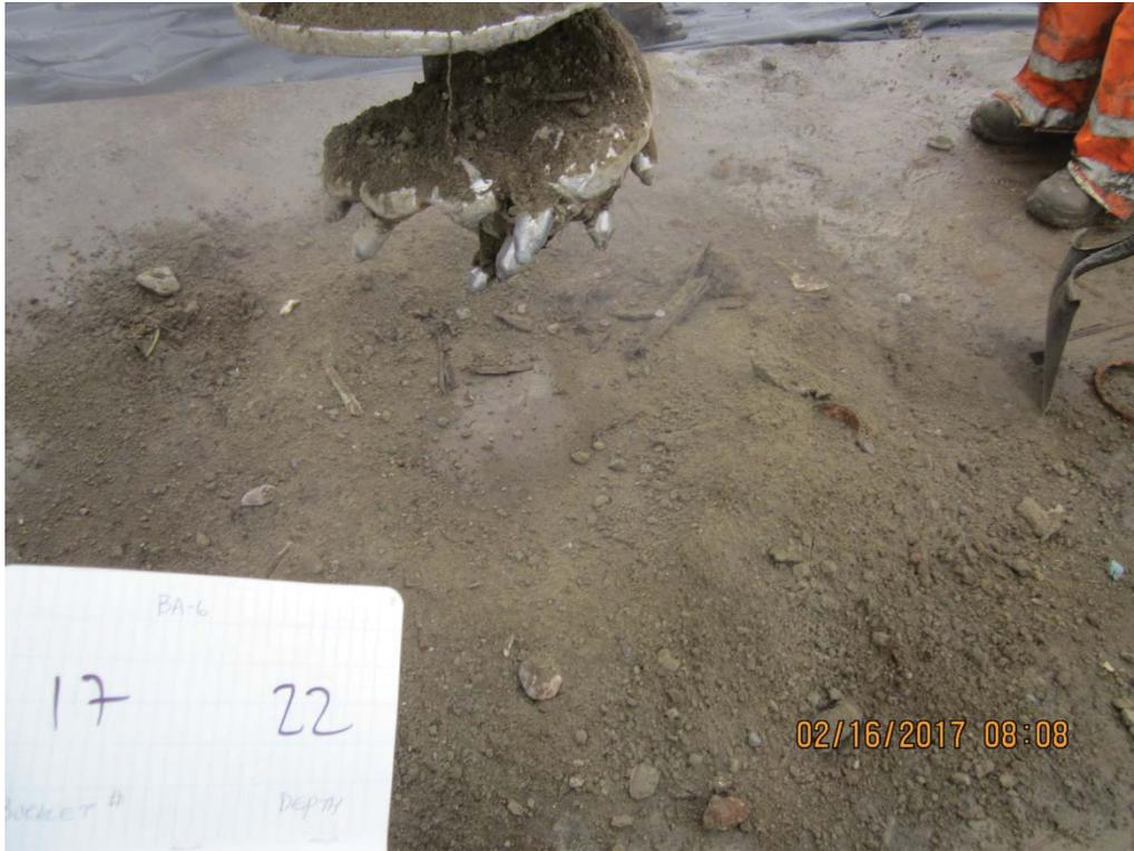
IMG\_5984: Recovery 20 to 22 ft bgs. Spread for inspection by Driller's assistant. (3/3)
