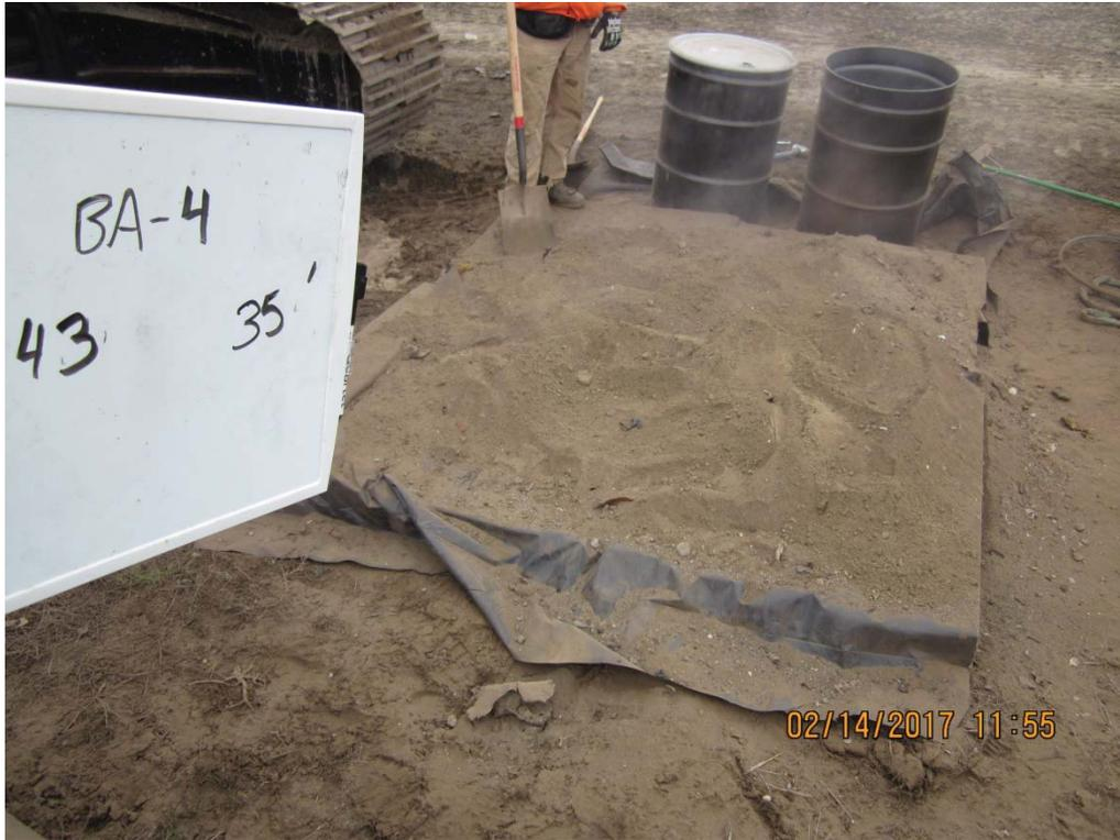
IMG\_5803: Recovery 33.5 to 35 ft bgs. Bottom of boring. (4/4)
