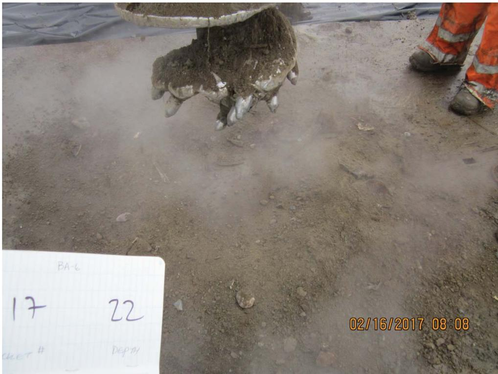
IMG\_5983: Recovery 20 to 22 ft bgs. Spread for inspection by Driller's assistant. (2/3)
