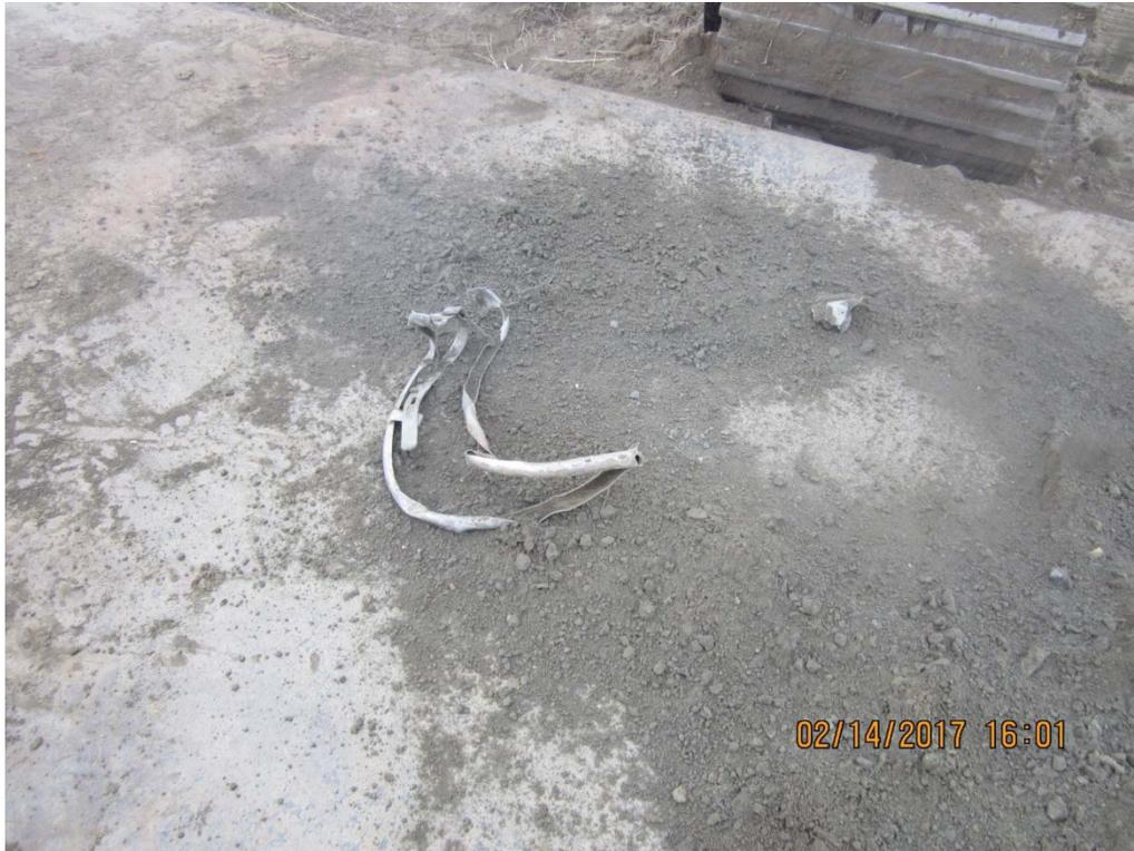
**IMG\_5873:** Recovery 35 to 36.5 ft bgs. Spread for inspection by Driller's assistant. Three (3) large metal pieces recovered.
