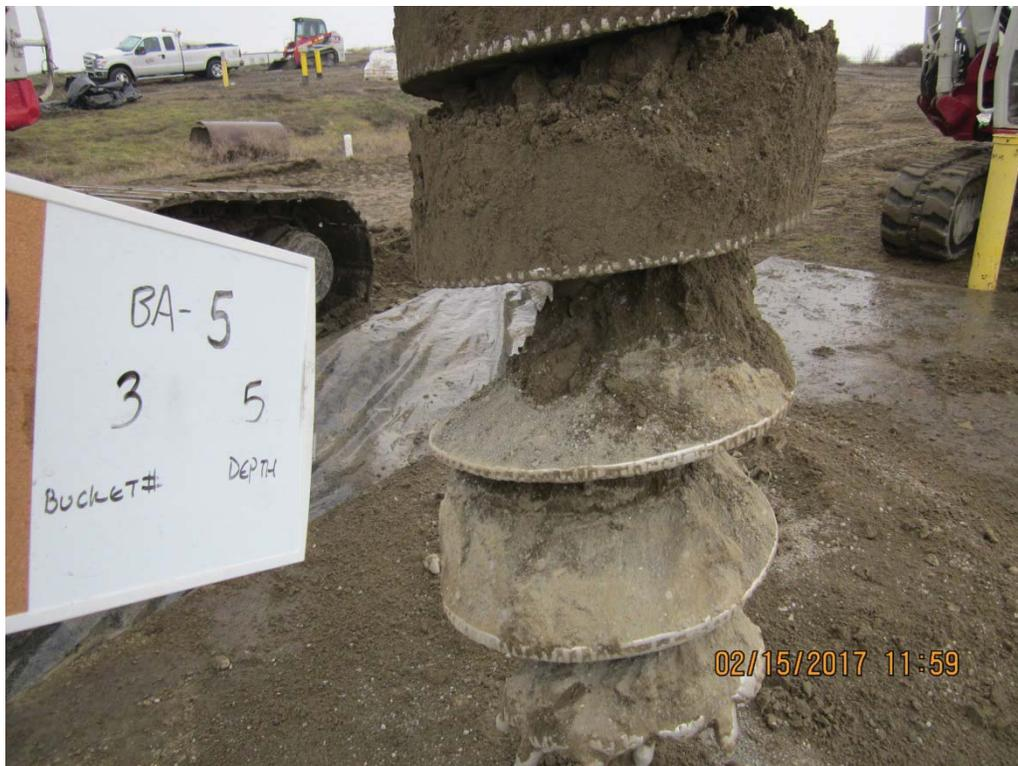
IMG\_5926: Recovery 4 to 5 ft bgs. Pass No. 2. (3/4)
