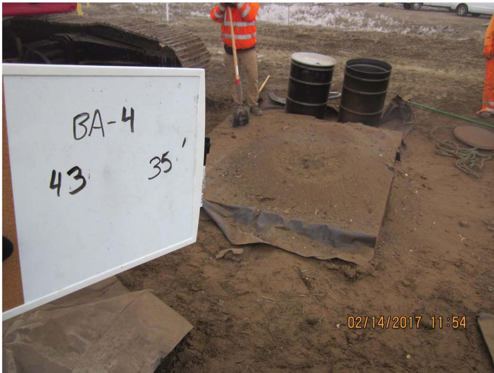
IMG\_5802: Recovery 33.5 to 35 ft bgs. Bottom of boring. (3/4)
