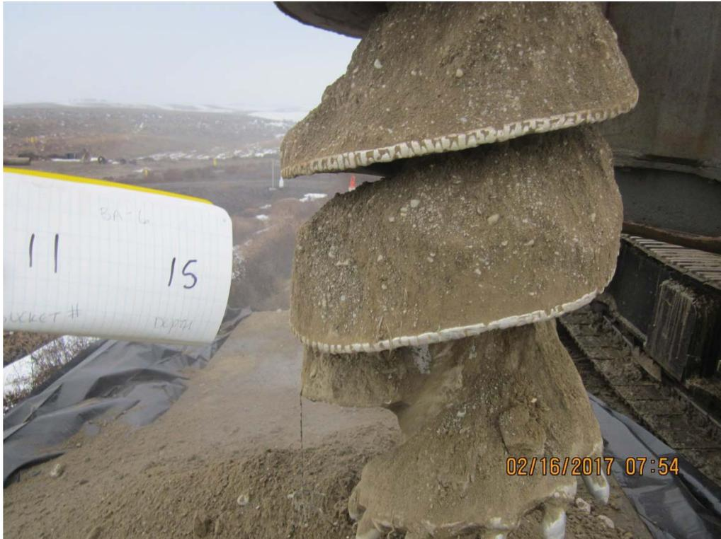
IMG\_5976: Recovery 12 to 15 ft bgs. Pieces of Geonet and Geotextile recovered.
