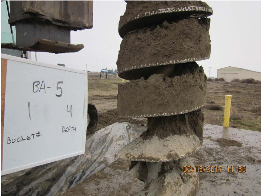
IMG\_5923: Recovery 0 to 4 feet (ft) below ground surface (bgs.).
