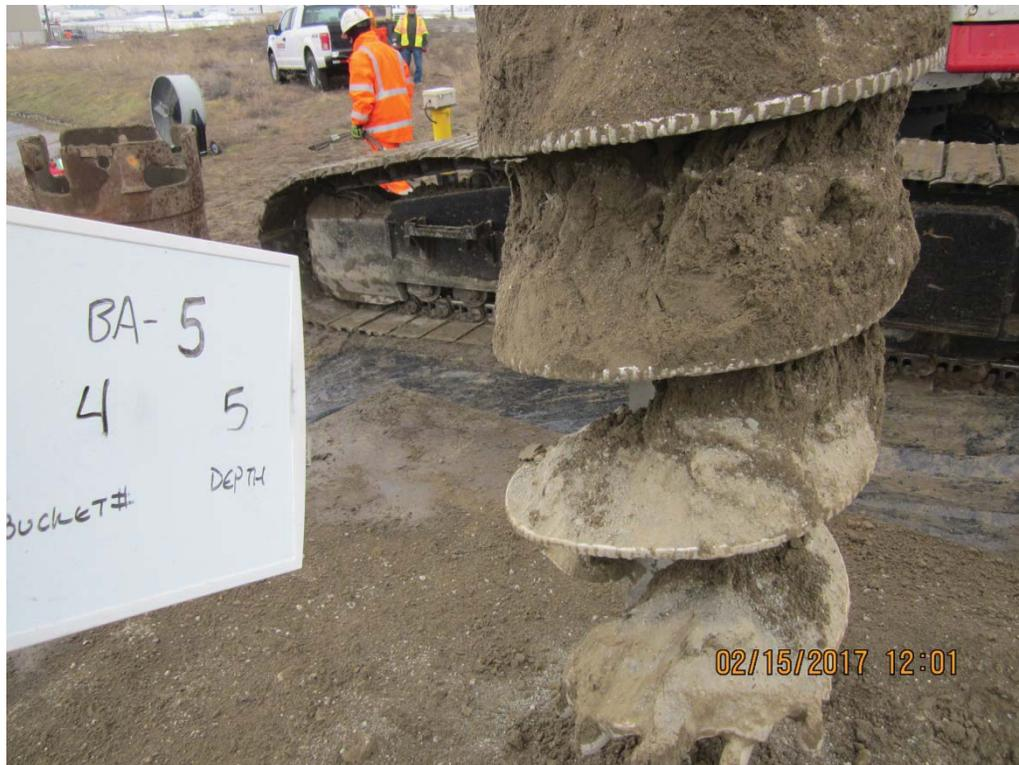
IMG\_5927: Recovery 4 to 5 ft bgs. Pass No. 3 (4/4)
