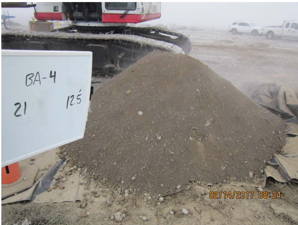
IMG\_5706: Recovery 11 to 12.5 ft bgs. Pass No. 4. (8/8)
