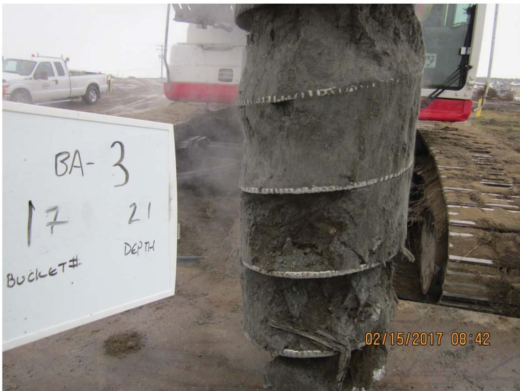
IMG\_5892: Recovery 19.5 to 21 ft bgs. Wood debris recovered on bottom flights of auger. (1/2)
