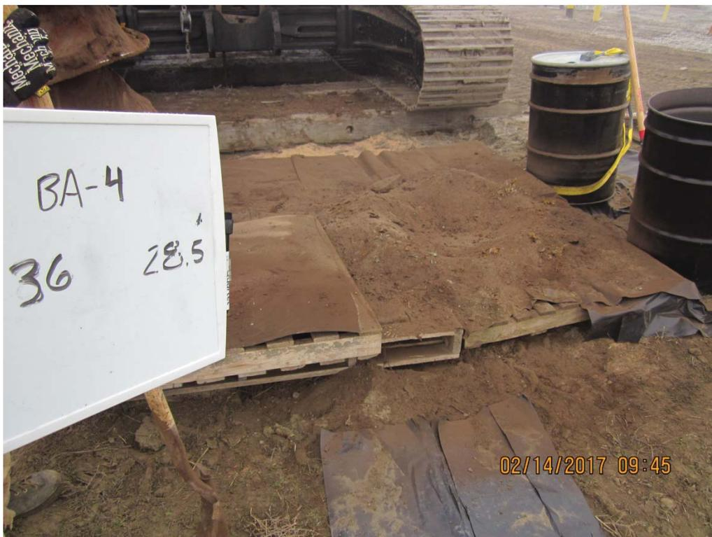
IMG\_5746: Recovery 26 to 28.5 ft bgs. Pass No. 1. (4/15)
