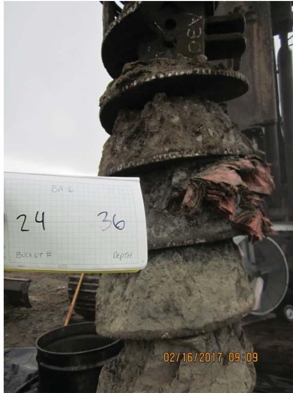
**IMG\_5999:** Recovery 34 to 36 ft bgs. Bottom of boring. (2/4)
