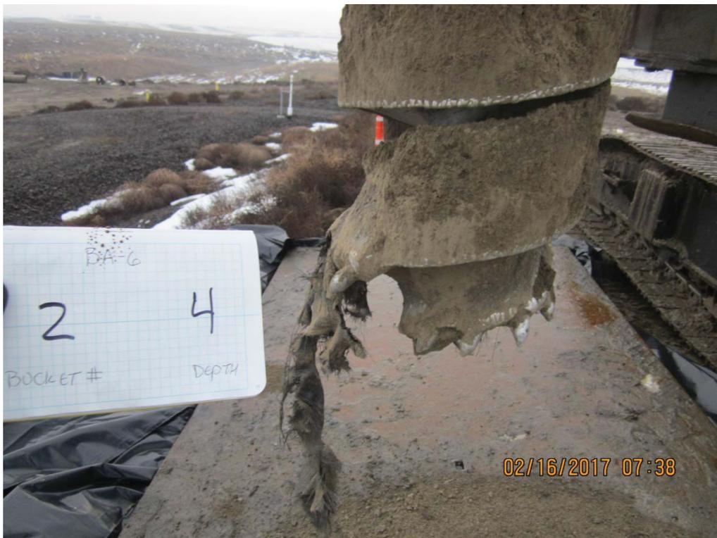
**IMG\_5966:** Recovery 3 to 4 ft bgs. Piece of Geonet recovered on bottom flight of auger. (2/2)
