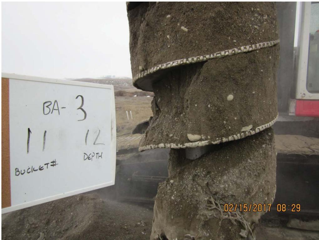
**IMG\_5887:** Recovery 8 to 12 ft bgs. Pieces of Geotextile and Geonet recovered on bottom flight of auger.
