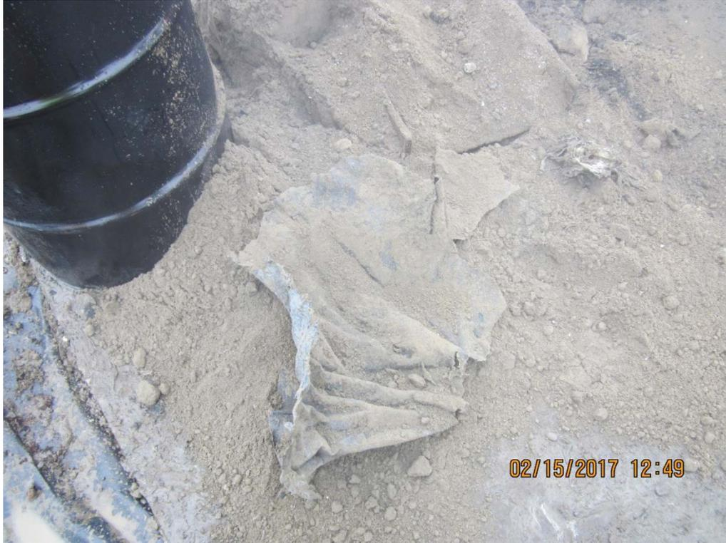
IMG\_5943: Recovery 17 to 18 ft bgs. Piece of Geomembrane recovered. (3/4)
