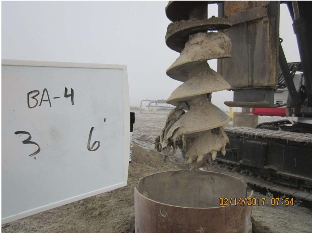
IMG\_5669: Recovery 5 to 6 ft bgs. Piece of Geomembrane recovered. (1/2)
