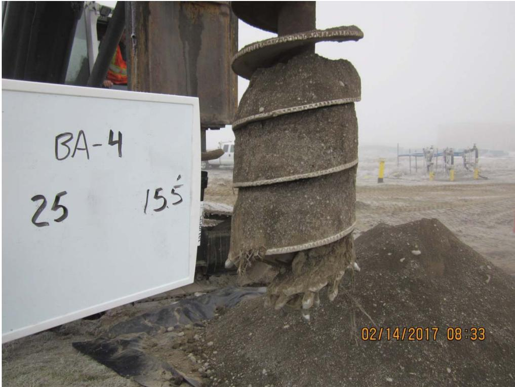
**IMG\_5713:** Recovery 14 to 15.5 ft bgs. Piece of Geogrid recovered on bottom flight of auger. (1/3)
