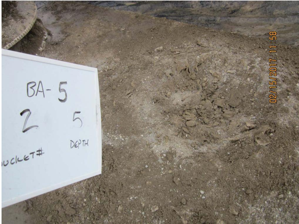
IMG\_5925: Recovery 4 to 5 ft bgs. Pass No. 1. Spread for inspection by Driller's assistant. (2/4)
