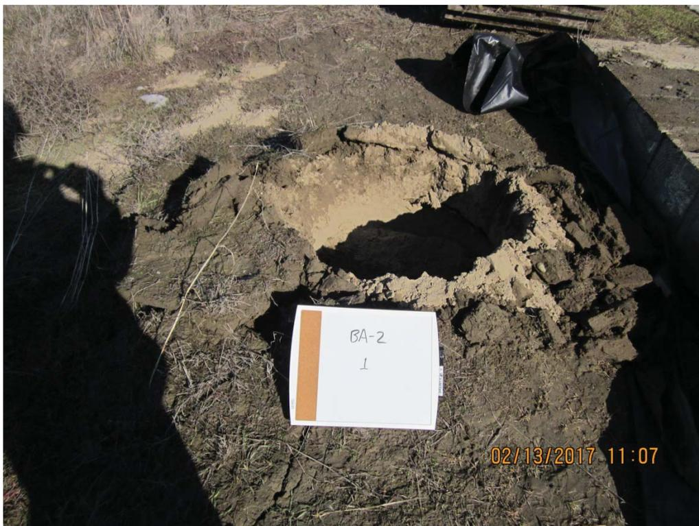
IMG\_5564: Open boring after initial pass. Geomembrane visible in boring. Depth of boring 1 foot (ft) below ground surface (bgs).
