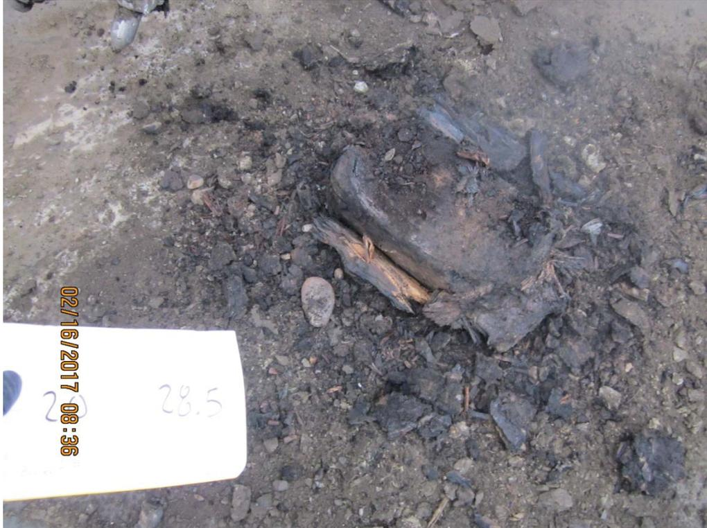
IMG\_5990: Recovery 26 to 28.5 ft bgs. Wood debris recovered. (1/3)
