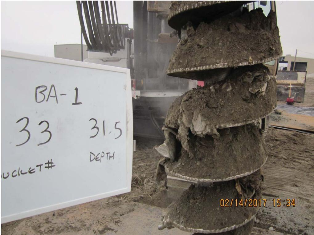
**IMG\_5858:** Recovery 32 to 33 ft bgs. Pass No. 2. Lost depth of boring from previous passes due to slough within boring. (1/2)
