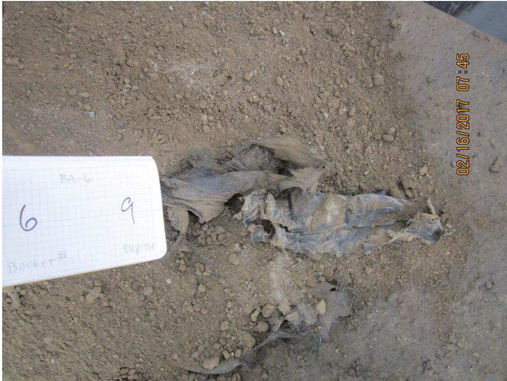
IMG\_5971: Recovery 8 to 9 ft bgs. Piece of Geomembrane recovered on bottom flight of auger. (2/2)
