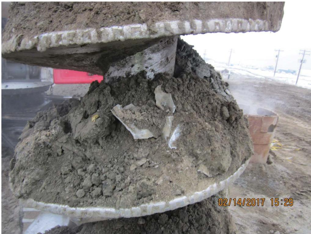
IMG\_5855: Recovery 32 to 33 ft bgs. Pass No. 1. Metal fragments recovered. (1/2)
