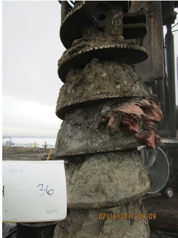
**IMG\_6001:** Recovery 34 to 36 ft bgs. Bottom of boring. (4/4)
