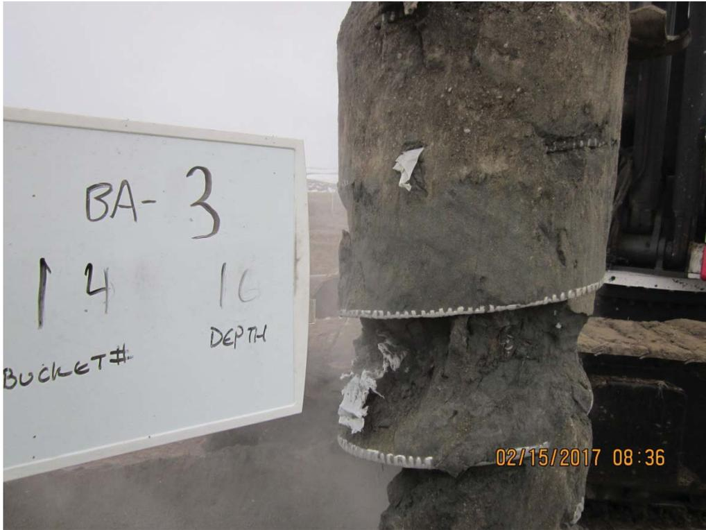
IMG\_5889: Recovery 15 to 16 ft bgs. Pieces of Visqueen (white) recovered on the auger.
