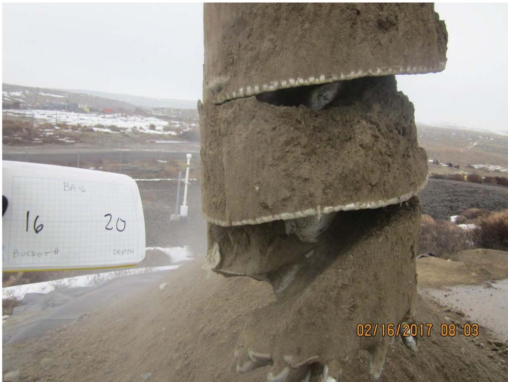
IMG\_5981: Recovery 19 to 20 ft bgs. Pieces of Visqueen (white) recovered on auger.
