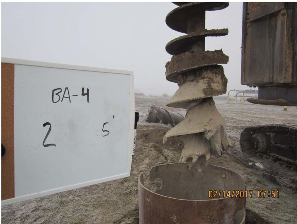
IMG\_5666: Recovery 4.5 to 5 ft bgs. Piece of Geotextile recovered on auger. (1/3).
