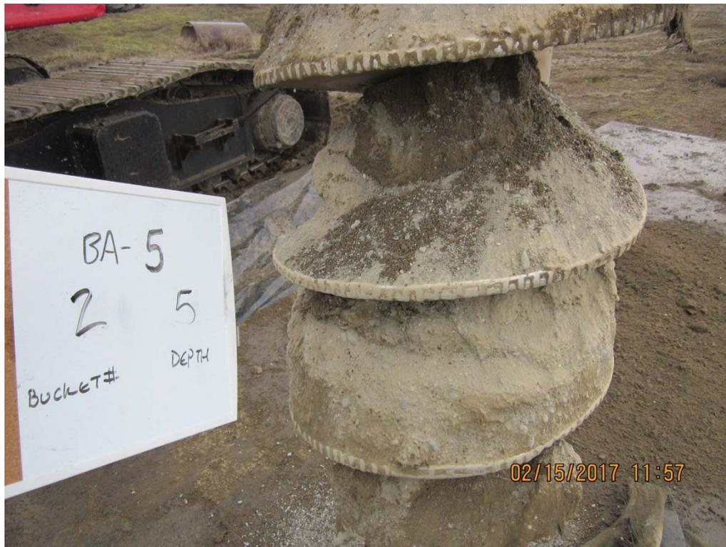
IMG\_5924: Recovery 4 to 5 ft bgs. Pass No. 1. (1/4)
