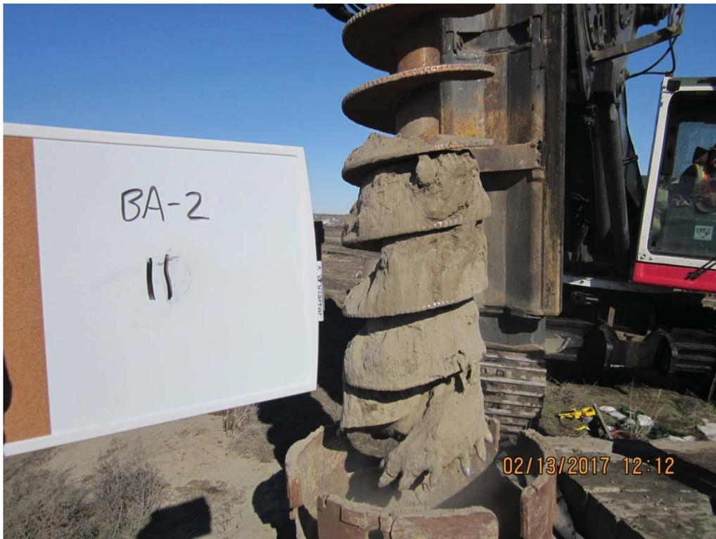
IMG\_5583: Recovery 5 to 7 ft bgs. Piece of Geomembrane visible. (1/2)
