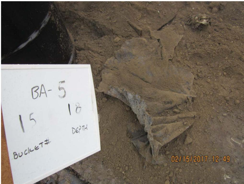
IMG\_5944: Recovery 17 to 18 ft bgs. Piece of Geomembrane recovered. (4/4)
