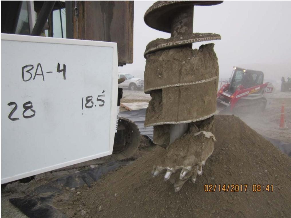
**IMG\_5719:** Recovery 17.5 to 18.5 ft bgs. Piece of Visqueen (white) recovered on bottom flight of auger. (1/2)
