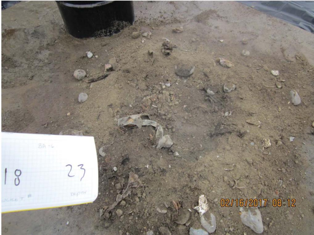
IMG\_5986: Recovery 22 to 23 ft bgs. Spread for inspection by Driller's assistant. (2/3)
