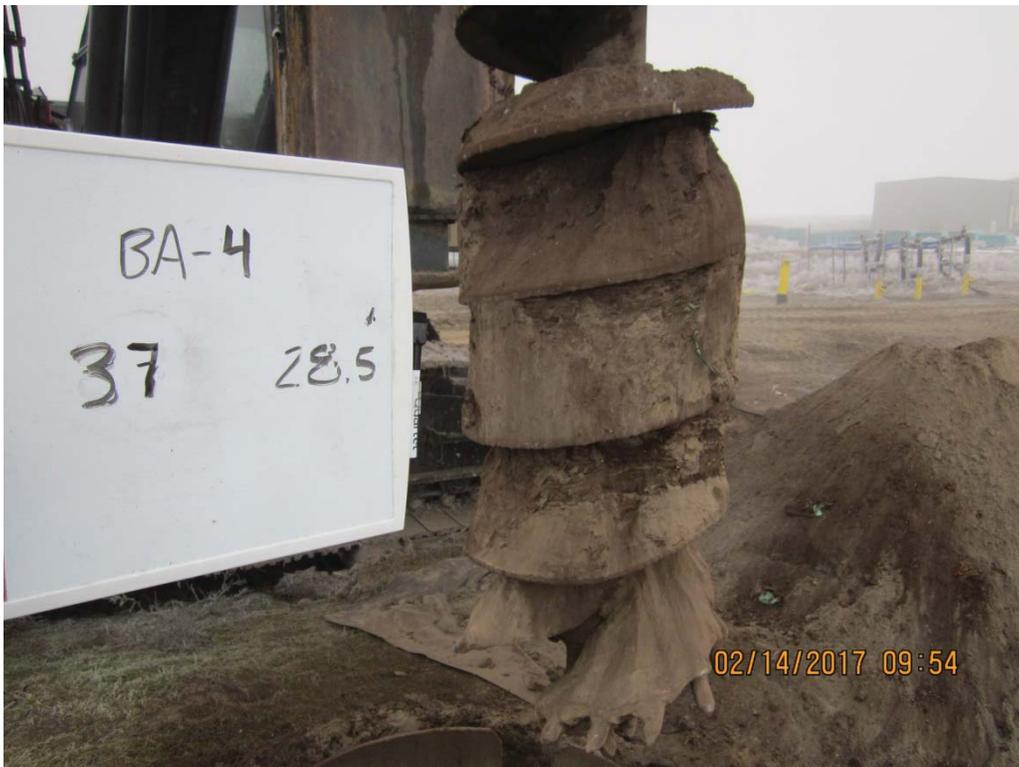
IMG\_5752: Recovery 26 to 28.5 ft bgs. Pass No. 2. (10/15)
