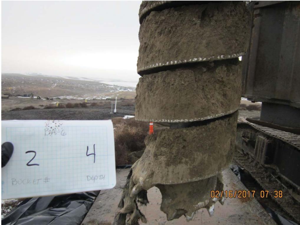
**IMG\_5965:** Recovery 3 to 4 ft bgs. Piece of Geonet recovered on bottom flight of auger. (1/2)
