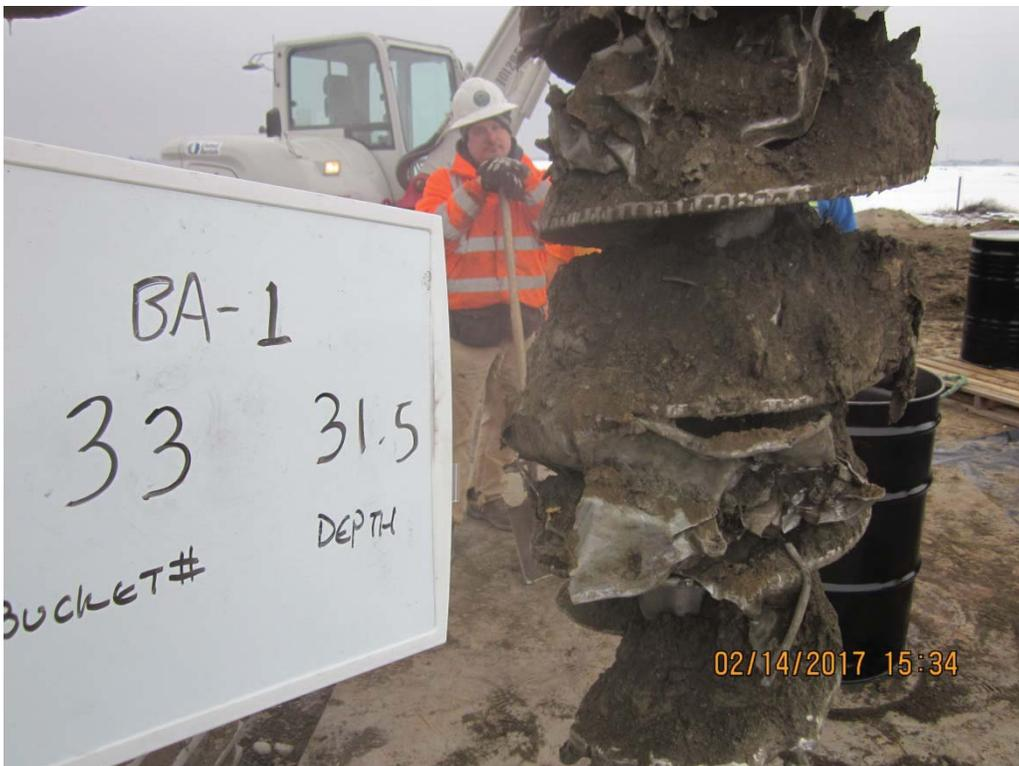
**IMG\_5859:** Recovery 32 to 33 ft bgs. Pass No. 2. Lost depth of boring from previous passes due to slough within boring. (2/2)
