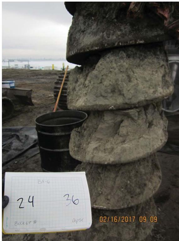
IMG\_5998: Recovery 34 to 36 ft bgs. Bottom of boring. (1/4)
