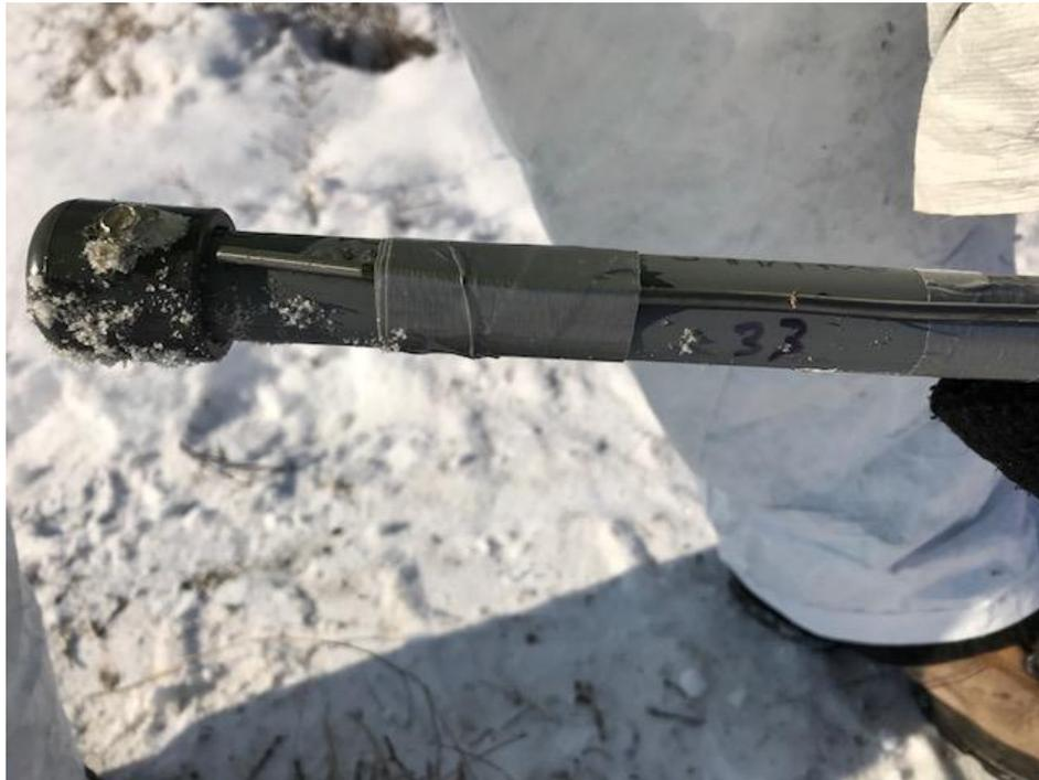
Photograph 1: Typical thermocouple array.
