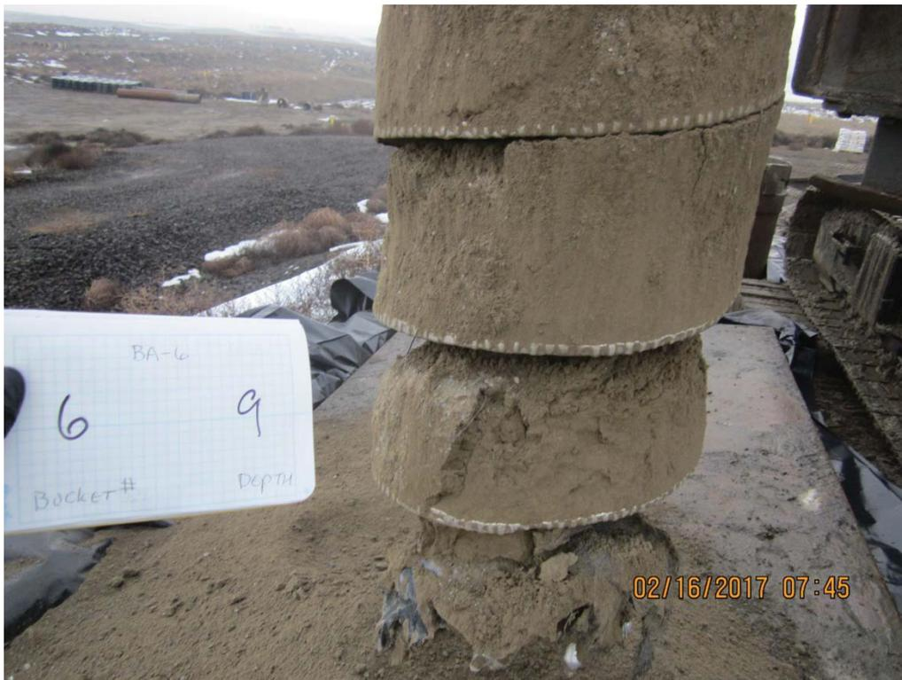
IMG\_5970: Recovery 8 to 9 ft bgs. Piece of Geomembrane recovered on bottom flight of auger. (1/2)
