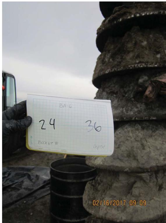
**IMG\_6000:** Recovery 34 to 36 ft bgs. Bottom of boring. (3/4)
