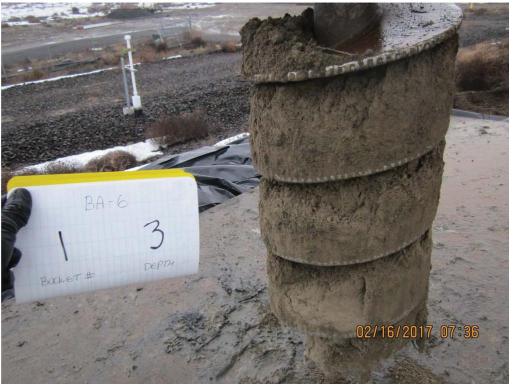
IMG\_5964: Recovery 0 to 3 feet (ft) below ground surface (bgs.).
