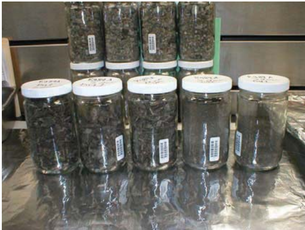
Figure 3: DU 2 Sample fraction not passing 2mm sieve.
