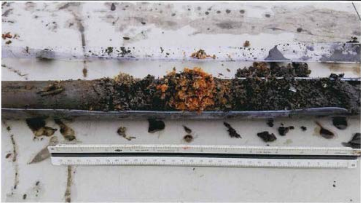
Boring B1 soil core depicting wood-chip fill layer encountered between 4 and 6 feet below the ground surface.
