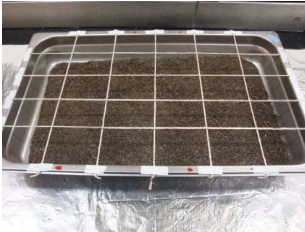
Figure 6: Splitting tray with 30 section grid
