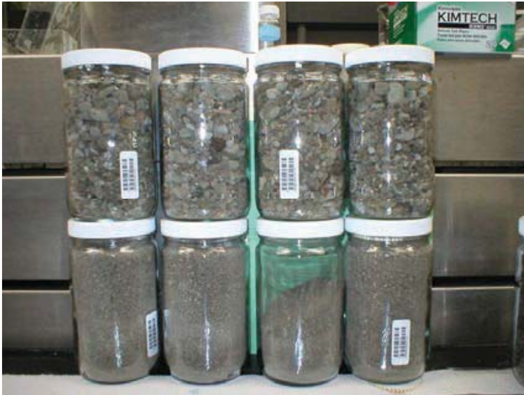
Figure 4: DU 3 Sample fraction not passing 2mm sieve.
