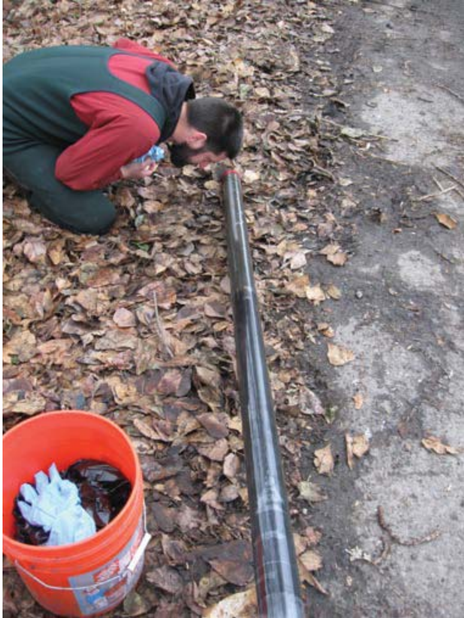
Former West Ditch Core SS-2 with approx. 6 feet of recovered soil
