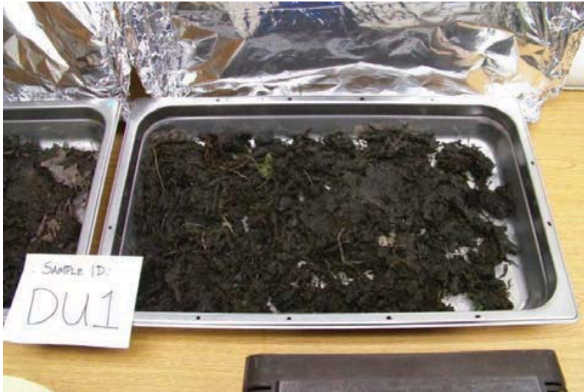
Figure 2: DU 1 Sample fraction not passing 2mm sieve.
