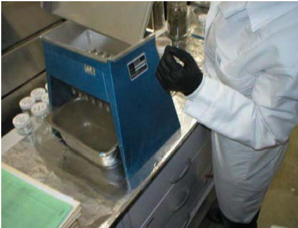
Figure 5: Jones-type or chute riffle splitter
