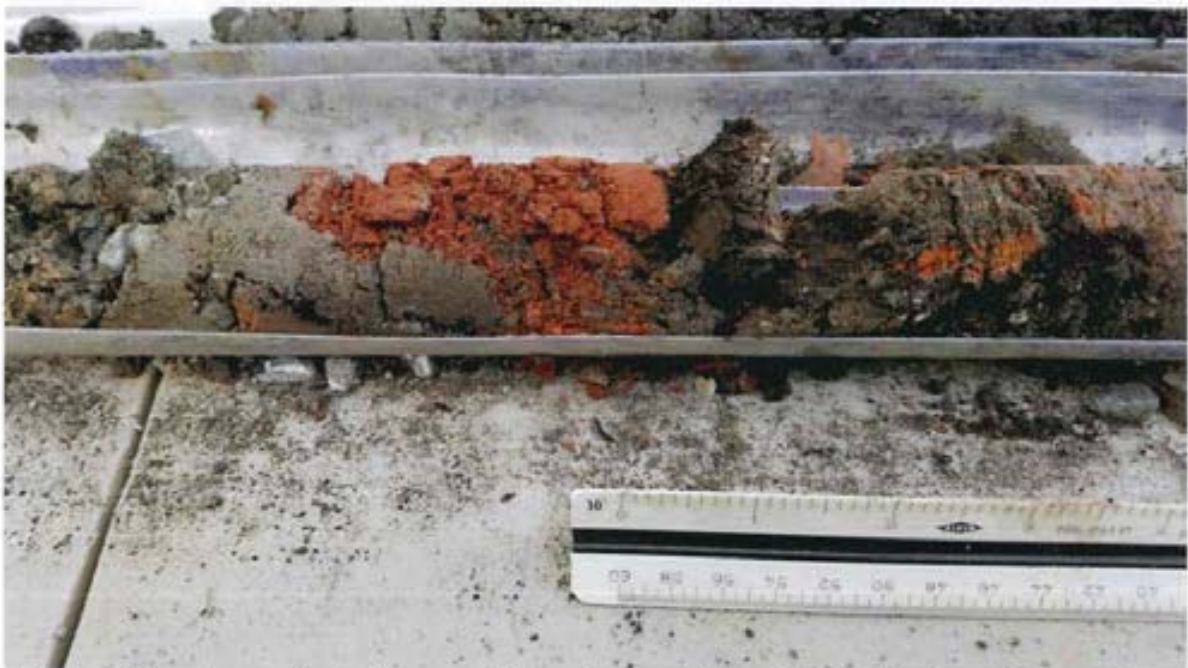
Boring B2 soil core depicting a mixture of wood-chips, brick debris, and organic silts.
