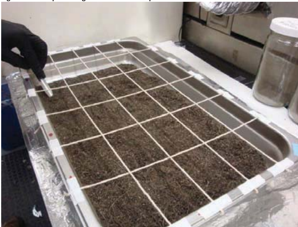
Figure 8: Grid sub-section sampling
