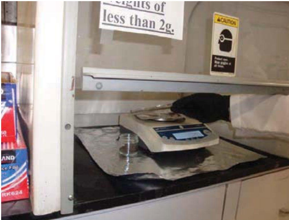
Figure 9: Checking the mass of each grid sub-section sample
