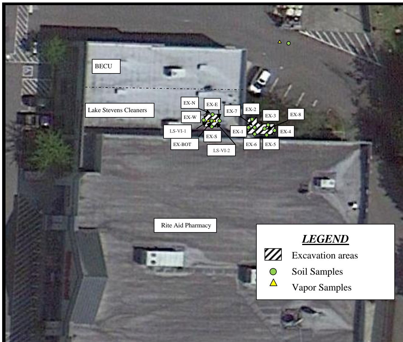
FIGURE 4-1 — POST EXCAVATION SOIL AND VAPOR SAMPLE MAP
