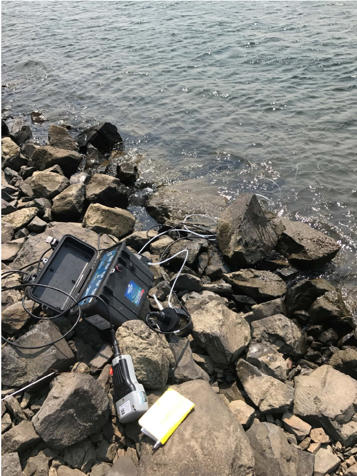
Photograph 3: PushPoint groundwater sampling
