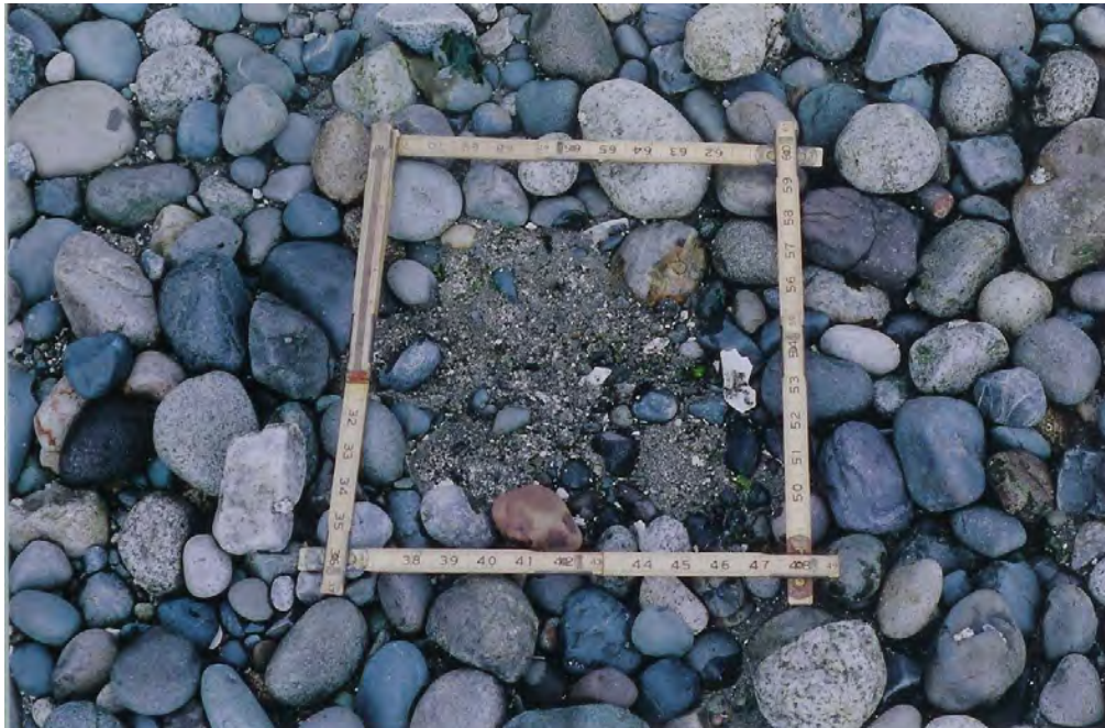
Figure 8. Representative type of material that may be used for construction of south gravel cobble beach
