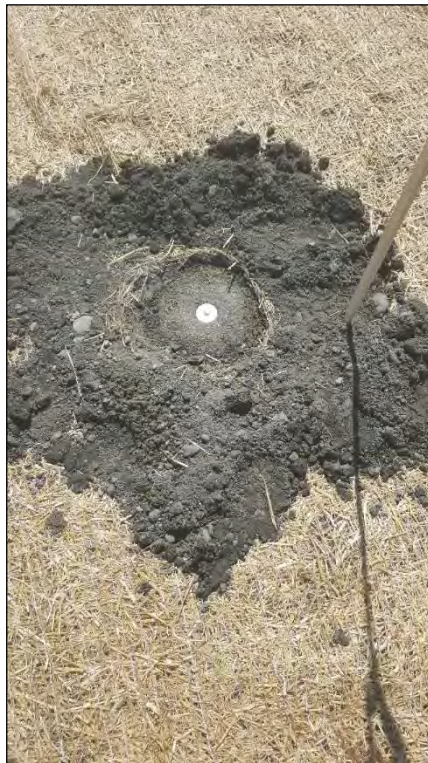
30. Settlement survey monument installed on top of stockpile.
