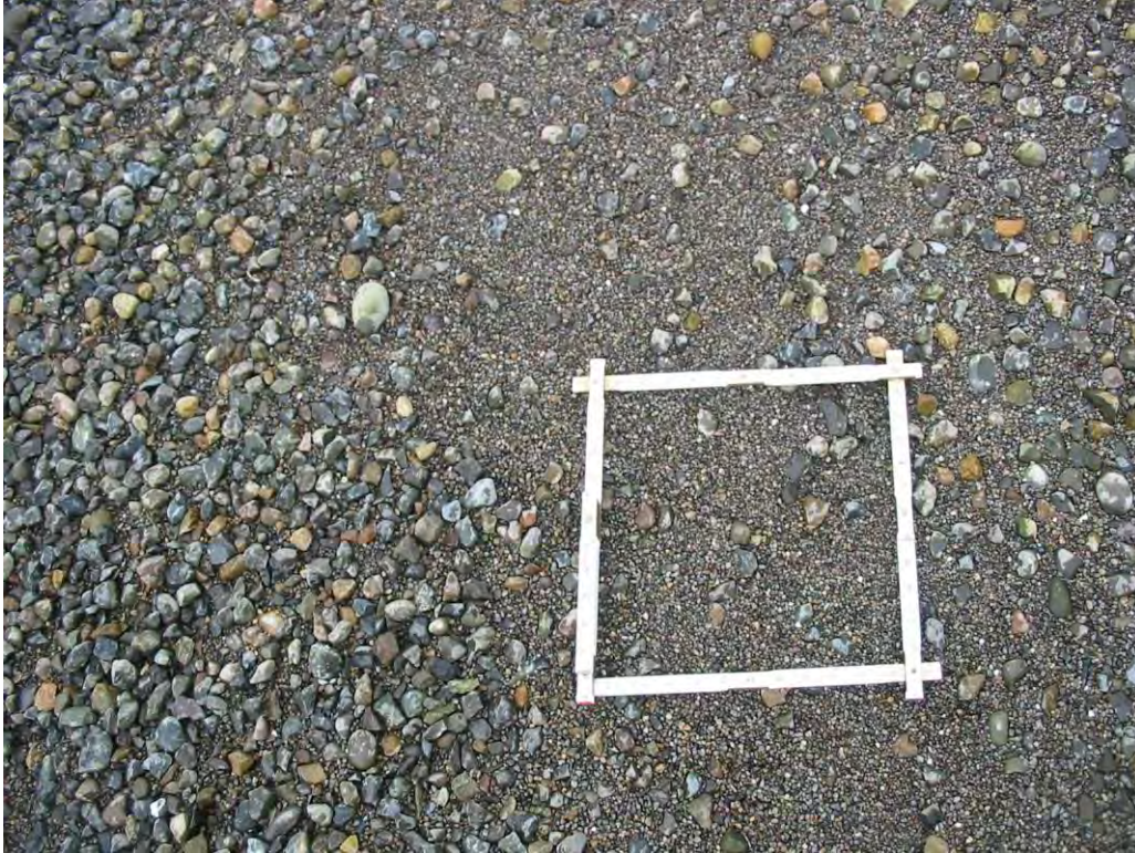
Figure 10. Representative type of material that may be used for construction of sandy gravel beach at this part of shoreline
