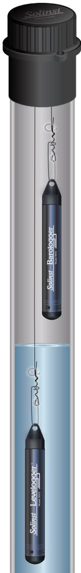
Figure 10-12 Levellogger and Barologger in Well
