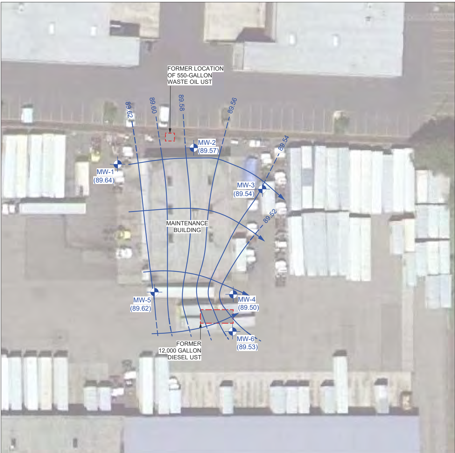
FIGURE 3 JUNE 21, 2016 GROUNDWATER ELEVATIONS AND FLOW DIRECTIONS
