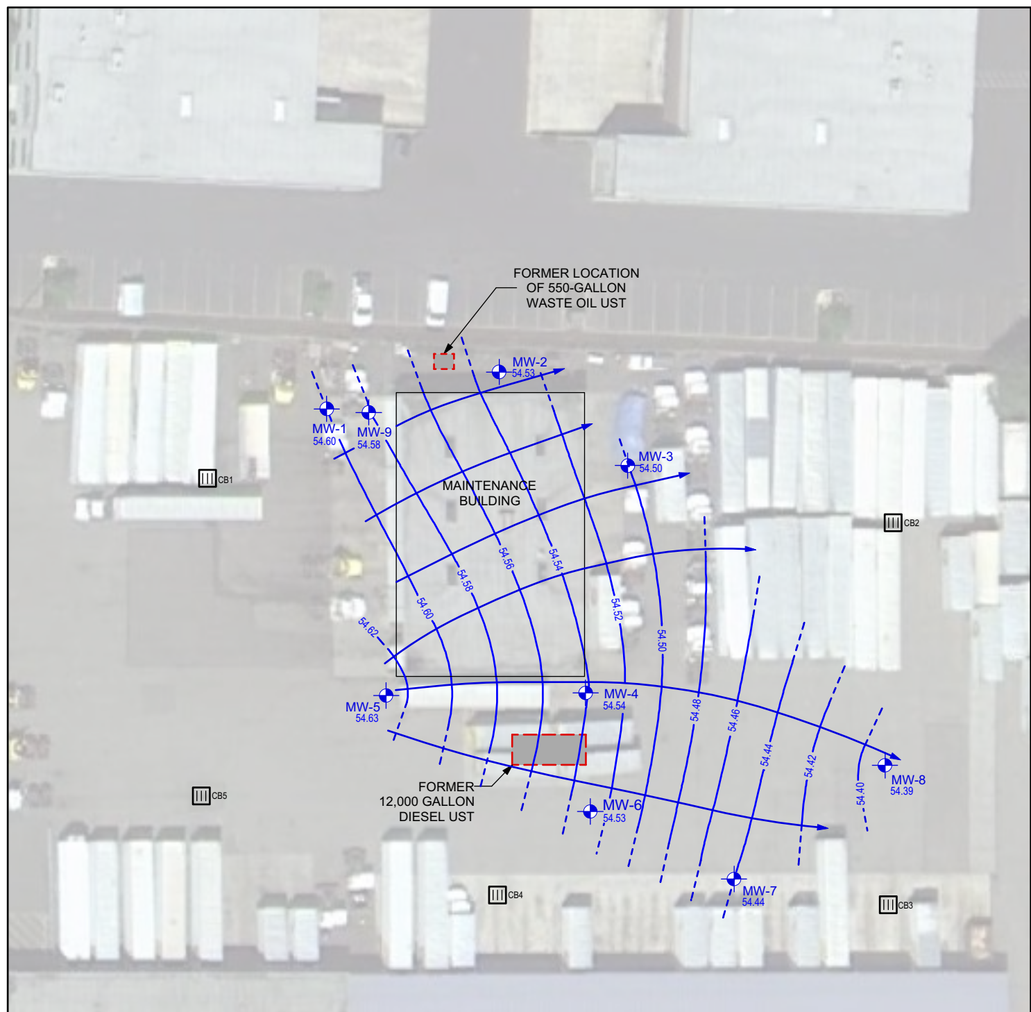
FIGURE 3 SEPTEMBER 5, 2017 GROUNDWATER ELEVATION CONTOURS AND FLOW DIRECTION
