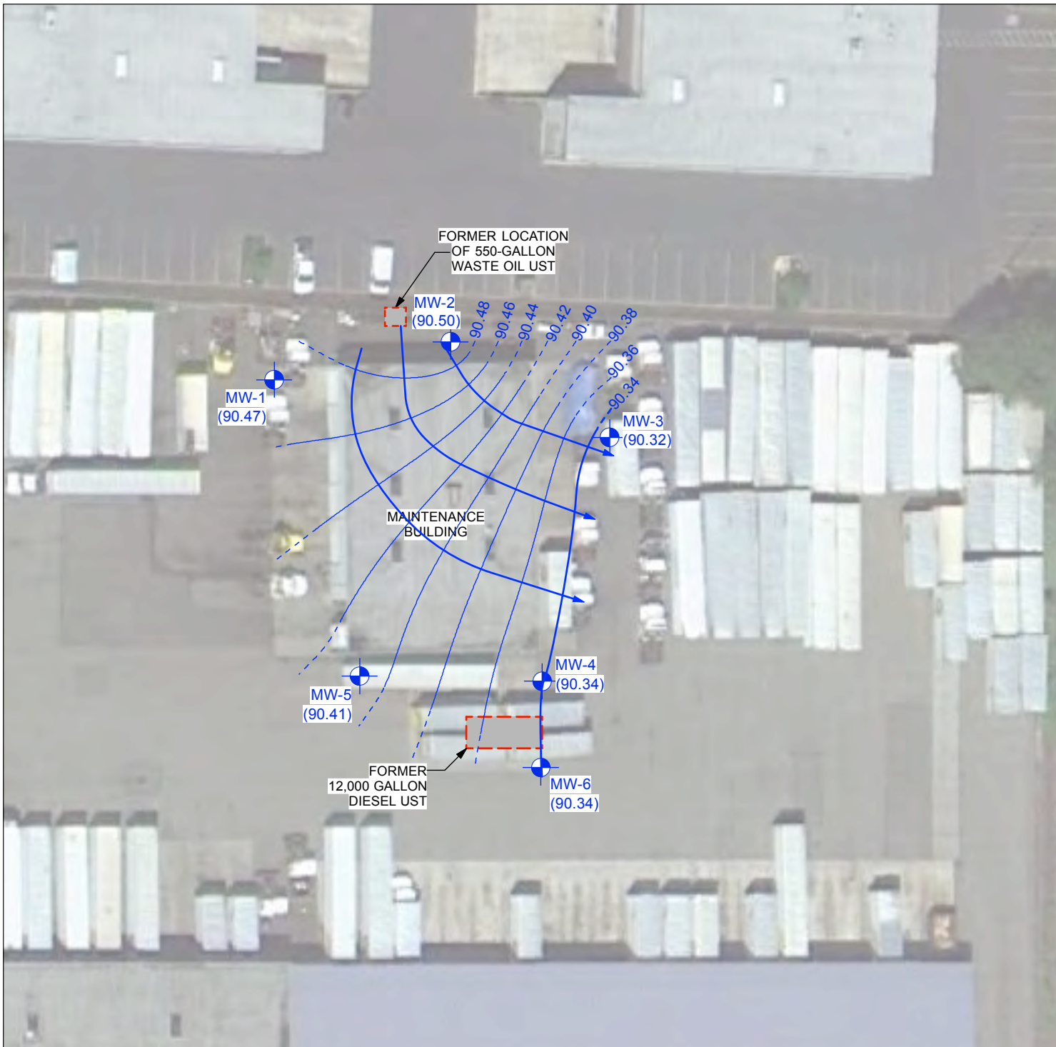
FIGURE 3 MARCH 31, 2015 GROUNDWATER ELEVATIONS AND FLOW DIRECTIONS
