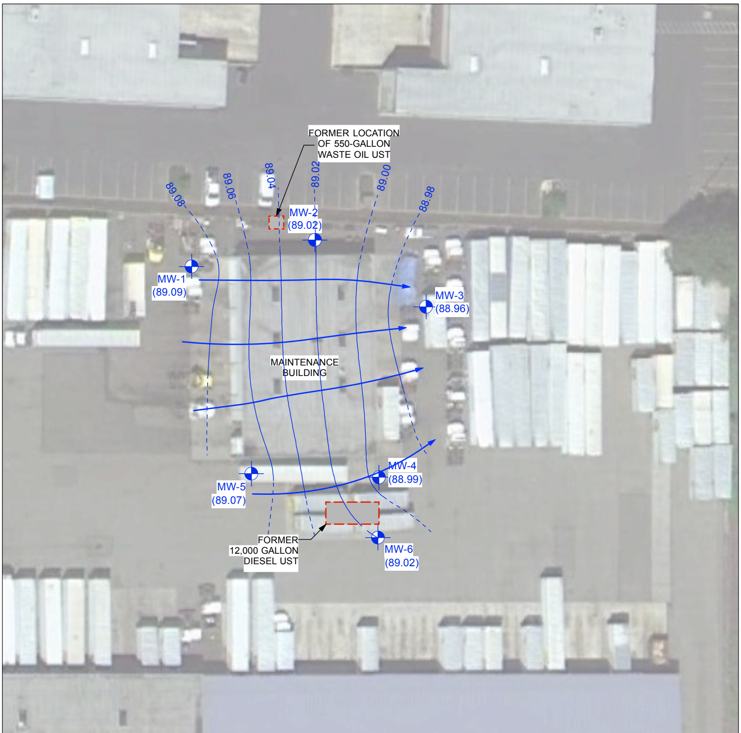
FIGURE 3 SEPTEMBER 28, 2015 GROUNDWATER ELEVATIONS AND FLOW DIRECTIONS
