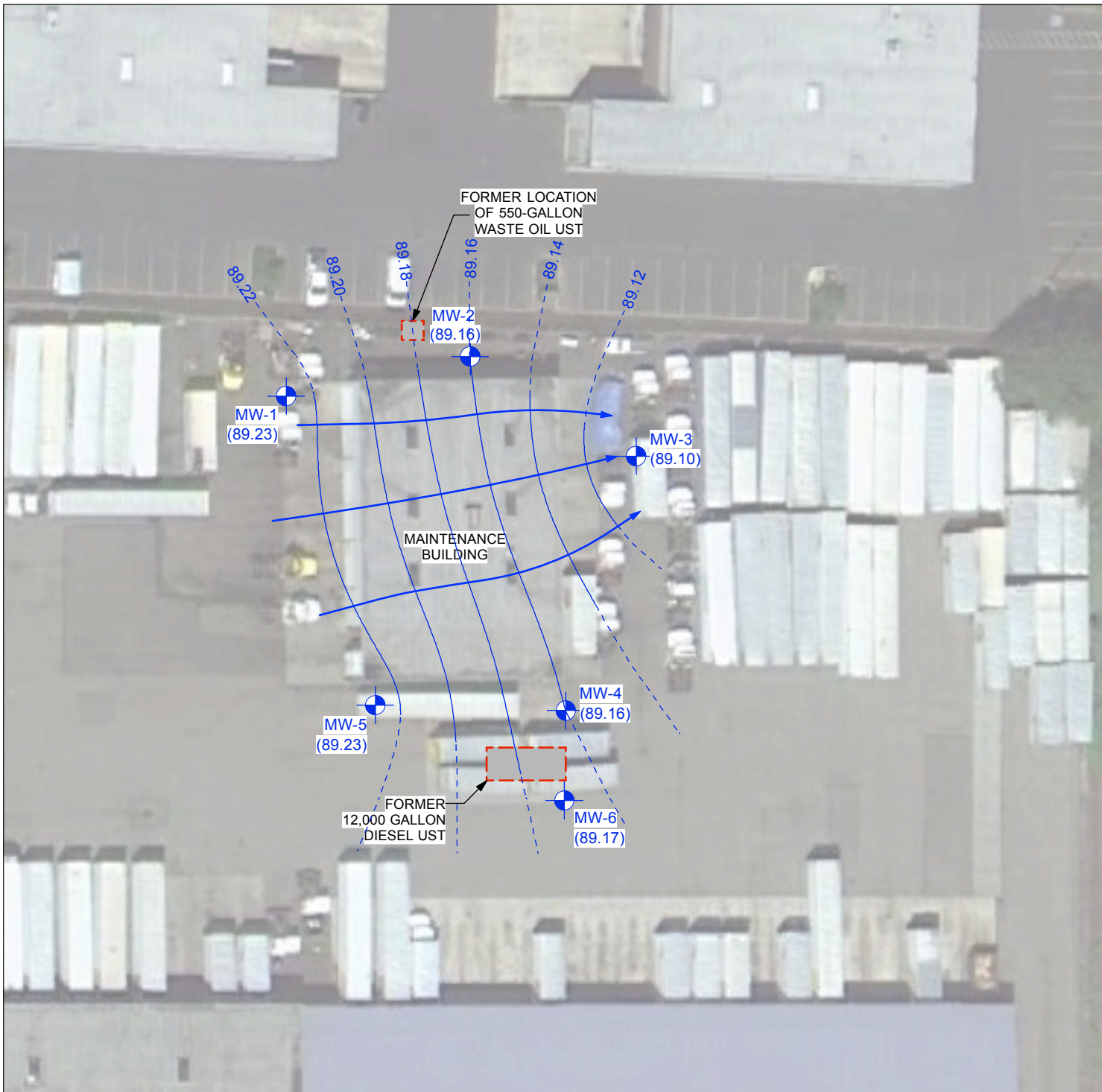
FIGURE 3 JUNE 29, 2015 GROUNDWATER ELEVATIONS AND FLOW DIRECTIONS
