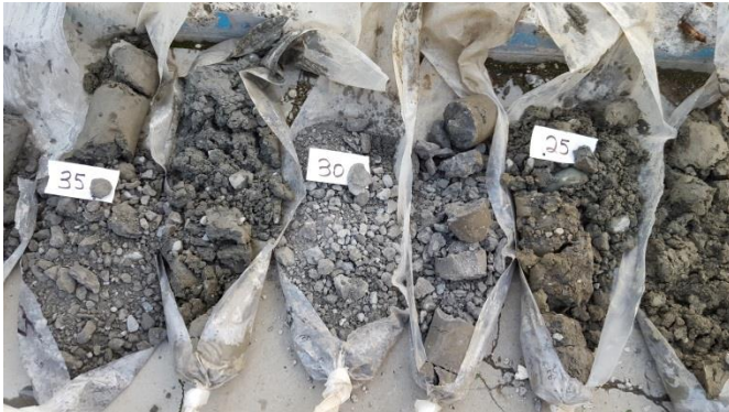
Photograph 1. Sonic core of injection well IW01 from approximately 0 to 15 feet bgs.
