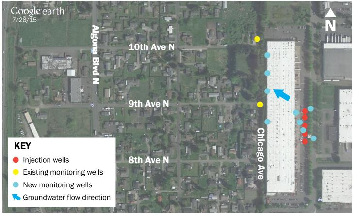
During the pilot study, Boeing tested a cleanup method called bioremediation. Groundwater was sampled downstream at new and existing monitoring wells (shown in blue and yellow). The study found that bioremediation decreases the contamination in the groundwater.
