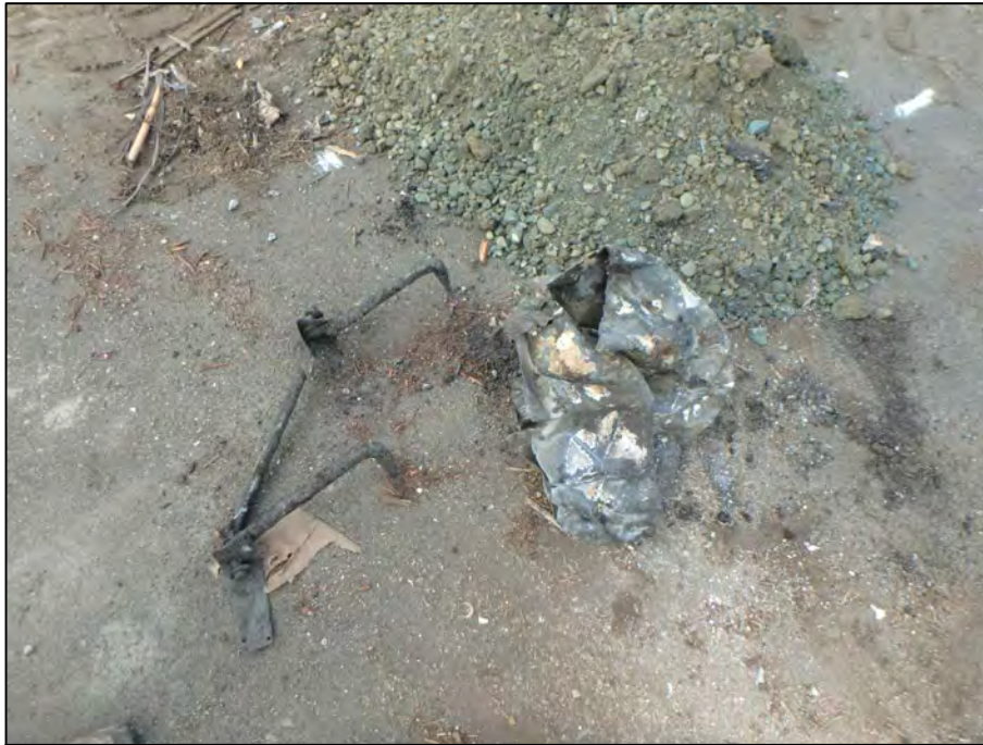
Photograph 23: Metal debris removed from TP1 and TP2, most likely the result of elevated metal detector readings during the geophysical survey.
