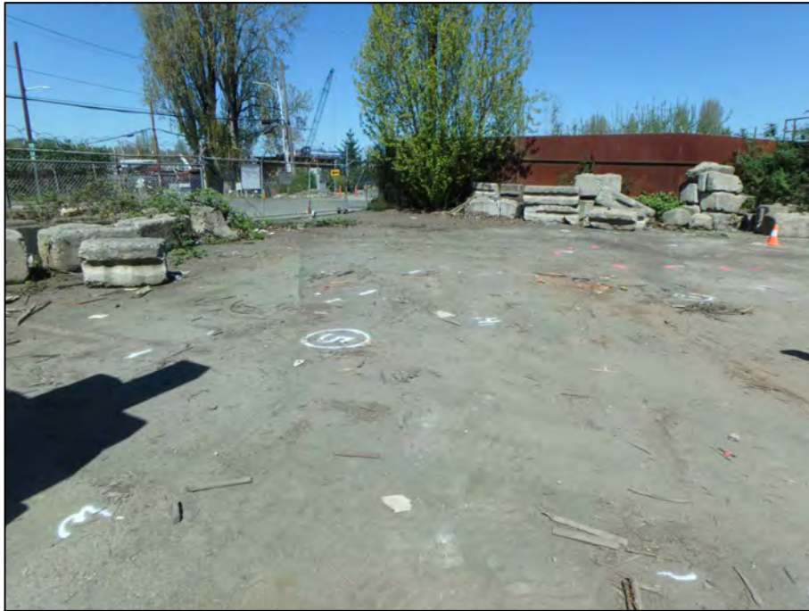
Photograph 3: View looking northwest at the northern portion of the Property and suspected location of USTs. The white markings depict suspected UST locations identified during a geophysical survey.
