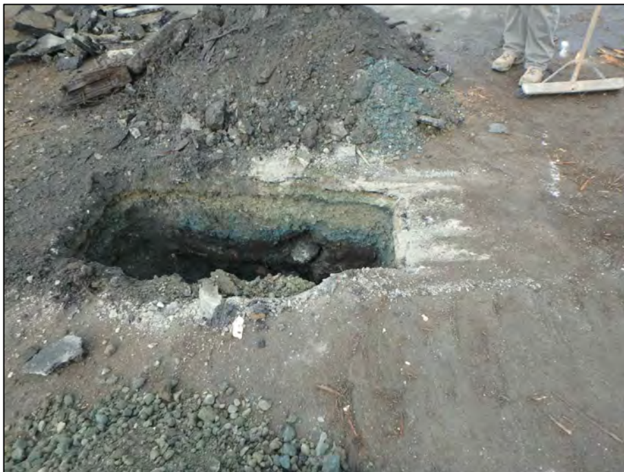
Photograph 22: Cross-section of TP1 showing the blueish-green layer beneath the pea gravel and asphalt. The mottled subsurface soils are also visible. Wood and metal fill was removed from TP1.
