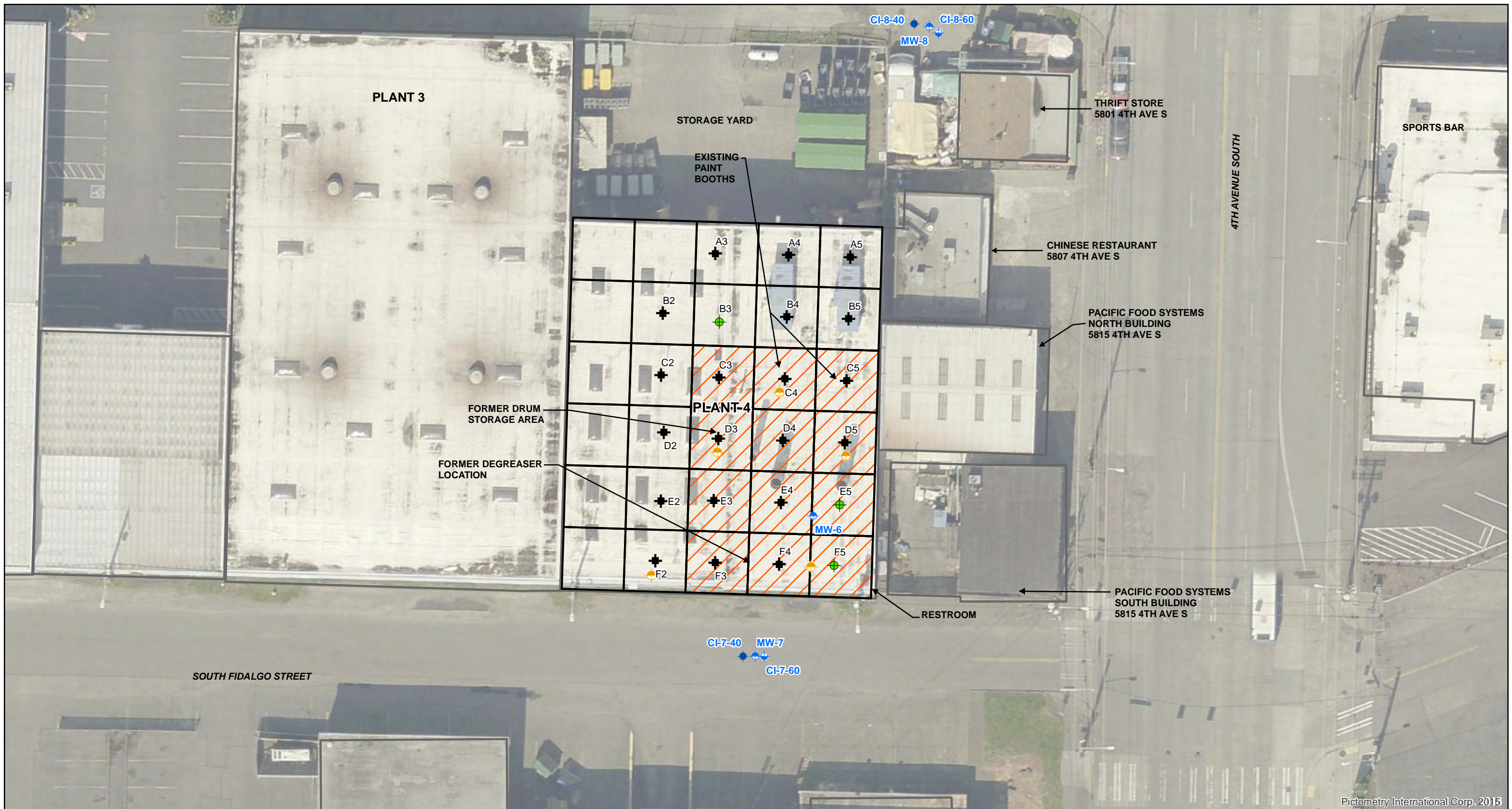
FIGURE 5 PLANT 4 ISCO INJECTION POINTS AND MONITORING WELLS WEST OF 4TH GROUP SITE CAPITAL INDUSTRIES, INC. 5815 4TH AVENUE SOUTH SEATTLE, WASHINGTON FARALLON PN: 457-008
