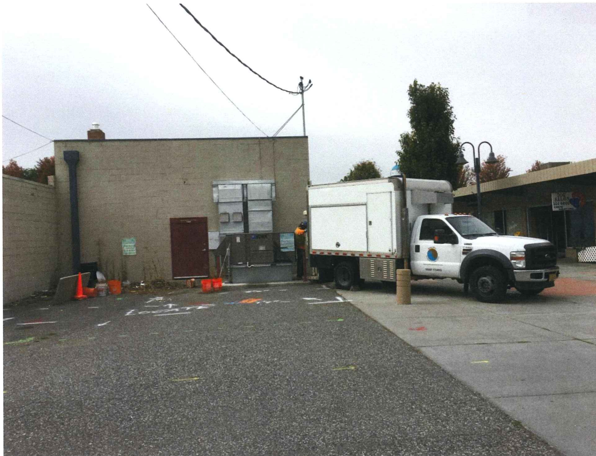
Photograph 4 – Geoprobe® subcontractor advancing BMEC-02 to a total depth of 8 feet below ground surface (facing west). Note single 16-gallon drum of investigation-derived waste near corner of building near orange safety cone.
