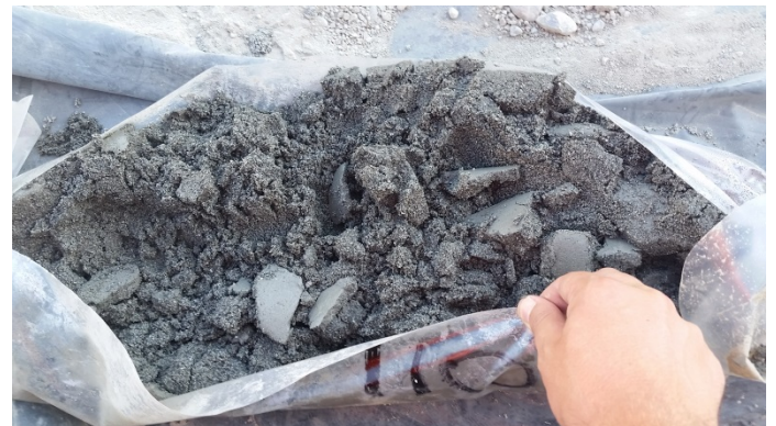
Photograph 4. Soil cuttings recovered from 110 feet below ground surface from MW-17.
