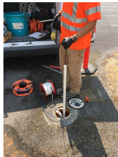
Photograph 6. Field setup during slug testing at monitoring well MW-11.
