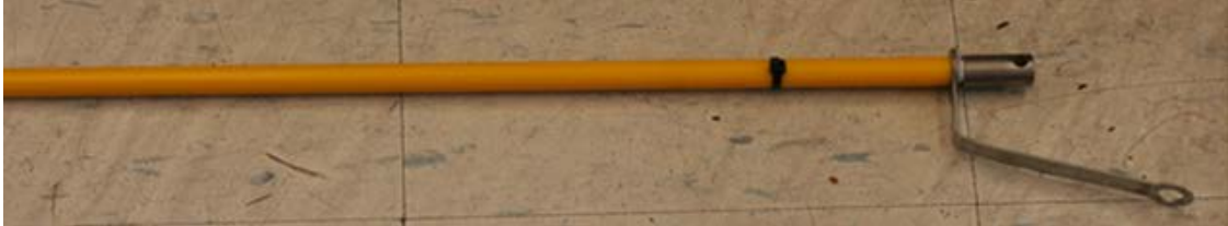
Figure 8. Zip-tie indicating location of "mud-line"
