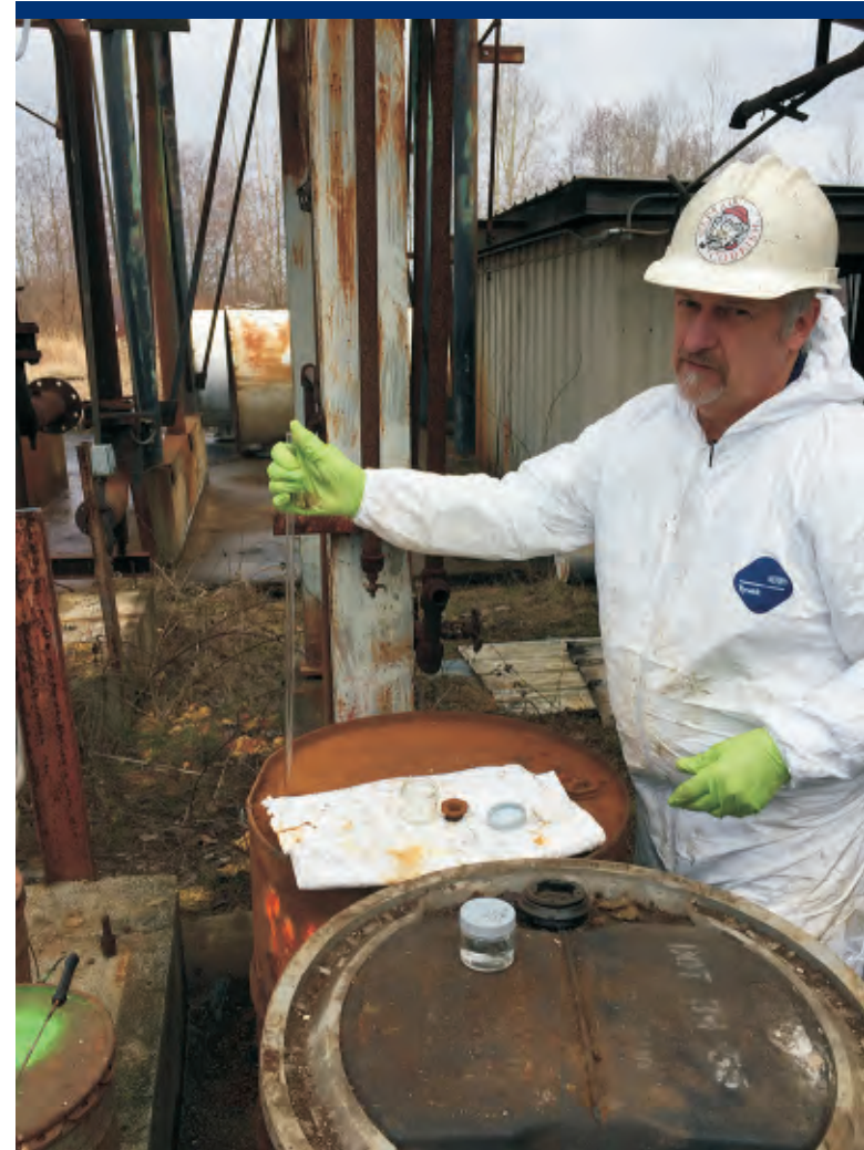
Photo 25 START collecting a sample from a drum of unknown contents from Warehouse B.
