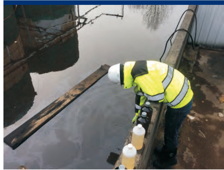
Photo 28 Location of surface water sample SCC01 collected from Secondary Containment C.
