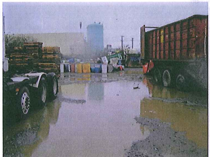
#16. DESCRIPTION: The drums stored here are damaged and are waiting for repair or to be scrapped. Stormwater flows from the drums towards the photographer. The permit requires these drums to be stored under cover or be provided with a tight fitting lid.
