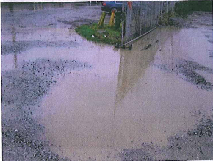
#1. DESCRIPTION: Seattle Iron & Metals Truck Parking (Annex) has coverage under the Industrial Stormwater General Permit. The site is a little over 3 acres and is divided into 3 sections. This gate is located on S. Myrtle Street. The turbid stormwater has a visible sheen on it.
