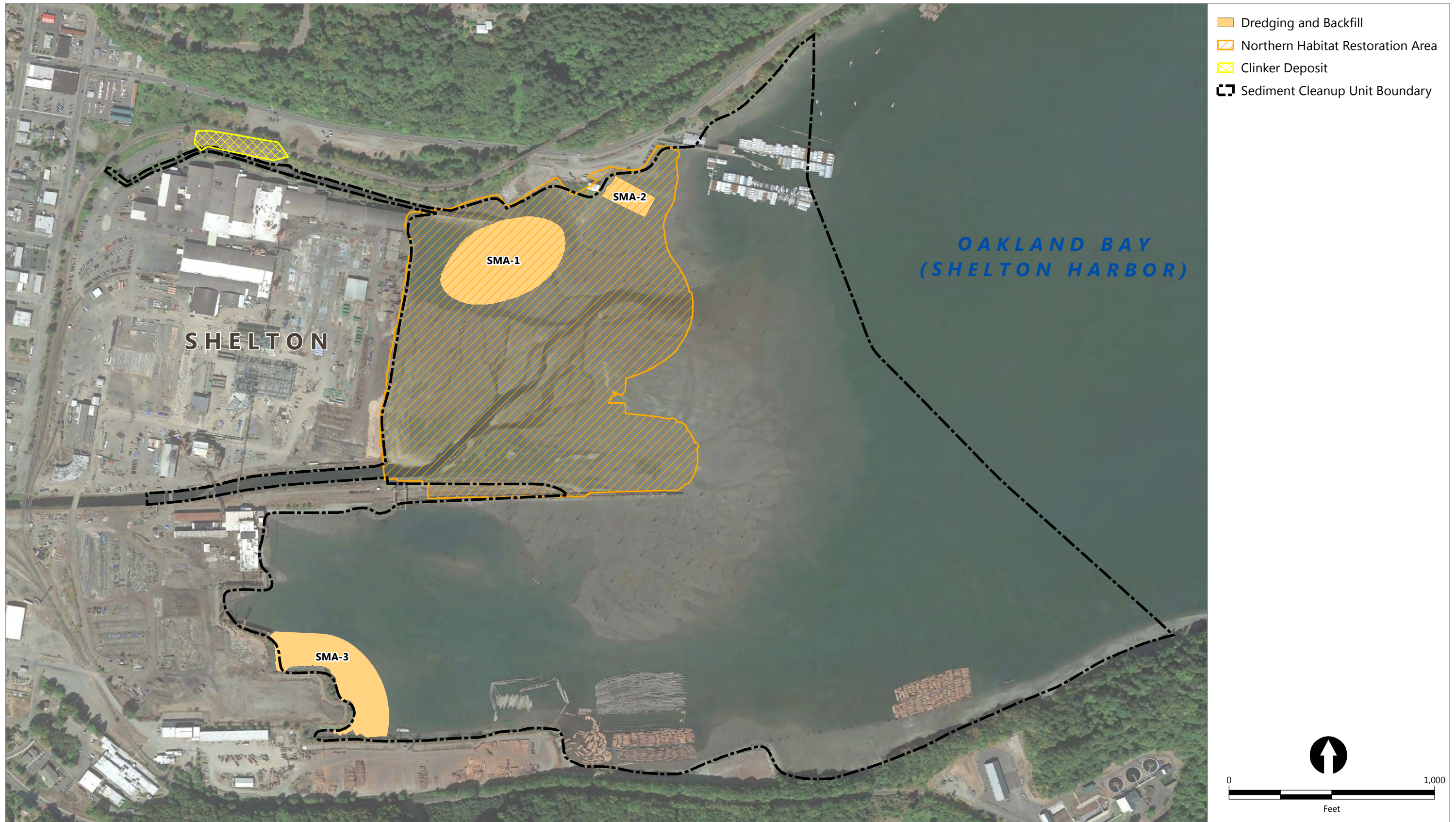
Figure 4-2 Interim Action Alternative 1 – Removal Shelton Harbor Interim Action Plan Oakland Bay and Shelton Harbor Sediments Cleanup Site
