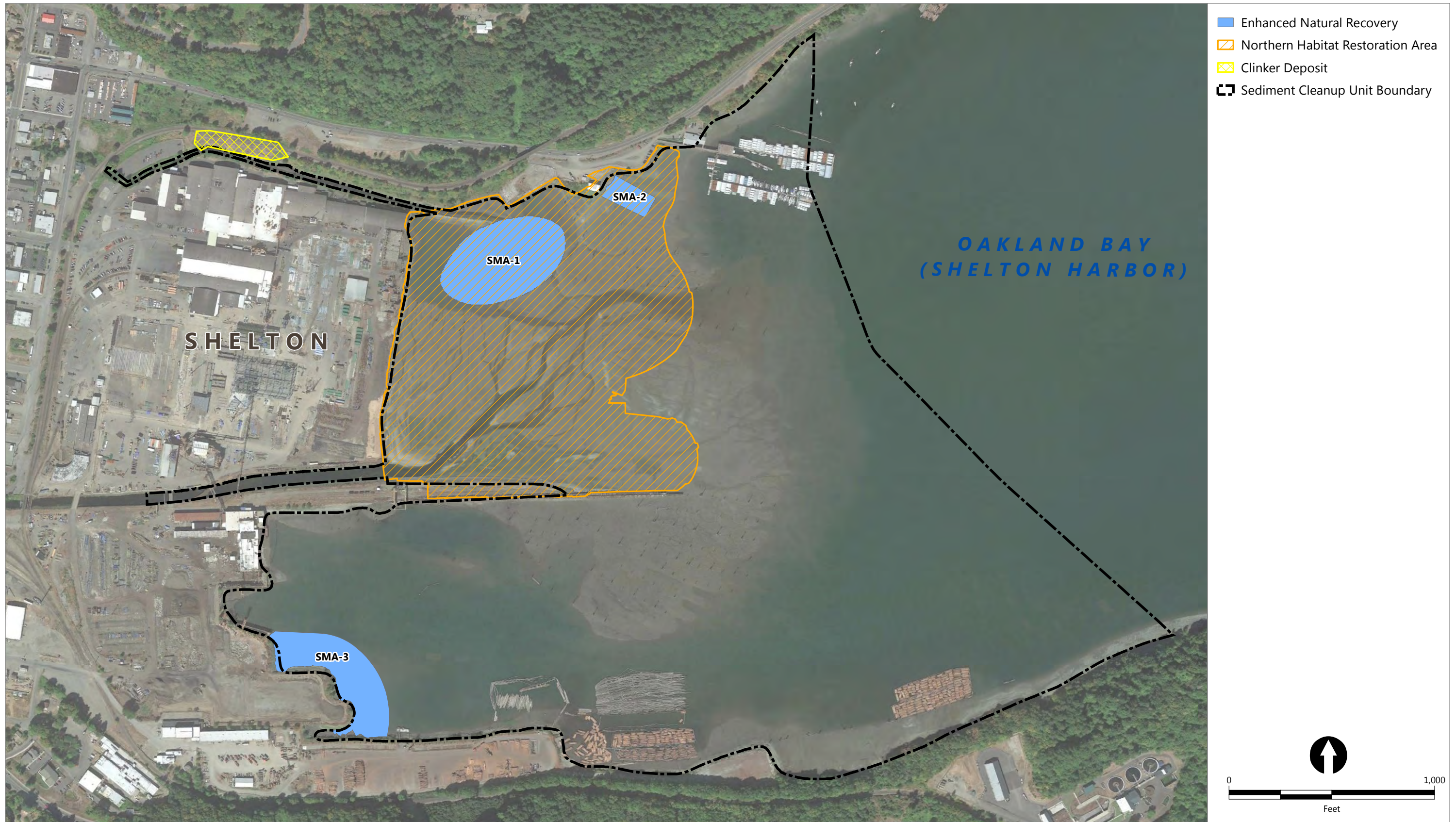
Figure 4-4 Interim Action Alternative 3 – Enhanced Natural Recovery Shelton Harbor Interim Action Plan Oakland Bay and Shelton Harbor Sediments Cleanup Site
