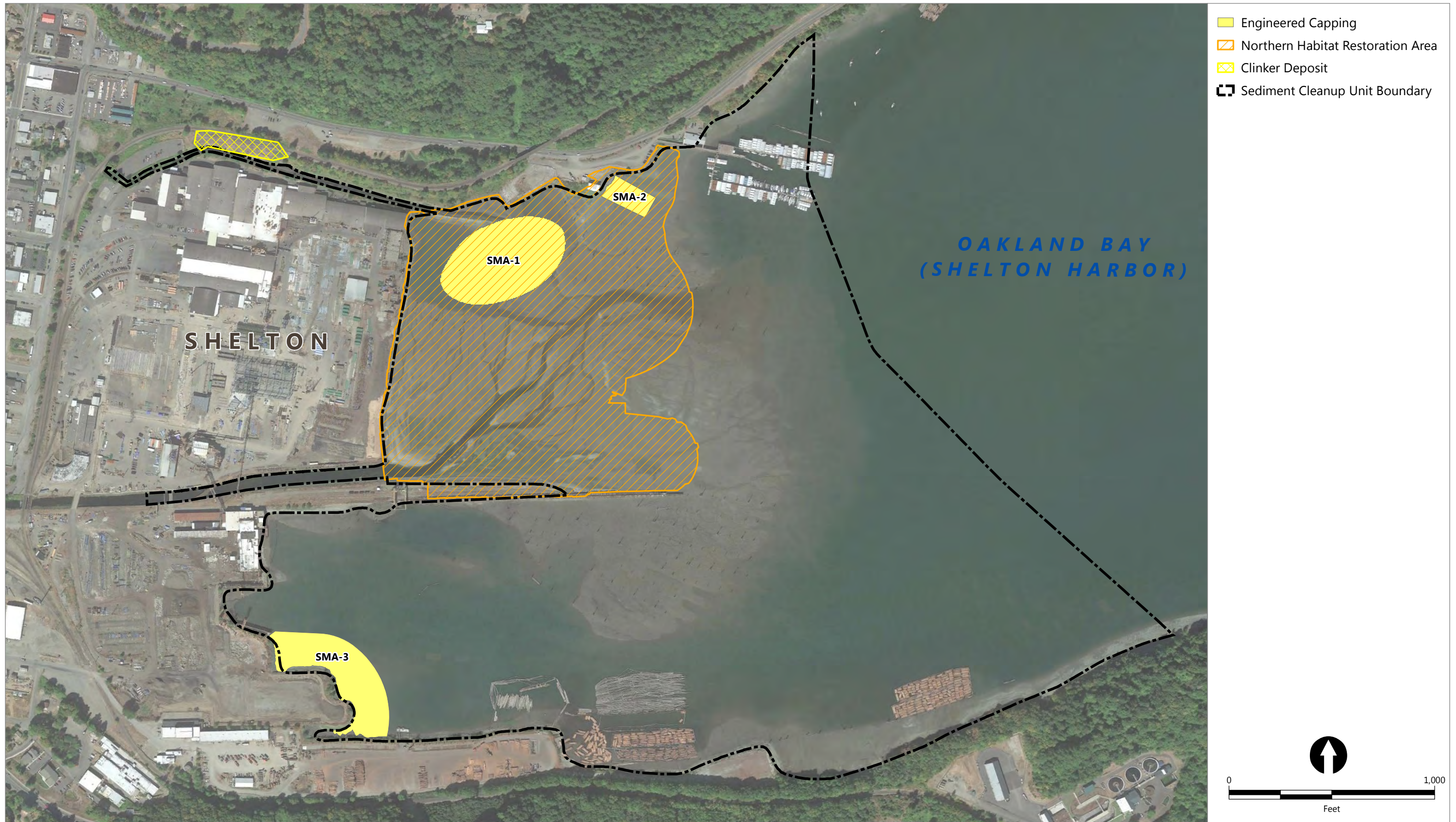
Figure 4-3 Interim Action Alternative 2 – Engineered Capping Shelton Harbor Interim Action Plan Oakland Bay and Shelton Harbor Sediments Cleanup Site
