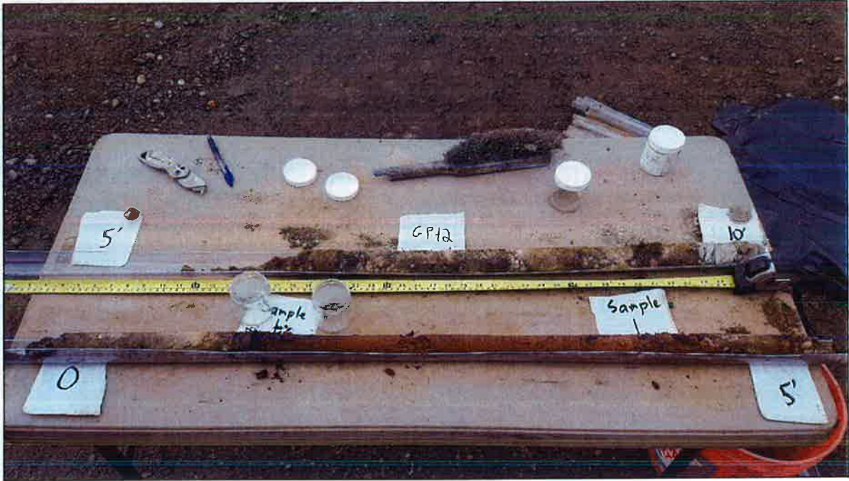
Photo 12. Continuous sample from borehole GP-12. Lab samples taken at 1.4 feet and 4.0 feet.
