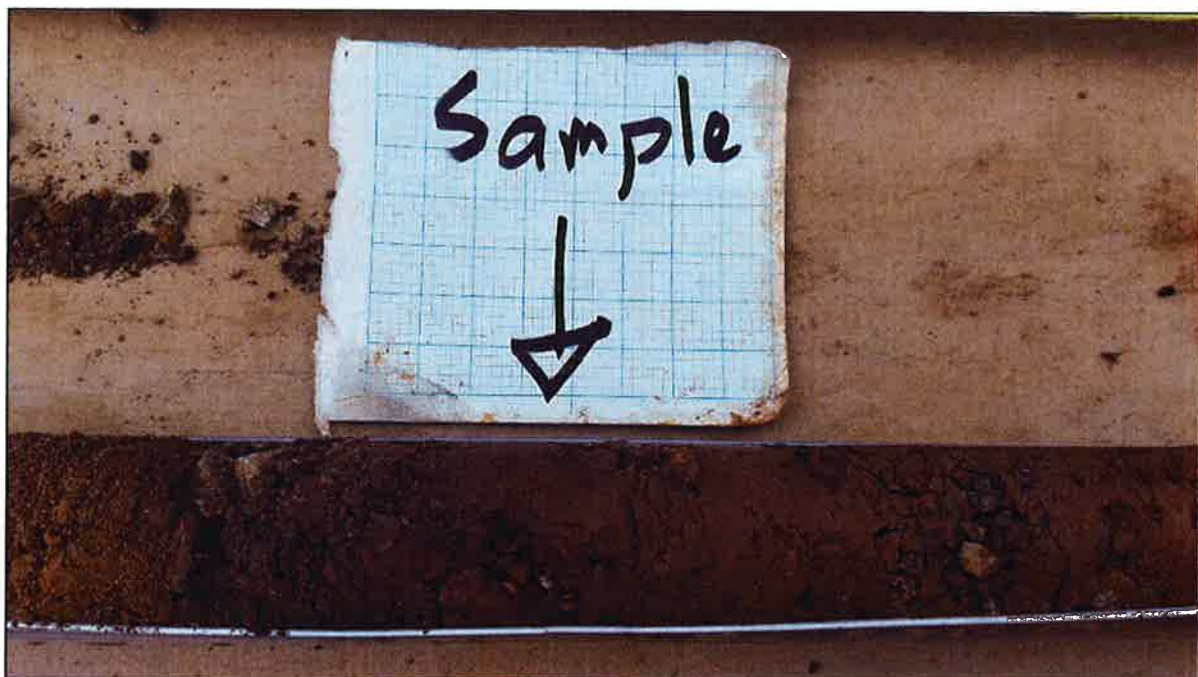
Photo 14. Lab samples were gathered directly to jars from 4" to 6" span within sample sleeves.
