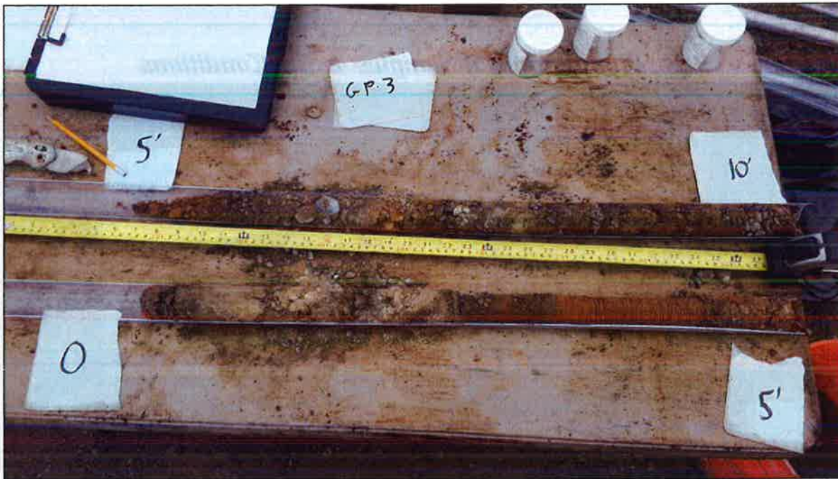
Photo 3. Continuous sample from borehole GP-3. Lab samples taken at 2.8 feet and 5.0 feet.
