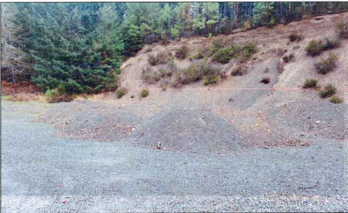
Photo 20. Close view of stockpile. Primarily crushed rock, sand and gravel in small piles.
