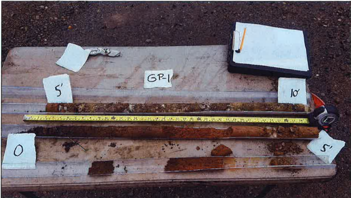
Photo 1. Continuous sample from borehole GP-1. Lab samples taken at 0.8 feet and 2.3 feet.
