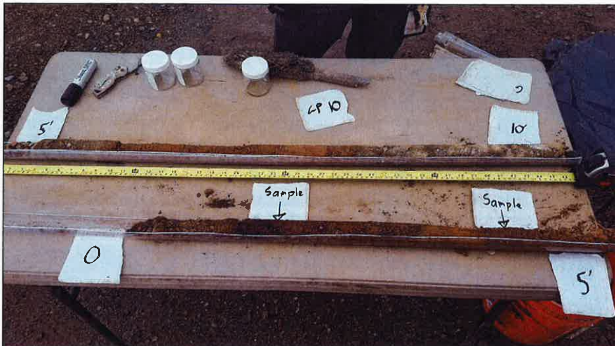
Photo 10. Continuous sample from borehole GP-10. Lab samples taken at 1.3 feet and 4.0 feet.
