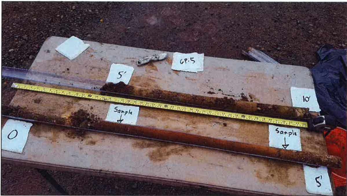
Photo 5. Continuous sample from borehole GP-5. Lab samples taken at 1.8 feet and 4.0 feet.
