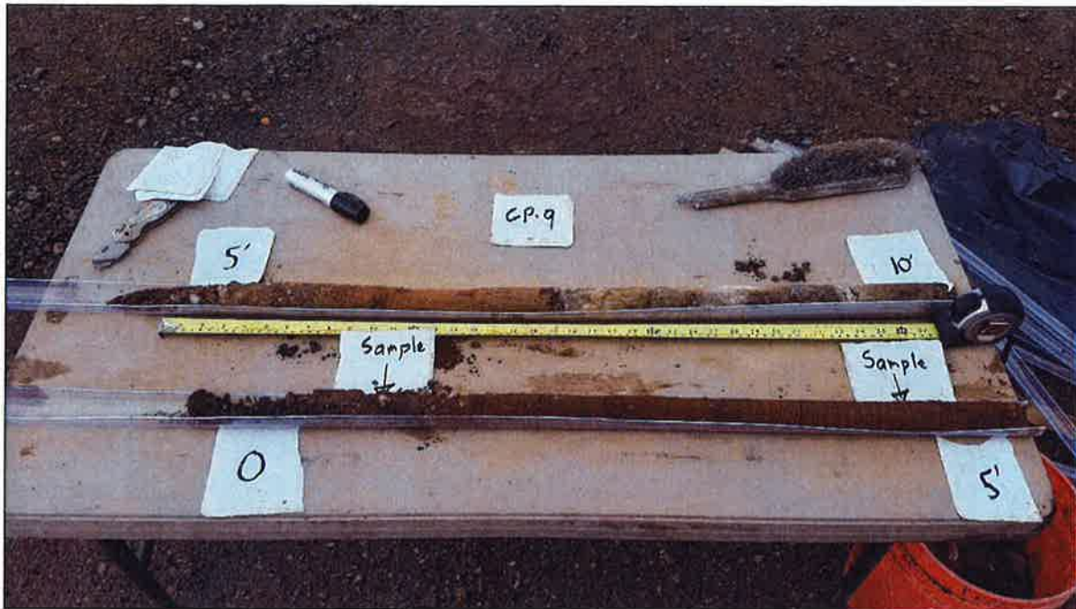
Photo 9. Continuous sample from borehole GP-9. Lab samples taken at 0.5 feet and 4.5 feet.
