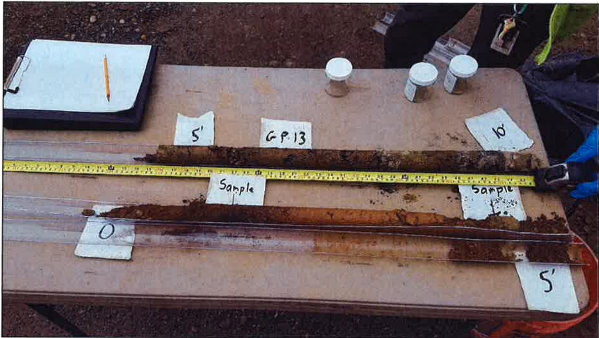
Photo 13. Continuous sample from borehole GP-13. Lab samples taken at 1.3 feet and 4.5 feet.
