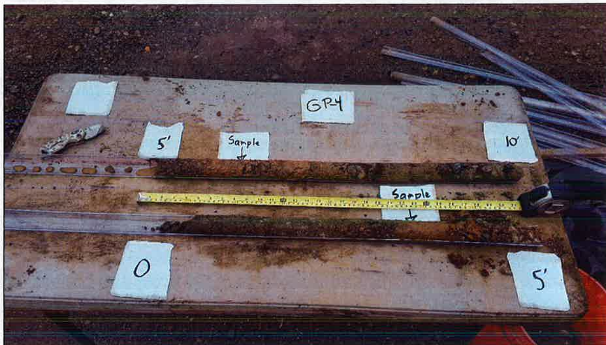
Photo 4. Continuous sample from borehole GP-4. Lab samples taken at 3.5 feet and 6.5 feet.
