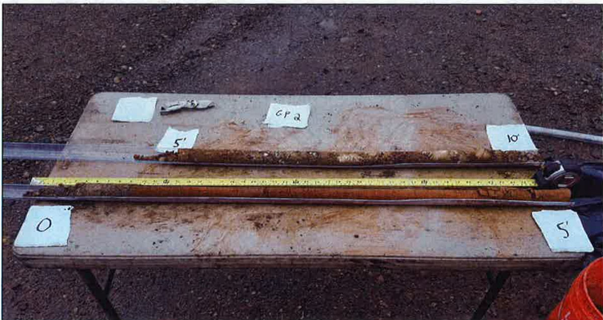
Photo 2. Continuous sample from borehole GP-2. Lab samples taken at 1.5 feet and 5.5 feet.
