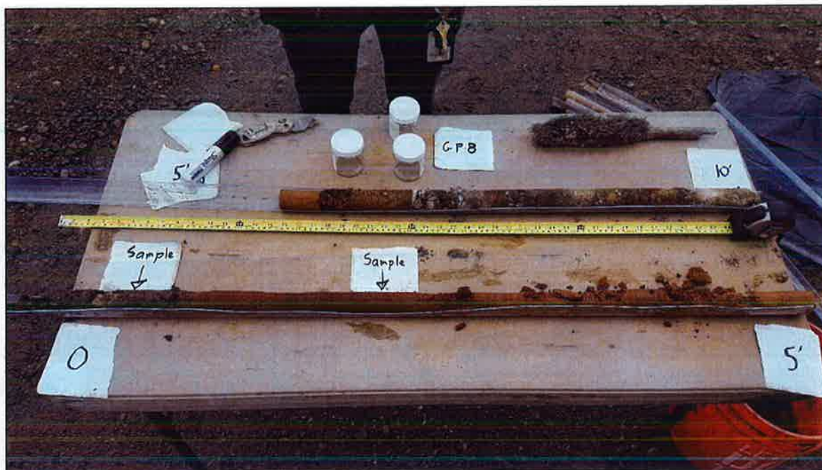
Photo 8. Continuous sample from borehole GP-8. Lab samples taken at 0.6 feet and 2.3 feet.
