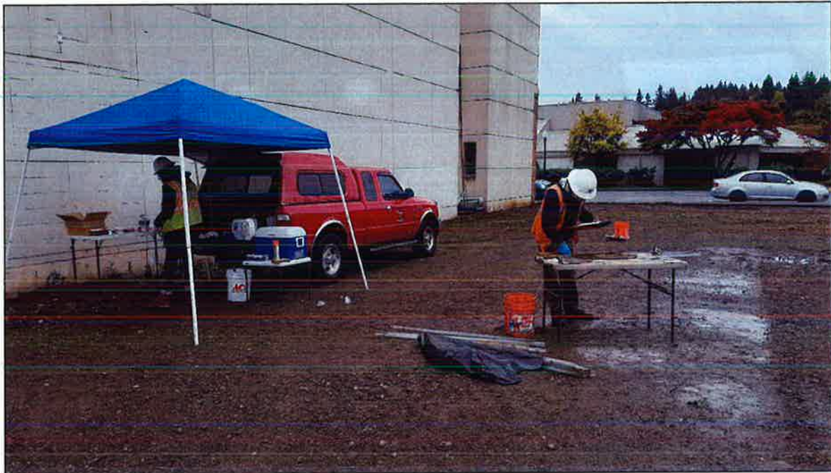
Photo 15. Sample sleeves were visually examined and soils logged prior to sample collection.
