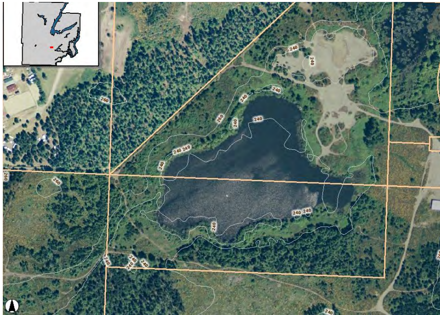
Figure 1. USGS Topography of Goose Lake area (20-ft contours) indicating a swale base elevation of 240 ft, and terrace surface elevation of 260 ft ( \pm 10 ft).
