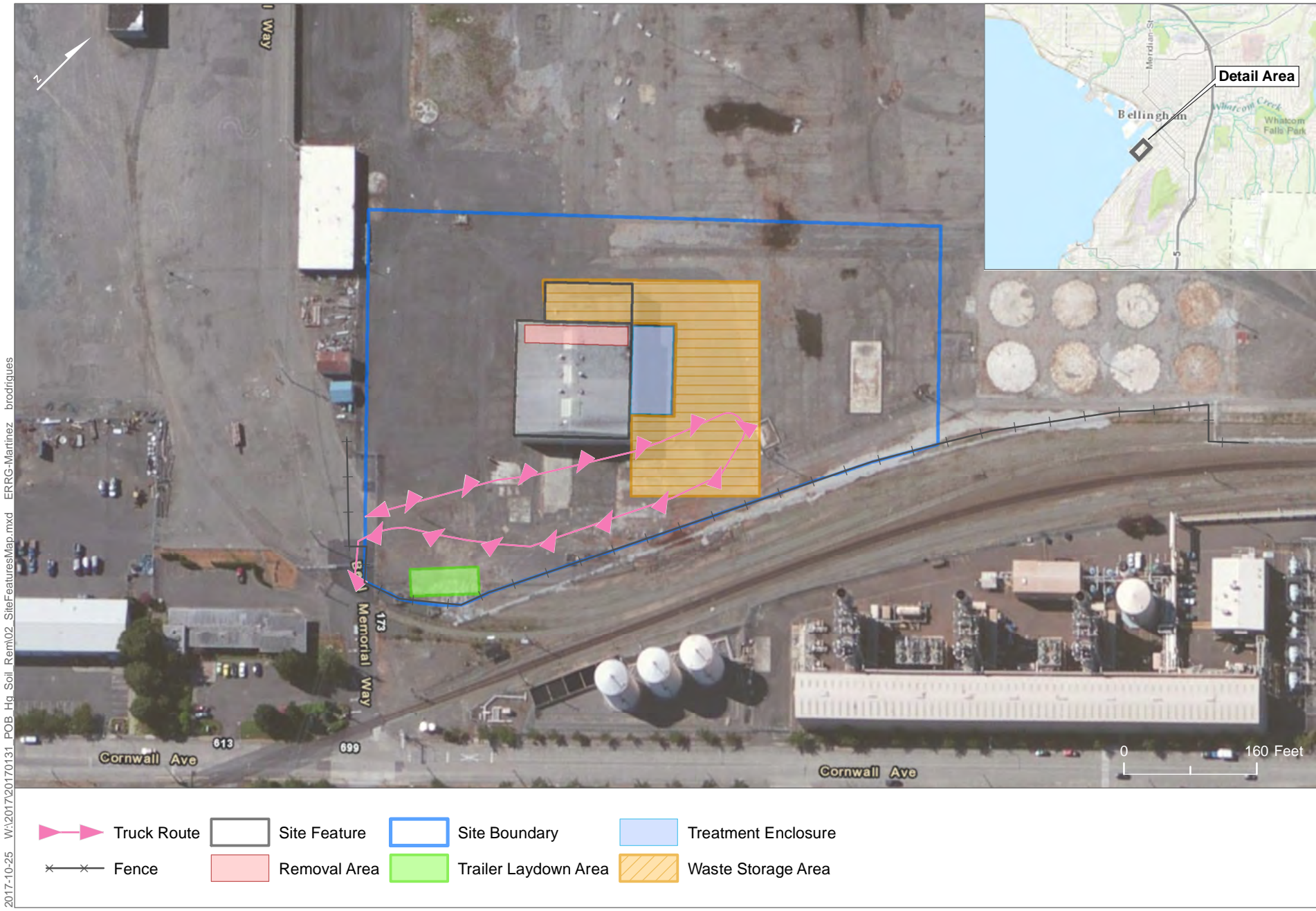
Figure 2. Site Features Map Port of Bellingham Mercury Soil Treatment and Disposal - Bellingham, Washington
