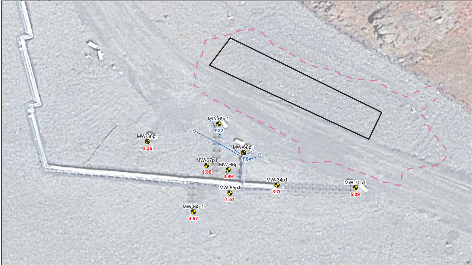
Figure 4 Thickness of P1 Vadose Zone on 6/12/17 (Pre-test)
