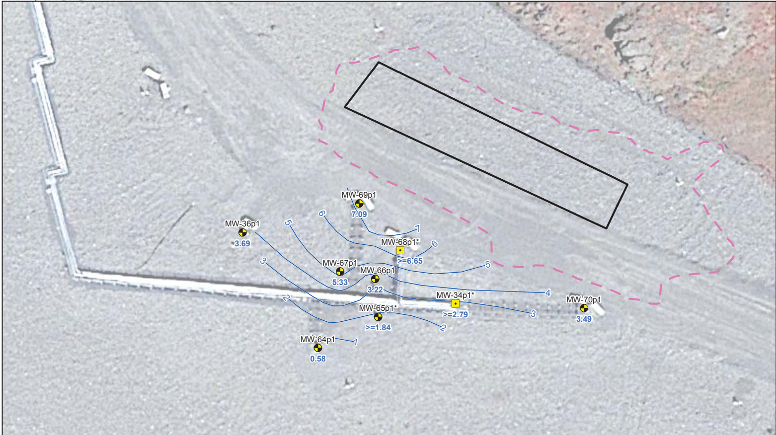
Figure 13 Thickness of P1 Vadose Zone on 9/26/17 (12.5 inches-Hg, Two Wells)
