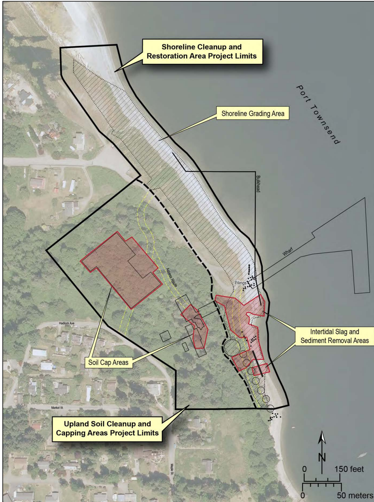
Figure 2. Irondale Iron and Steel Plant work areas.
