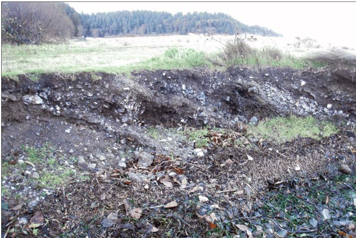
Figure 17. Cross-bedded slag deposits exposed in an erosion profile on the south side of the slag fill area.
