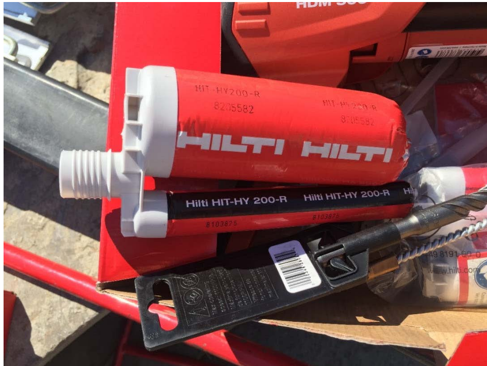
Photograph 7: Hilti adhesive for installation of new anchor bolts for lifting.
