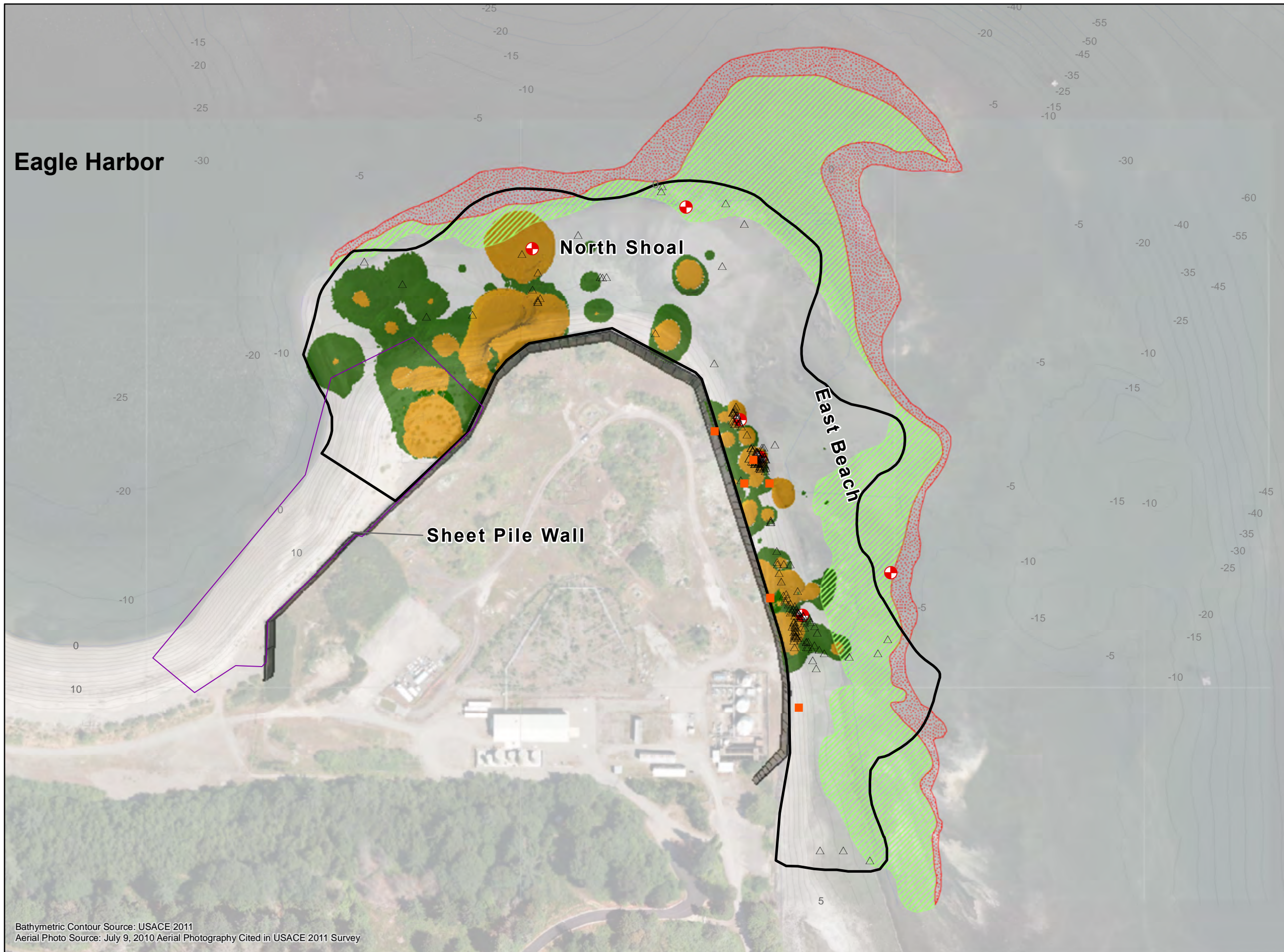
Figure 3-5 NAPL Distribution in Subsurface Sediments Wyckoff OU-1 Focused Feasibility Study
