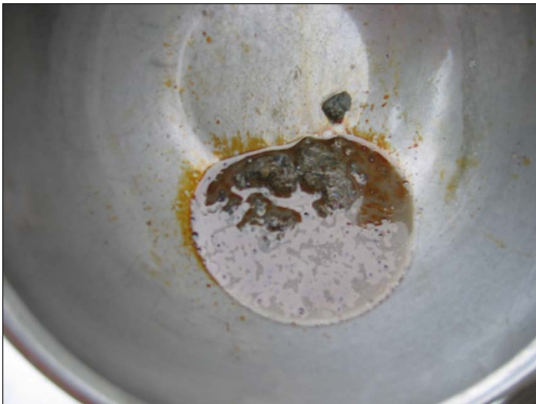
Field Photograph 2. NAPL encountered in Boring SB-2 at the groundwater table.
