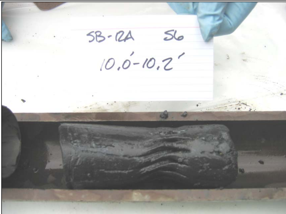
Field Photograph 1. Tar-like material observed in Boring SB-12A. Petrophysical sample.
