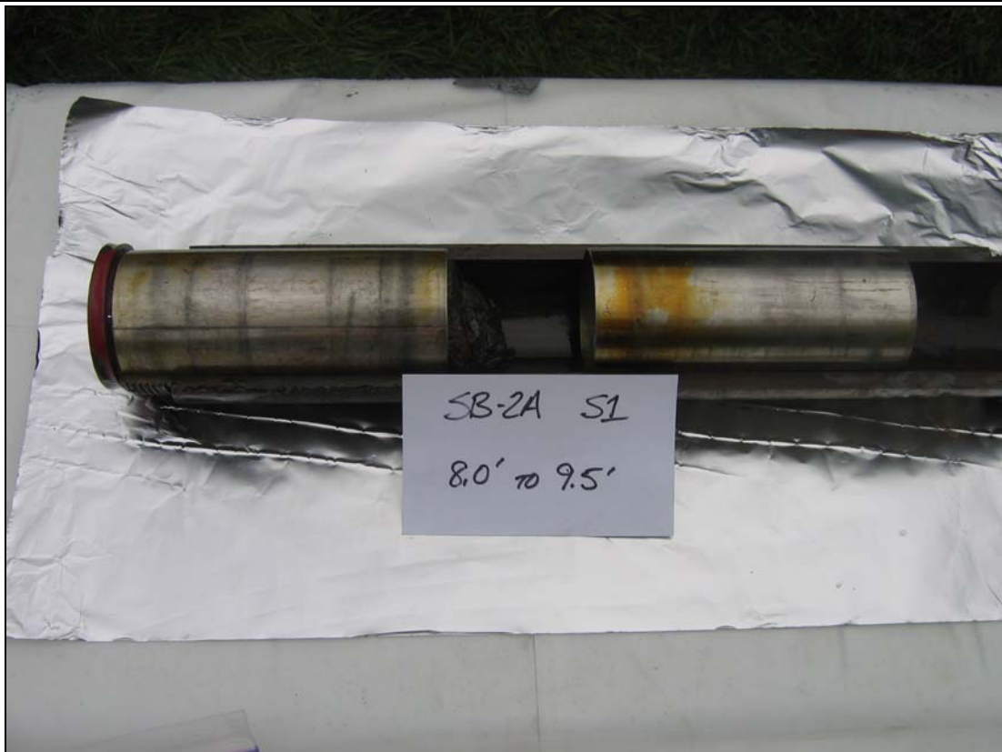
Field Photograph 3. NAPL encountered in SB-2A at a depth of 8.0 to 9.5 feet below ground surface.
