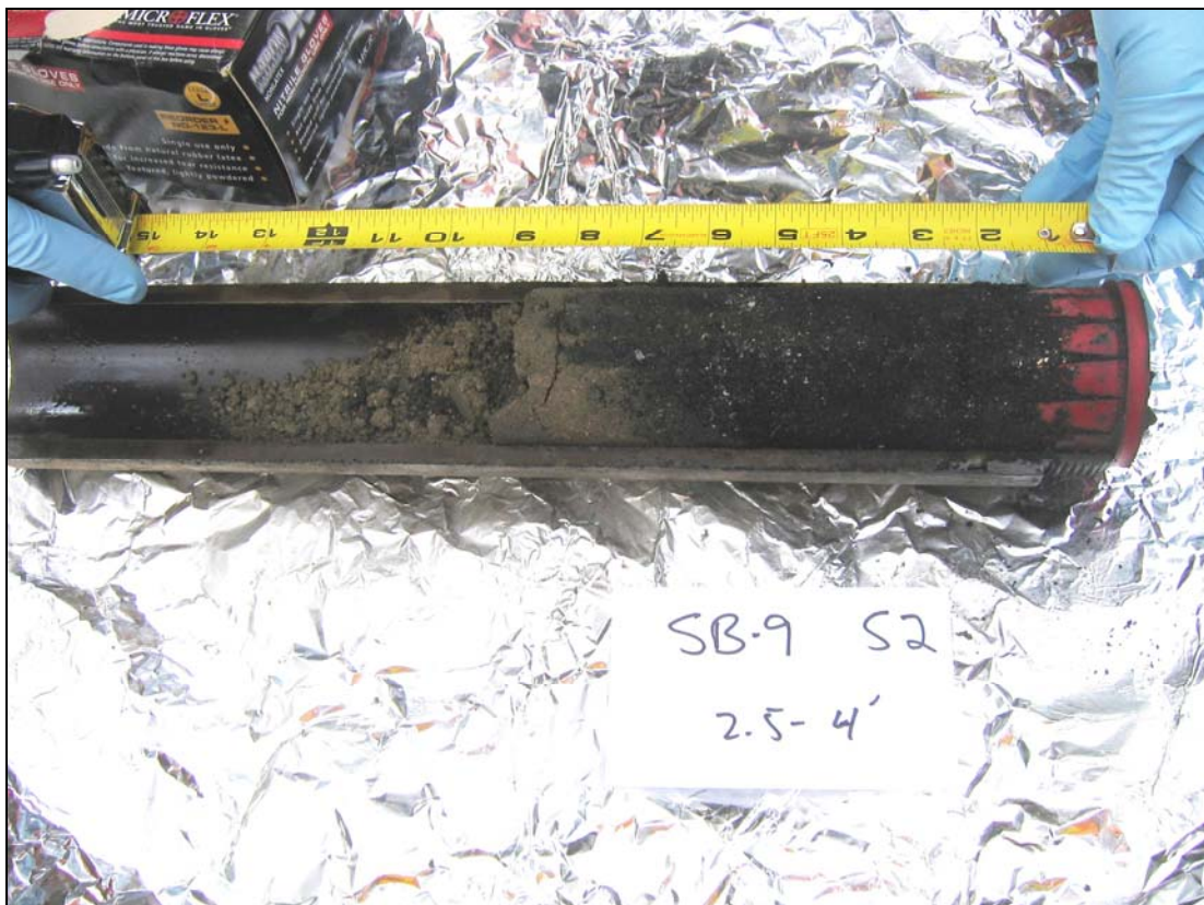
Field Photograph 4. Black staining of the Gas Works Fill Unit observed in Boring SB-9.
