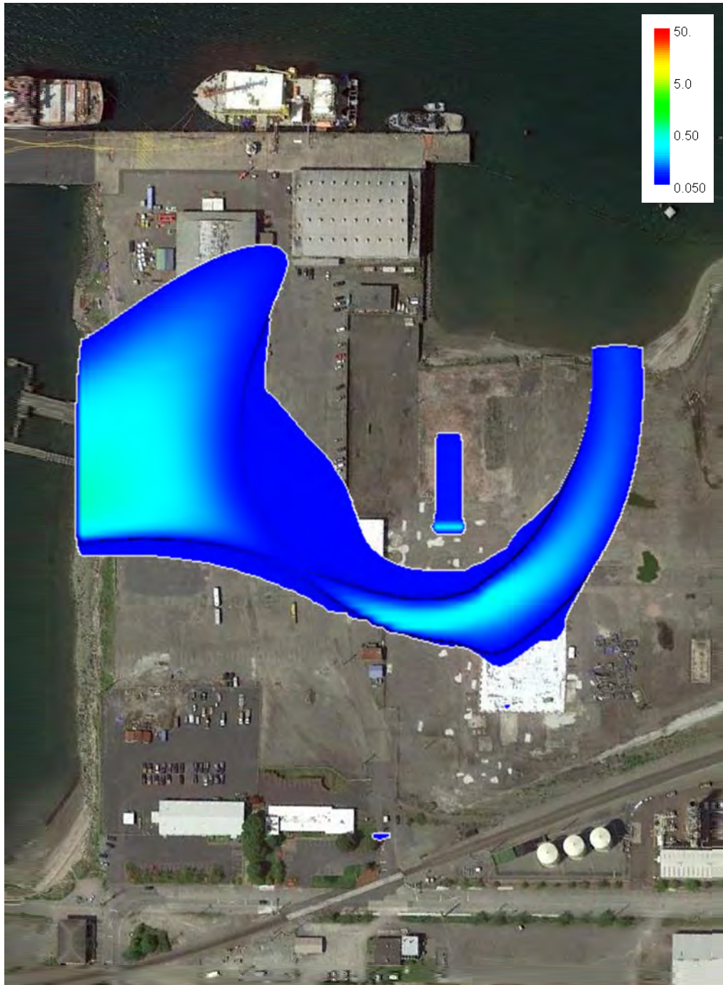
Figure 4 Simulated Hg concentrations in groundwater 20 years after active remediation for Alternative 5
