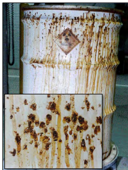
Figure 2.1. Pinhole corrosion of drums containing chlorinated solvents in CH-TRU waste at Idaho National Lab (Zeck, 1998). Inset is close up photo of pinhole corrosion.
