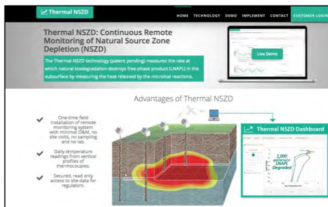
Figure 3.2. Thermal NSZD technology to measure biodegradation in subsurface by measuring heat (ThermalNSZD.com).
