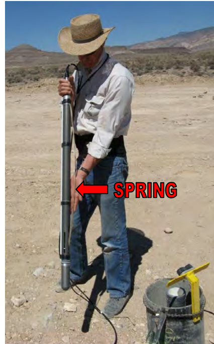
Photo 2: BHG3 Downhole Geophone
