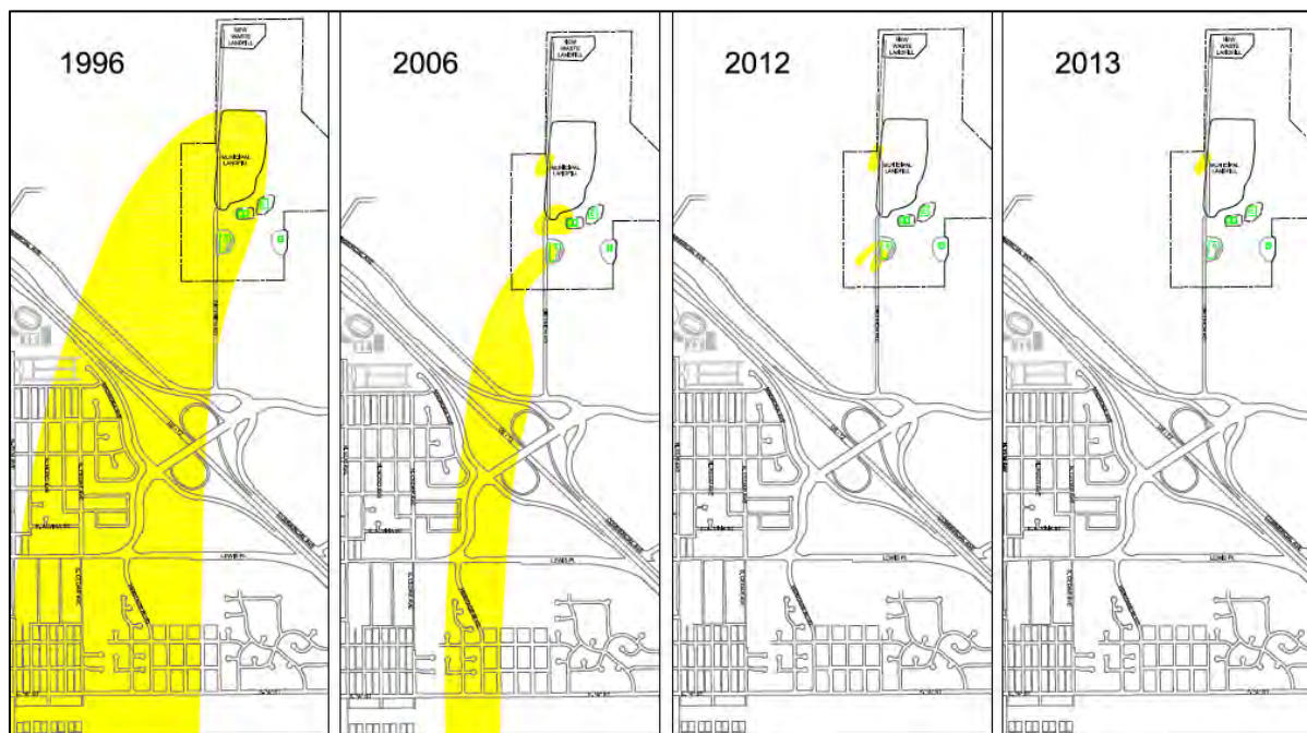
Figure 1.1. Reduction in volatile organic compound (VOC) concentrations in the off-property groundwater plume 1996-2013. Remediation measures included startup of the SVE system in 1997; installation of an engineered cap in 2002; and startup of an enhanced SVE system in 2012.
