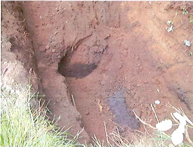
Photograph 3. Gray petroleum staining evident in soil directly below and surrounding UST (June 21, 2007).
