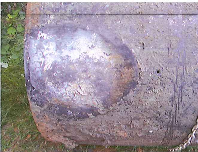
Photograph 5. Holes visible on bottom and west end of UST (June 21, 2007).
