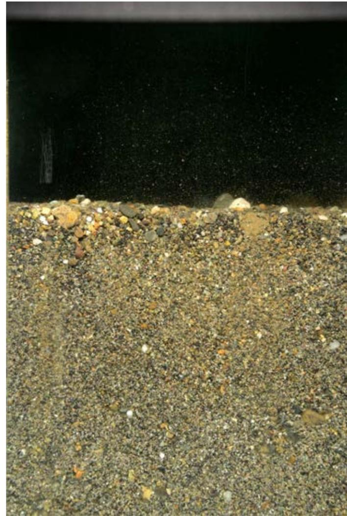
Figure 3-10. Representative SPI images from Stations LDW-Y0-SC-ENR+AC-2-A-SPI-R3 (left) and LDW-Y0-SC-ENR+AC-3-B-SPI-R1 (right) showing typical ENR+AC material from the scour subplot. In both images, ENR+AC material extends beyond the depth of camera prism penetration. Small, fine sand-sized, black, low reflectance particles are interspersed throughout the sediment column and its extent into the sediment column persists beyond the depth of prism penetration. SPI images are 14.42 cm in width.
