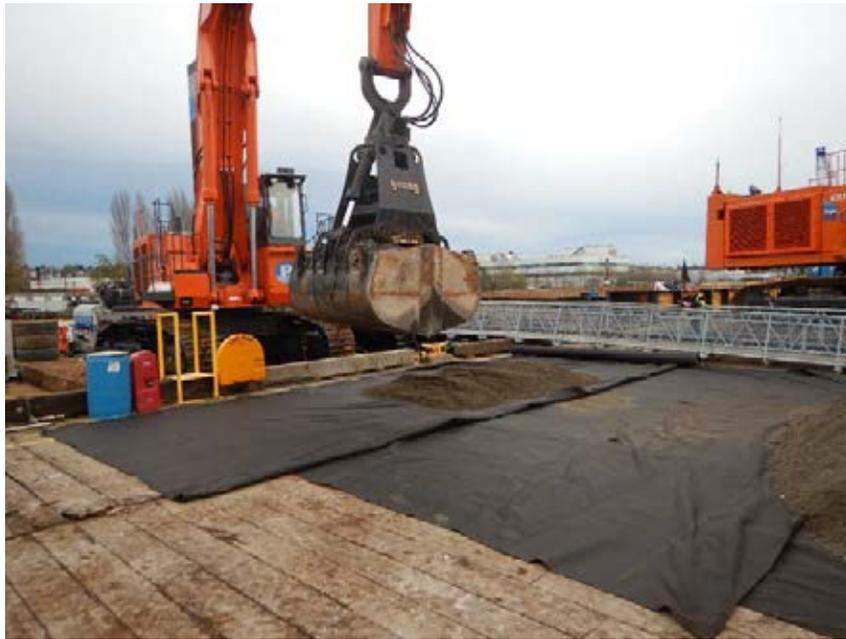
Photo 9 Bucket testing on dock with dry sand ENR.
