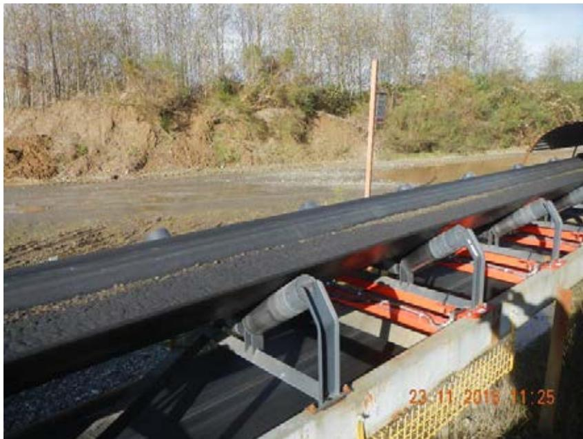
Photo 4 Black AC on top of brown ENR material moving down conveyor. Both materials are blended as they pass through several transition points prior to arriving at barge-loading dock.
