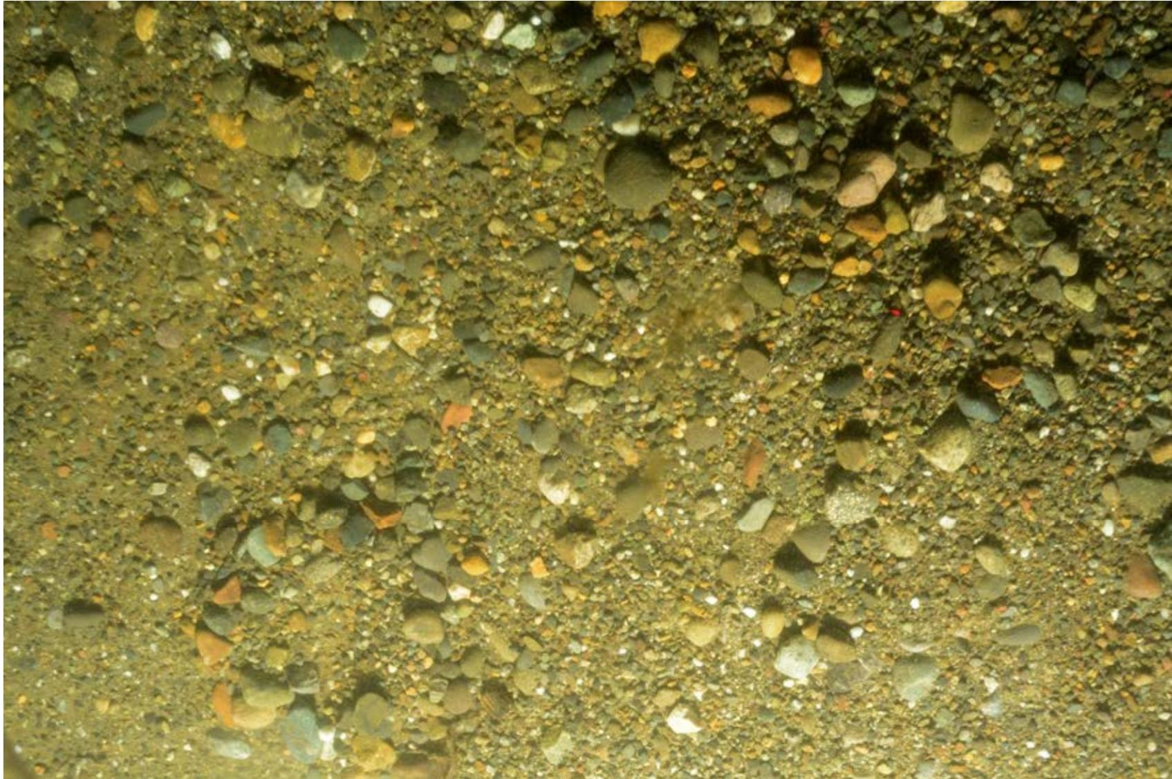
Figure 3-9. PV image from Station LDW-Y0-SC-ENR-2-B-PV-R1 showing typical ENR sediments from the scour ENR subplot. ENR materials are lithic sands and gravels. The sediment surface is mostly free of fine-grained sediment. Scaling lasers (red dots) are 26 cm apart.
