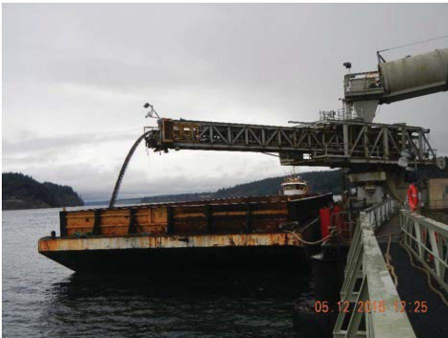
**2016-12-05 11.25.40** Bow of KP-3 barge being loaded with Gravelly Sand ENR material at CalPortland's DuPont dock with conveyor near full extension.
