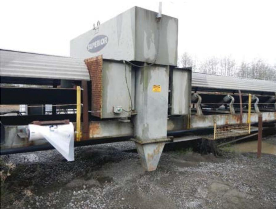
**2016-11-23 08.59.33** Cross section sampler used to collect samples directly off the conveyor. Volume of each sample is approximately two gallons.
