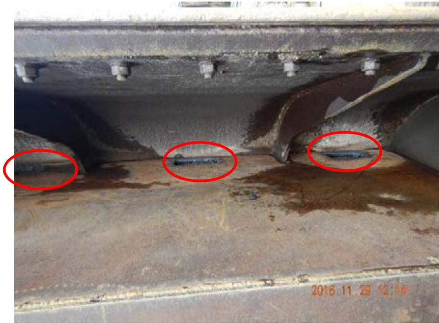
Photo 15 Three vents cut into baffles to allow bucket to vent freely.
