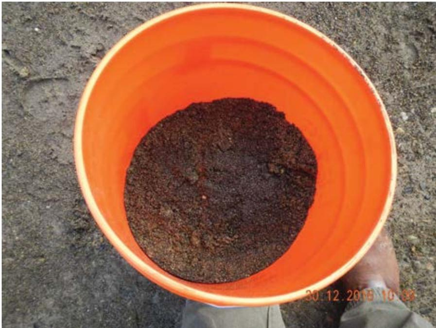
**2016-12-30 10.09.31** ENR+AC sample representing the 1,000 to 1,500 ton interval prior to homogenizing.
