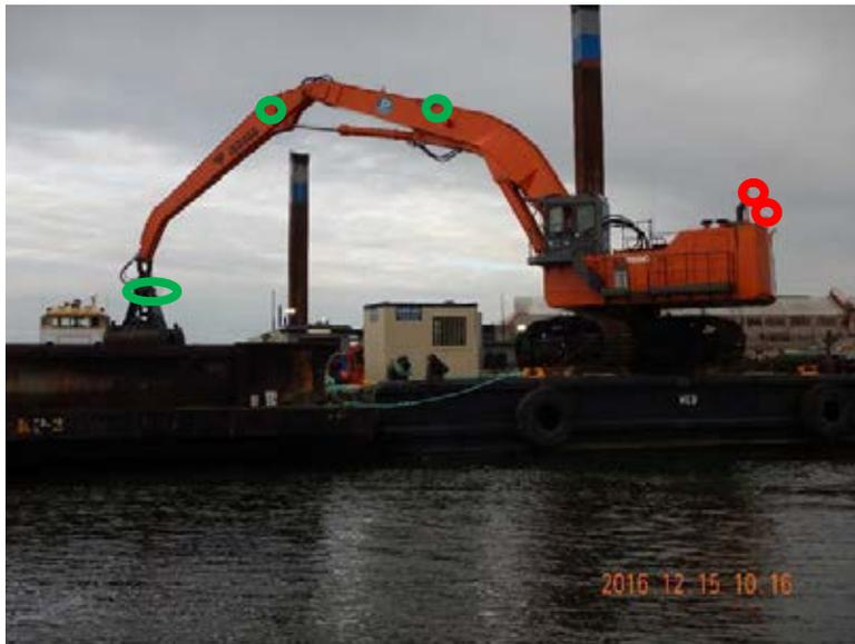
Photo 18 Excavator taking from the material barge. GPS antennas and sensors used for bucket positioning are circled in red and green, respectively.
