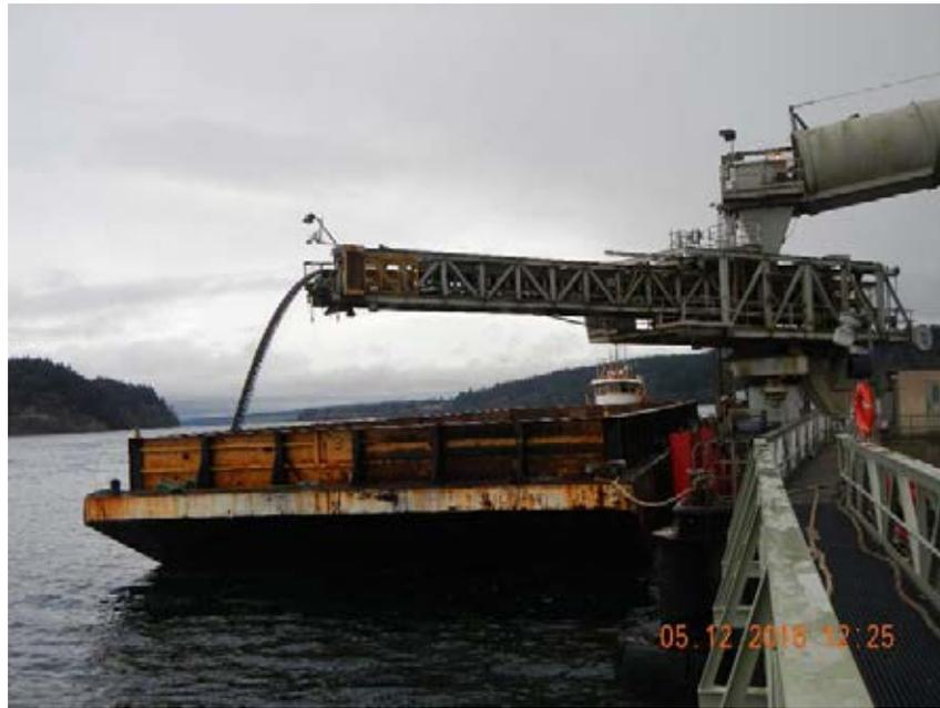
Photo 1 KP-3 barge being loaded with ENR material at CalPortland's Pioneer Aggregates barge-loading dock.
