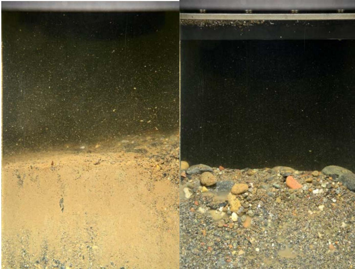
Figure 3-5. Representative SPI images from LDW-Y0-IN-ENR+AC-6-A-SPI-R1 and LDW-Y0-IN-ENR+AC-3-B-SPI-R3 showing the variability in recent deposition observed. At LDW-Y0-IN-ENR+AC-6-A-SPI-R1, there is abundant recent deposition that has been smeared down. At LDW-Y0-IN-ENR+AC-3-B-SPI-R3 there is only a trace amount of post-placement recent deposition. SPI images are 14.42 cm in width.
