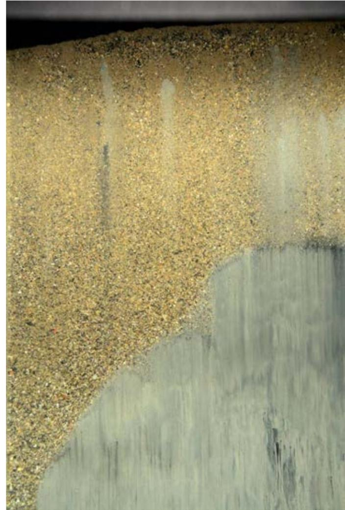
Figure 3-18. Representative SPI images from Stations LDW-Y0-SU-ENR+AC-4-B-SPI-R1 (left) and LDW-Y0-SU-ENR+AC-4-B-SPI-R1 (right) from the subtidal ENR+AC subplot. ENR+AC material overlies gray, reduced native sediments providing 100% cover. These are the only two replicates from this subplot (from the same station) where the ENR+AC thickness is less than prism penetration. SPI images are 14.42 cm in width.
