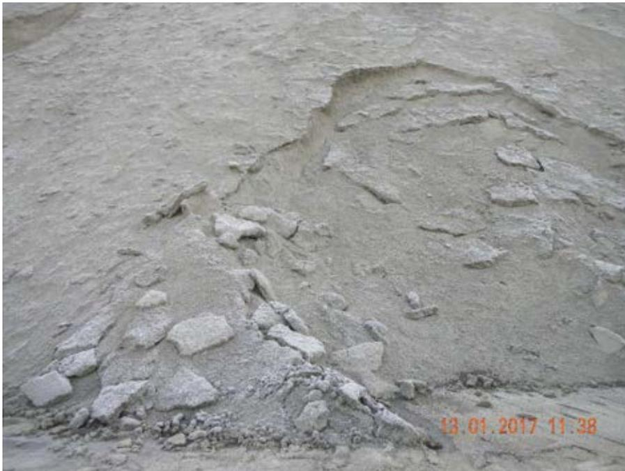
**2017-01-13 11.38.46** Clumps of frozen sand at the stockpile caused loading of the KP-3 barge to be interrupted several times. The clumps would get caught in the bars of the grizzly; effectively blinding off the hopper below until removed.
