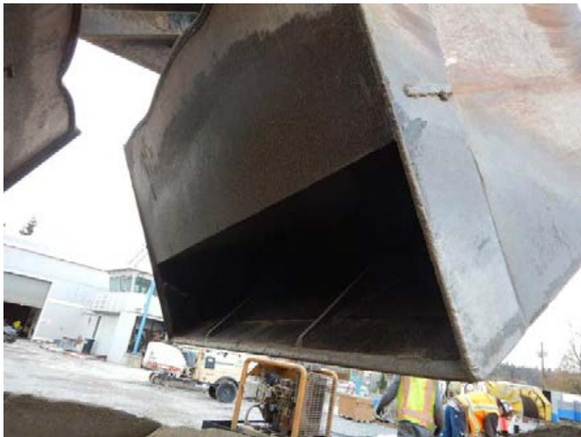
Photo 8 Baffle welded into right half of bucket to reduce bucket volume.
