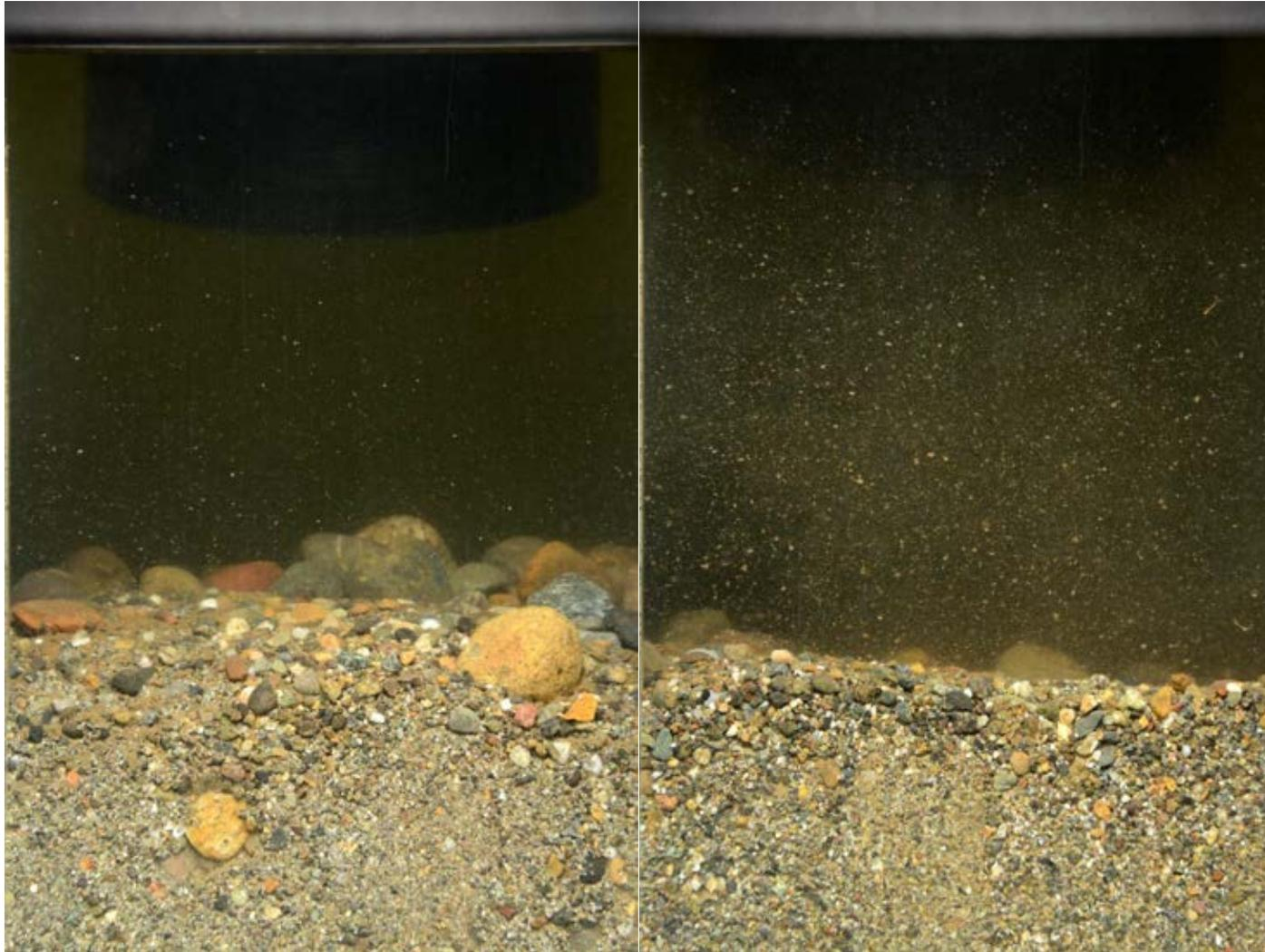
Figure 3-1. Representative SPI images from Stations LDW-Y0-IN-ENR-2-B-SPI-R1 (left) and LDW-Y0-IN-ENR-4-B-SPI-R1 (right) showing ENR sands and gravels typical of the intertidal ENR subplot. SPI images are 14.42 cm in width.
