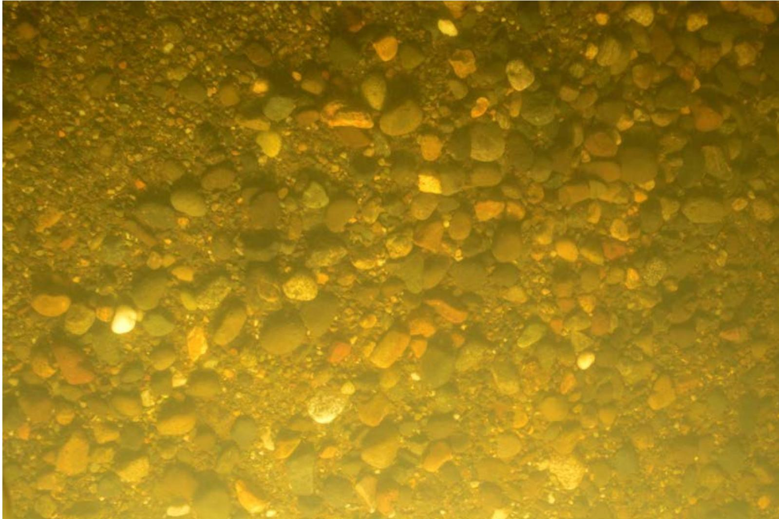
Figure 3-2. Representative PV image from Station LDW-Y0-IN-ENR-3-A-PV-R1 showing ENR sands and gravels typical of the intertidal ENR subplot at 100% cover.
