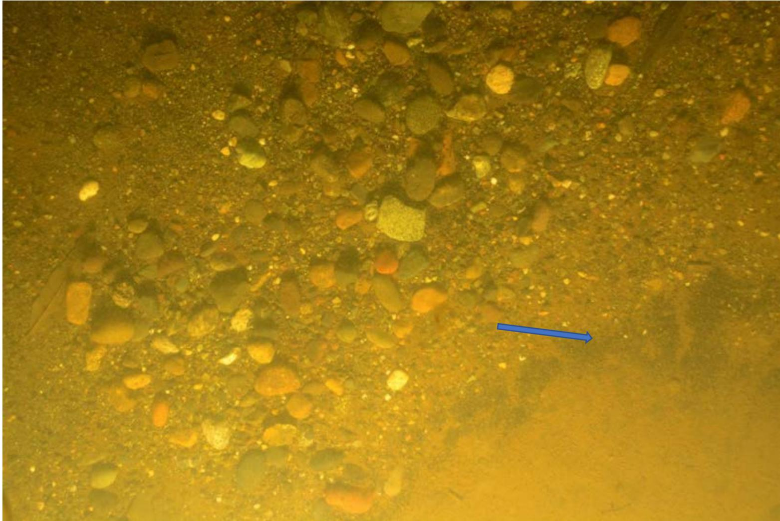
Figure 3-7. Representative PV image from Station LDW-Y0-IN-ENR+AC-6-A-PV-R1 showing ENR+AC sands and gravels from the ENR+AC subplot. Small sand-sized black particles can be seen at the sediment surface and in a band at the lower right. At this station and replicate, there are patches of recently deposited fine-grained sediment that obscure the ENR+AC material (lower right). Scaling lasers (red dots) are 26 cm apart.
