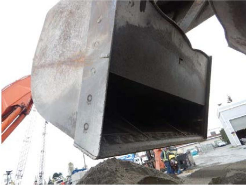
Photo 7 Baffle welded into left half of bucket to reduce bucket volume.
