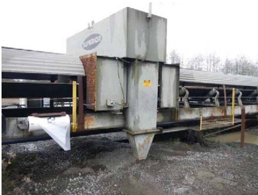
Photo 6 Belt cut sampler used to collect an approximate 2-gallon cross-section sample of ENR+AC directly from the belt.
