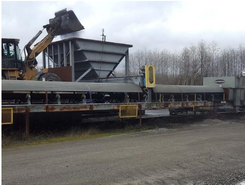
Photo 3 Hopper and auger used for blending AC with ENR material.
