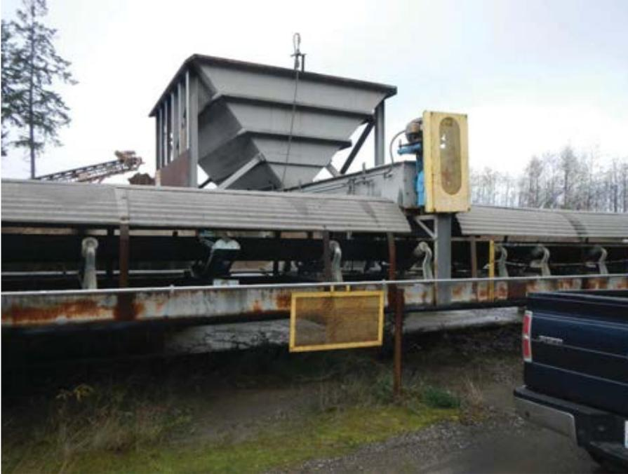
**2016-11-23 09.23.29** AC hopper and auger which delivers AC to ENR material. ENR and AC are blended as both materials pass through transition points while enroot to the loading wharf.
