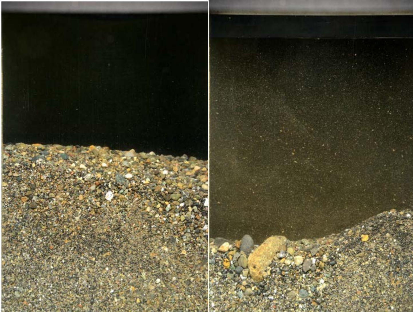
Figure 3-4. Representative images from Stations LDW-Y0-IN-ENR+AC-1-B-SPI-R3 and LDW-Y0-IN-ENR+AC-5-B-SPI-R3 that show ENR+AC sediments from the intertidal plot. SPI images are 14.42 cm in width.
