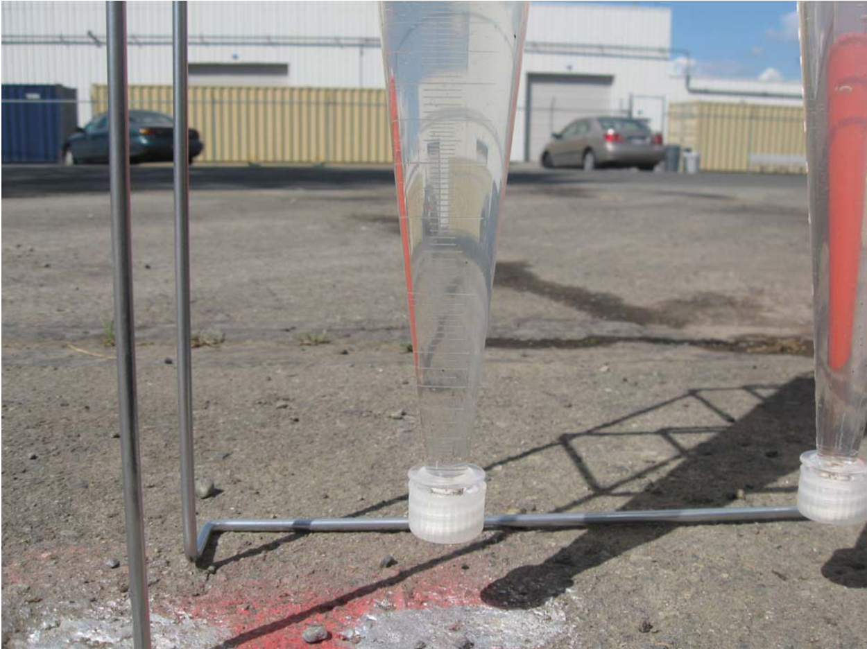
Close up of Imhoff test on stormwater stored in Baker tank.
