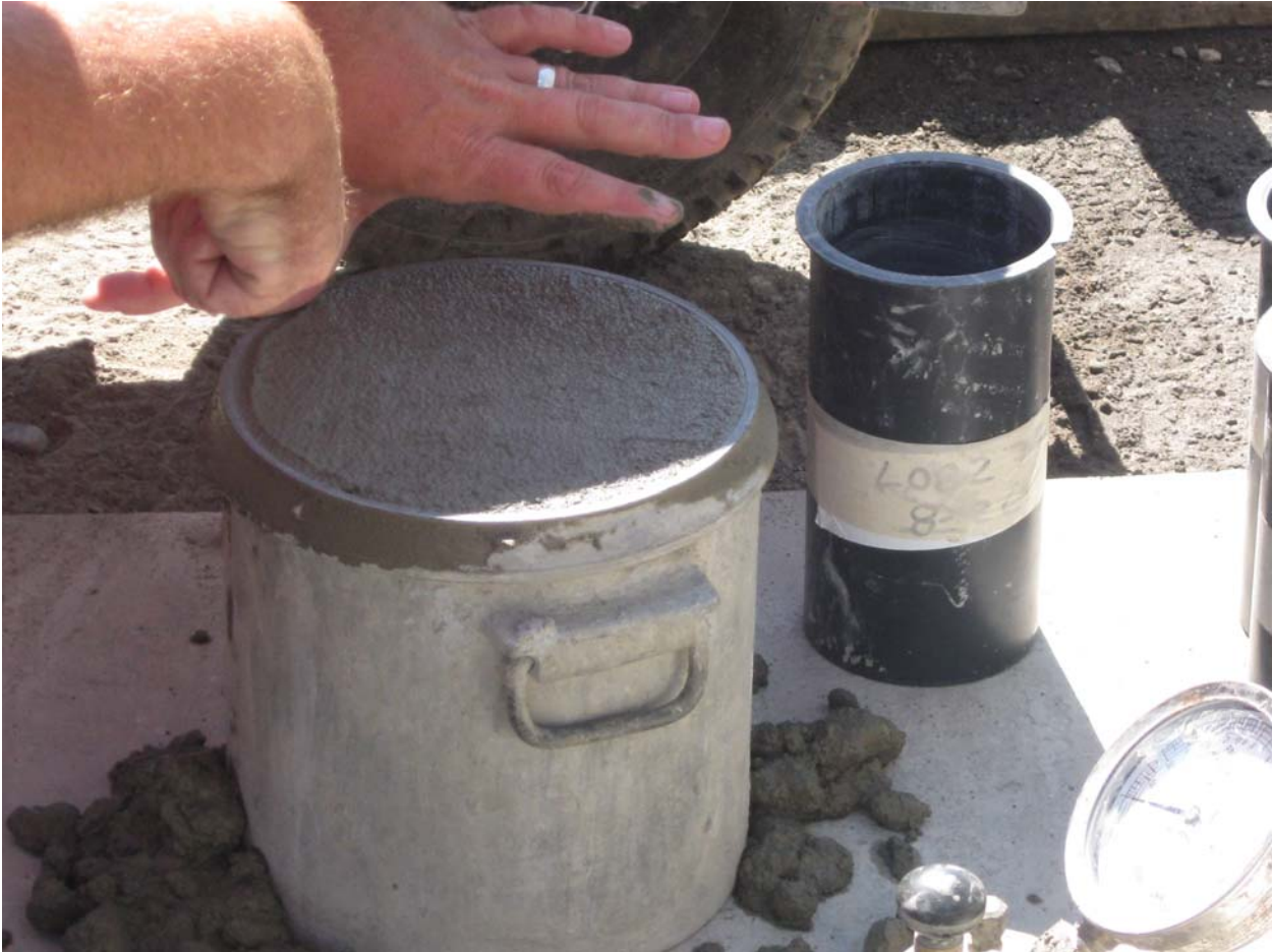
Preparing air content test specimen.
