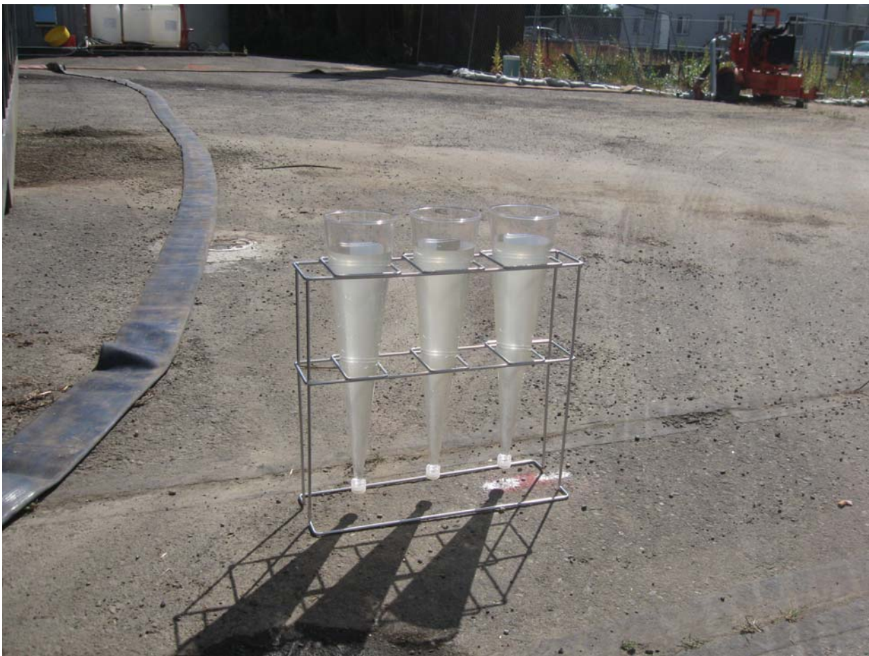
Imhoff test on stormwater stored in Baker Tank.
