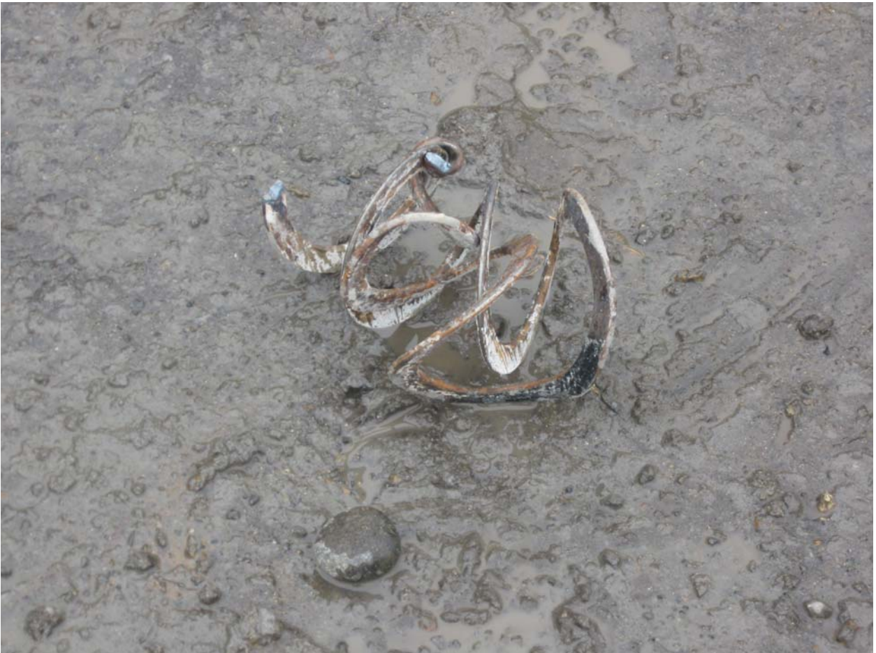
Example broken bentonite delivery system auger.
