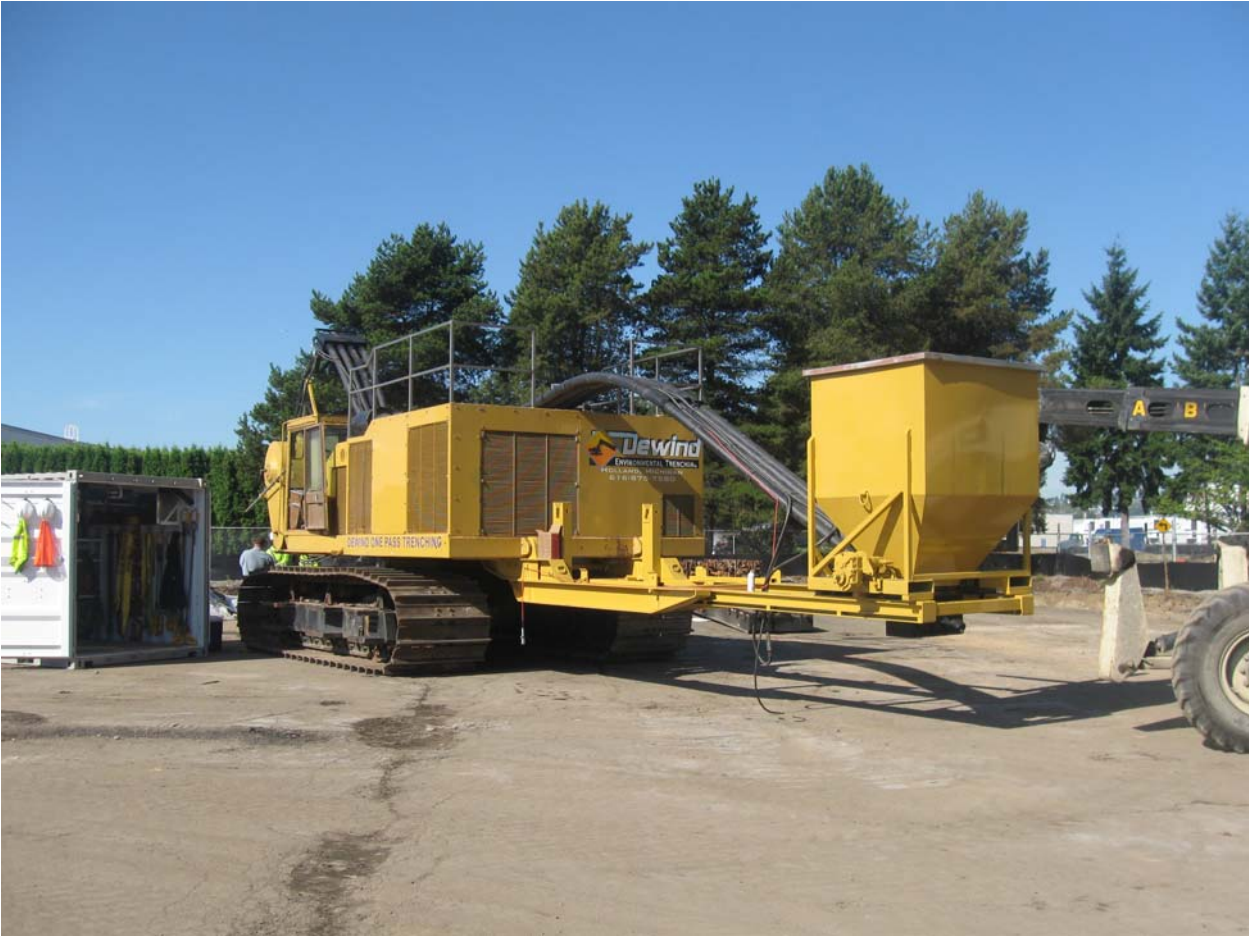
DeWind Trencher being assembled.
