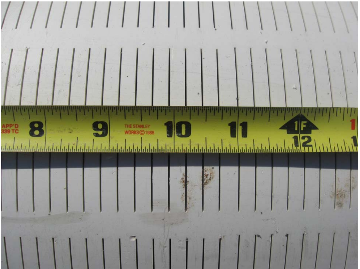
Slotted 12-inch diameter PVC well casing.
