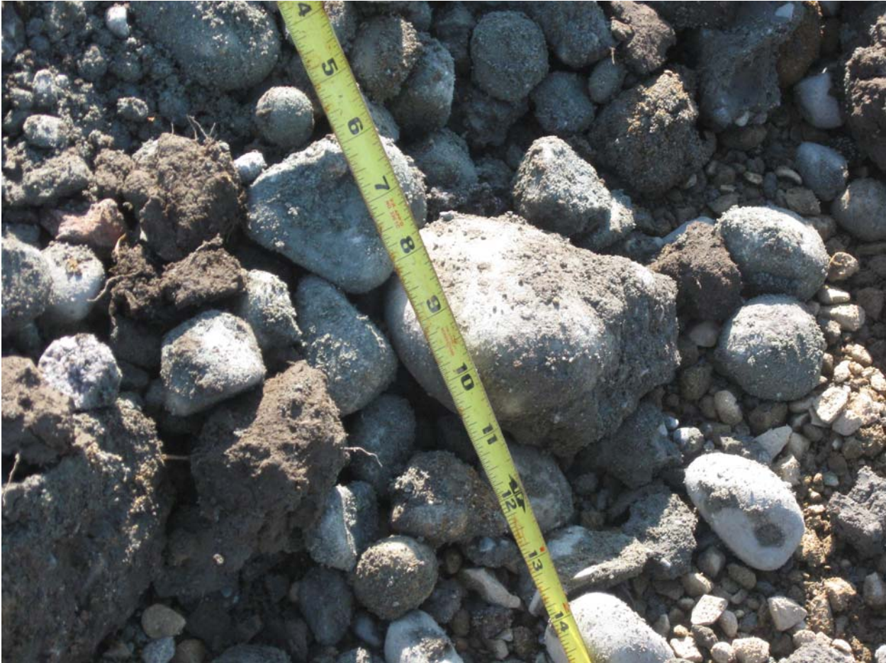
Typical gravel and cobble fill below 30 inches depth in the exploratory trench.
