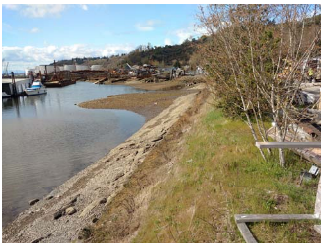
View Looking North Depicting High Tide Line Approximately 4 Feet Below Property Ground Surface
