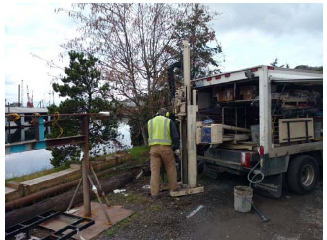
Direct Push Drilling at SB08 Location
