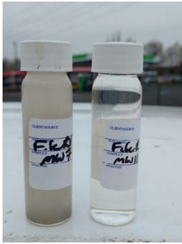
Example of Water from an Undeveloped Well (left) and an Aerotech-Developed Well (right)
