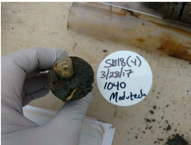
Fill at SB18 Location with Copper Wire
