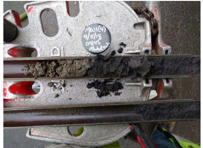
Fill from 0 to 4 Feet Below Ground Surface, followed by Water-Bearing Sand at MW1 Location
