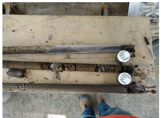
Profile from the SB12 Location. Fill present from 0 to 12 feet Below Ground Surface then by Silt and Sand
