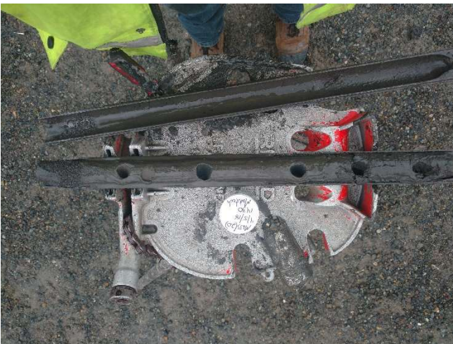
Silt with Clay and Intermittent Water Bearing Sand Lenses
