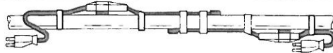
*When using 2 cables, overlap cables with overrun zone on opposite sides of pipe.
