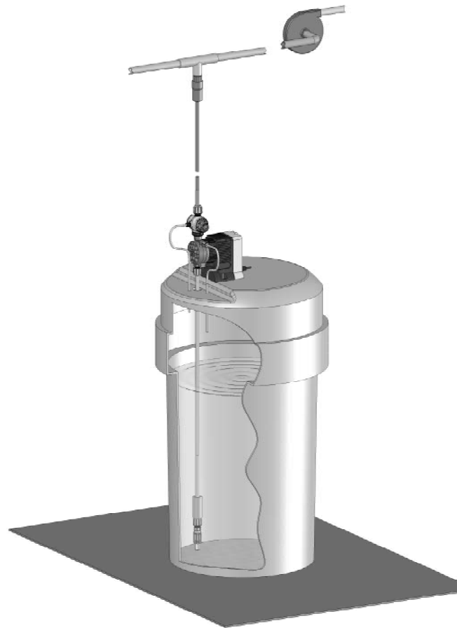
4-FV prevents syphoning when pumping into a vacuum such as the suction side of a recirculating pump.
