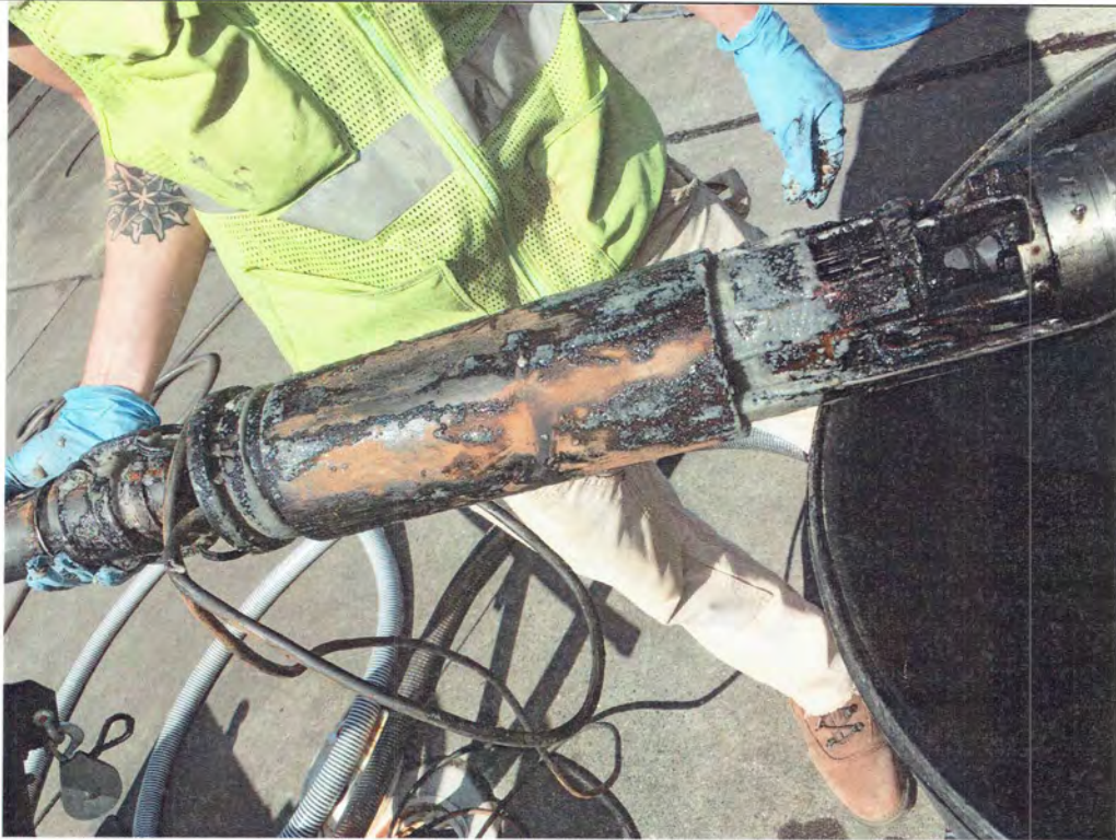
Photograph 5, extraction pump with biological growth and iron scale
