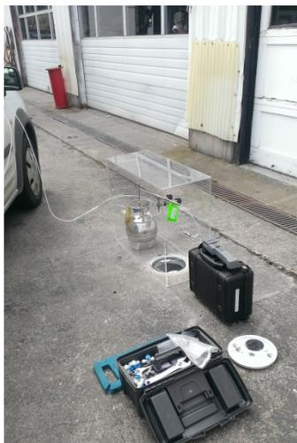
Photograph 3. Setting up soil gas sample Soil Gas 03.
