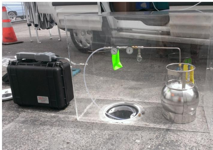
Photograph 4. Sample train for soil gas sample Soil Gas 03.
