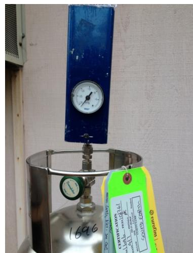
Photograph 6. Flow controller on summa canister used for collecting integrated air samples.
