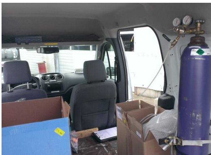
Photograph 5. Helium gas introduced to sample train as a leak detection tracer compound.
