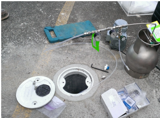
Photograph 3. Setting up soil gas sample Soil Gas_03.
