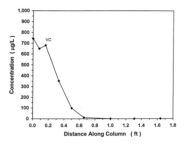
Figure 3: Steady state VC concentration profile versus distance along the bench-scale column.
