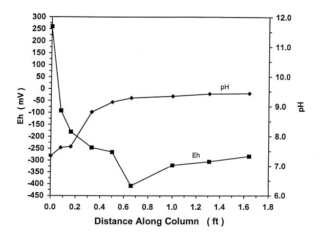
Figure 4: Steady state Eh/pH profiles versus distance along the bench-scale column.
