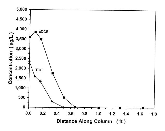
Figure 2: Steady state TCE and cDCE concentration profiles versus distance along the bench-scale column.
