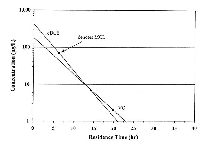
Figure 8: First-order kinetic model results for TCE, cDCE, and VC using anticipated field half-lives and low concentration scenario
