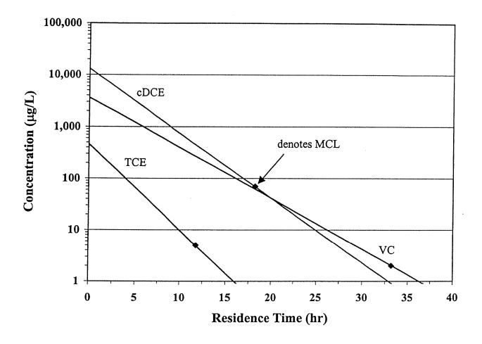
Figure 7: First-order kinetic model results for TCE, cDCE, and VC using anticipated field half-lives and high concentration scenario.
