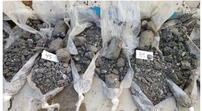
Photograph 2. Sonic core of injection well IW01 from approximately 15 to 25 feet bgs.
