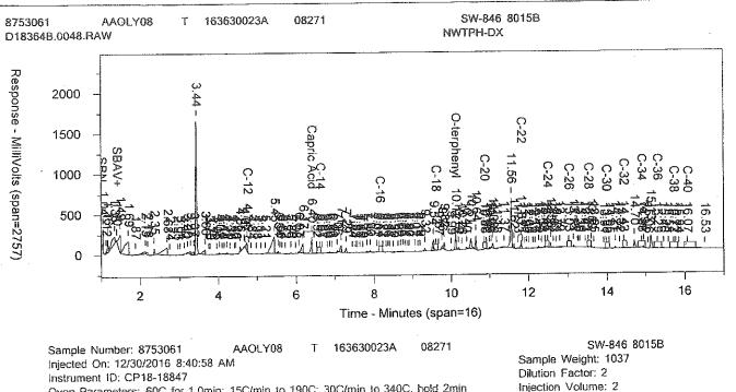
Oven Parameters: 60C for 1.0min; 15C/min to 190C; 30C/min to 340C, hold 2min GC Column: HP-5 30m x 0.32mm x 0.25um
