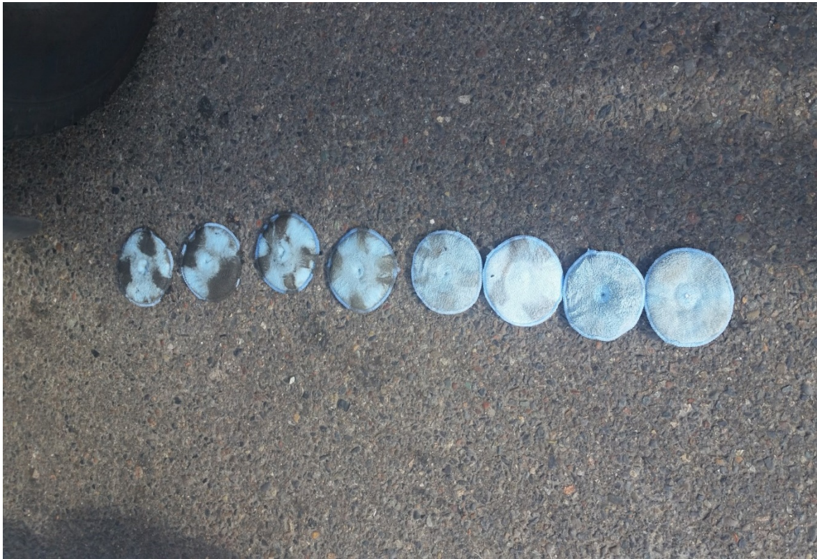
Progression of MW-8 cleaning pads on June 5, 2018.
