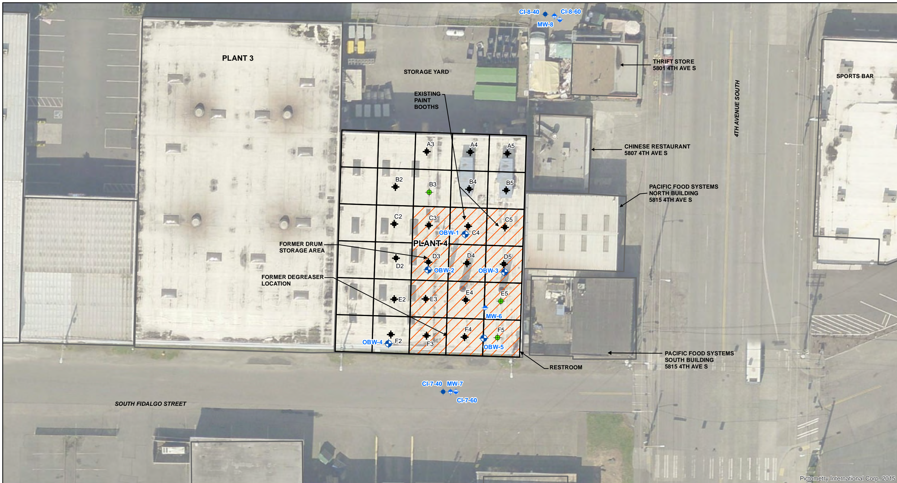
FIGURE 5 PLANT 4 ISCO INJECTION POINTS AND MONITORING WELLS WEST OF 4TH GROUP SITE CAPITAL INDUSTRIES, INC. 5815 4TH AVENUE SOUTH SEATTLE, WASHINGTON FARALLON PN: 457-008
