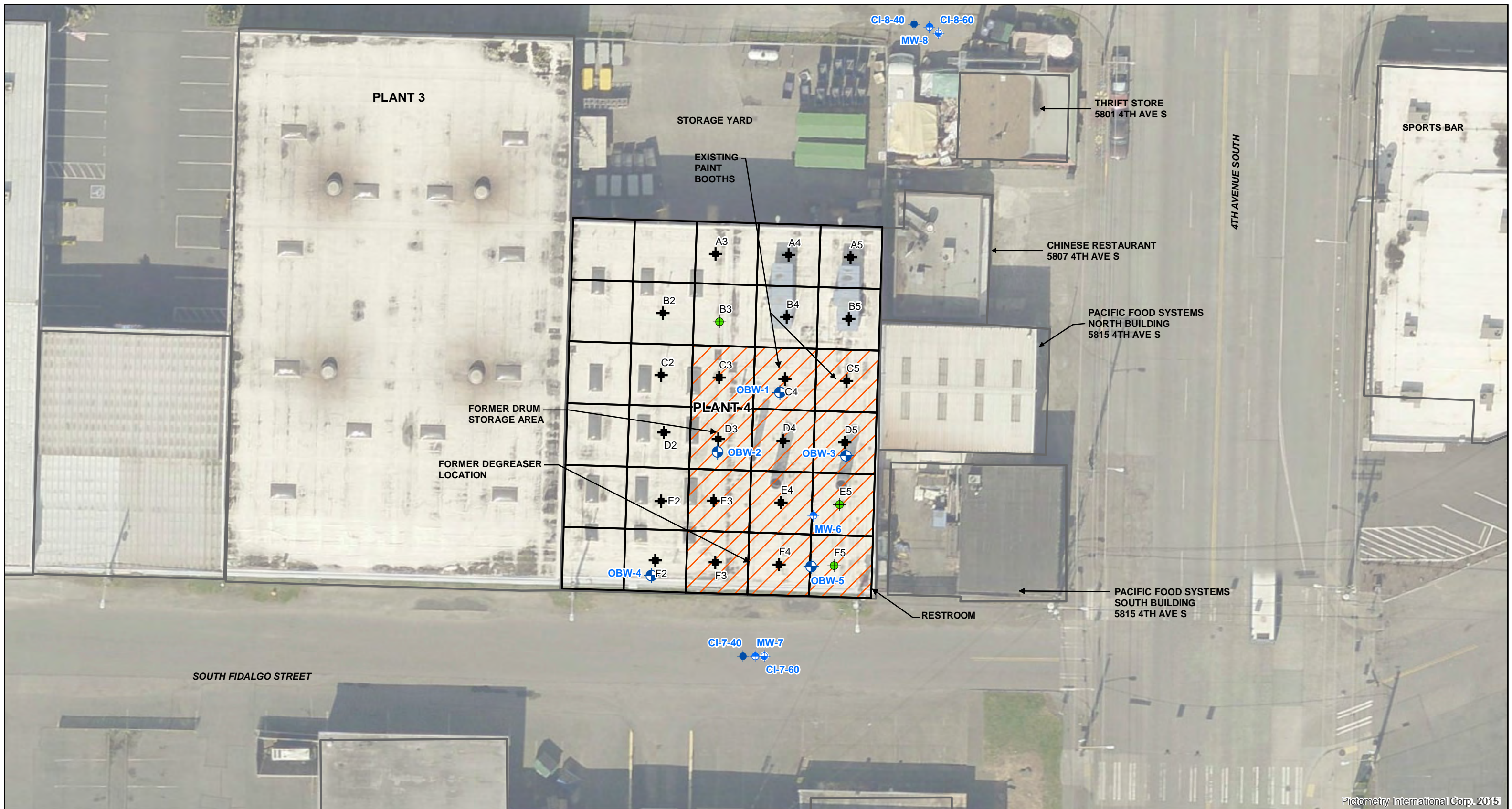
FIGURE 3 PLANT 4 ISCO INJECTION POINTS AND MONITORING WELLS WEST OF 4TH GROUP SITE CAPITAL INDUSTRIES, INC. 5815 4TH AVENUE SOUTH SEATTLE, WASHINGTON FARALLON PN: 457-008 Document Path: Q:\Projects\457 CapitalIndust\008 PilotStudy\InterimWorkPlan\Figure 3 ISCO InjectionPoints_PMW_SAP.mxd
