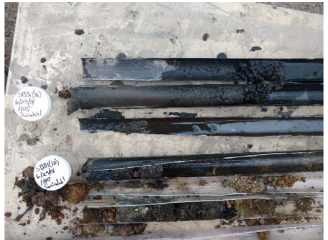
Samples from SB31 where dark oily sheen, stain and odor were observed
