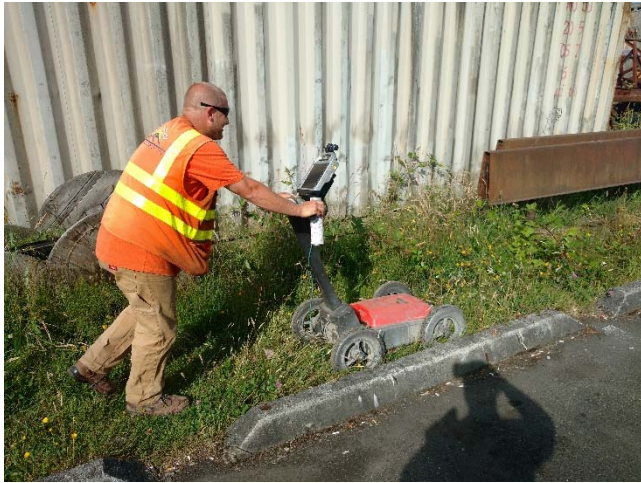
GPR survey prior to drilling
