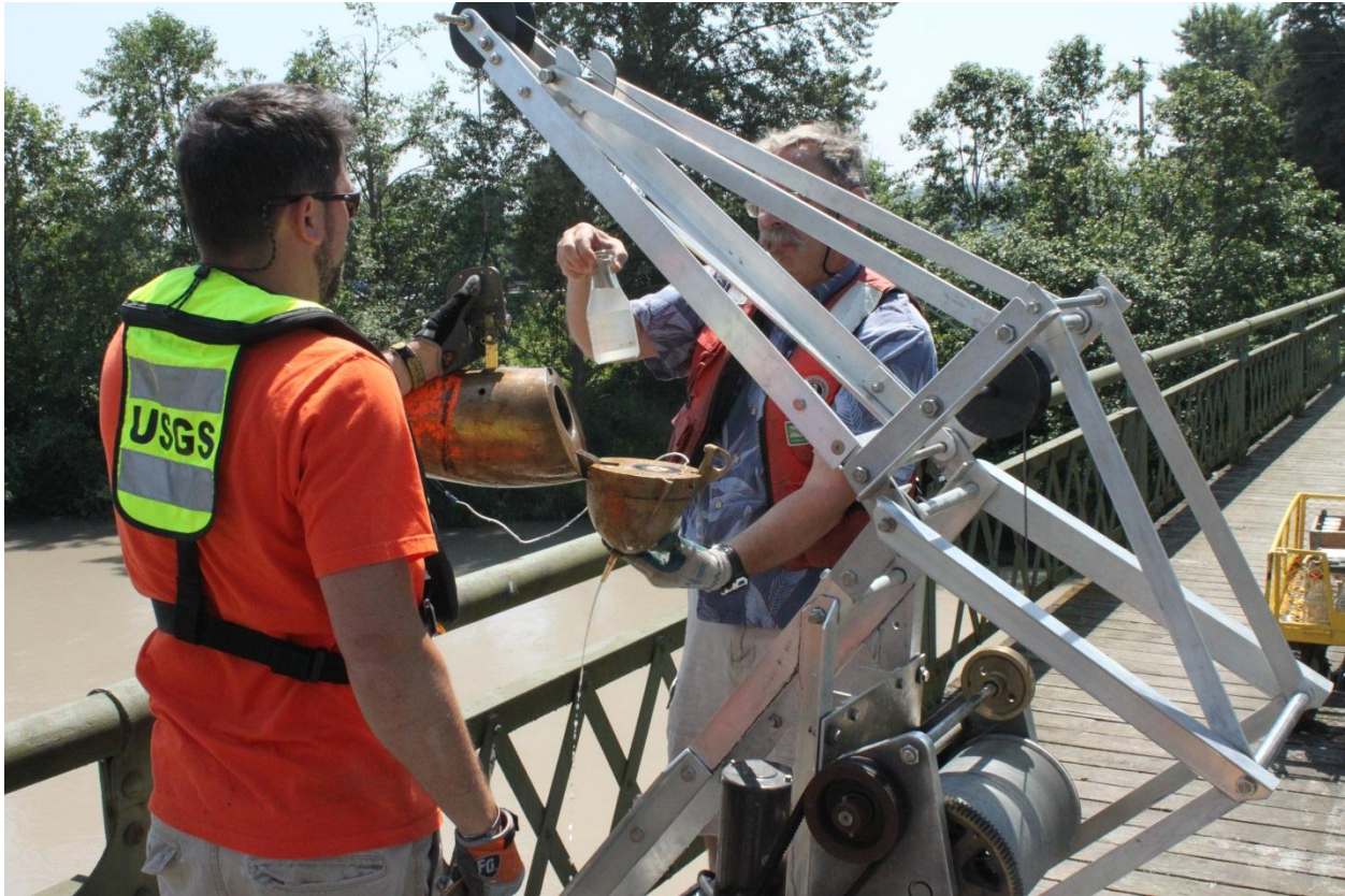
Figure 3. Photo of example USGS sampling equipment, including a crane, reel, and sampler for representative collection of depth- and width-integrated samples.
