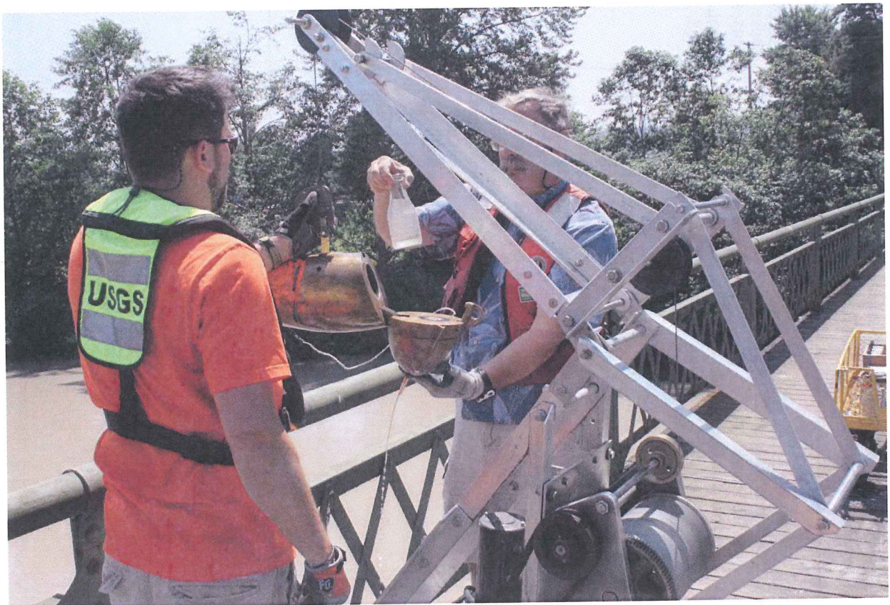
Figure 4. Photo of example USGS sampling equipment, including a crane, reel, and sampler for representative collection of depth- and width-integrated samples.
