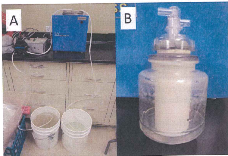
Figure 5. Flow-through centrifuge set-up (a) and centrifuge bowl (b).
