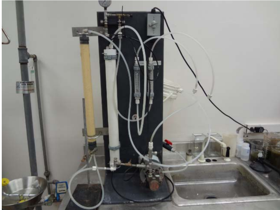
FIGURE 2-3. ION EXCHANGE AND RO TEST APPARATUS
