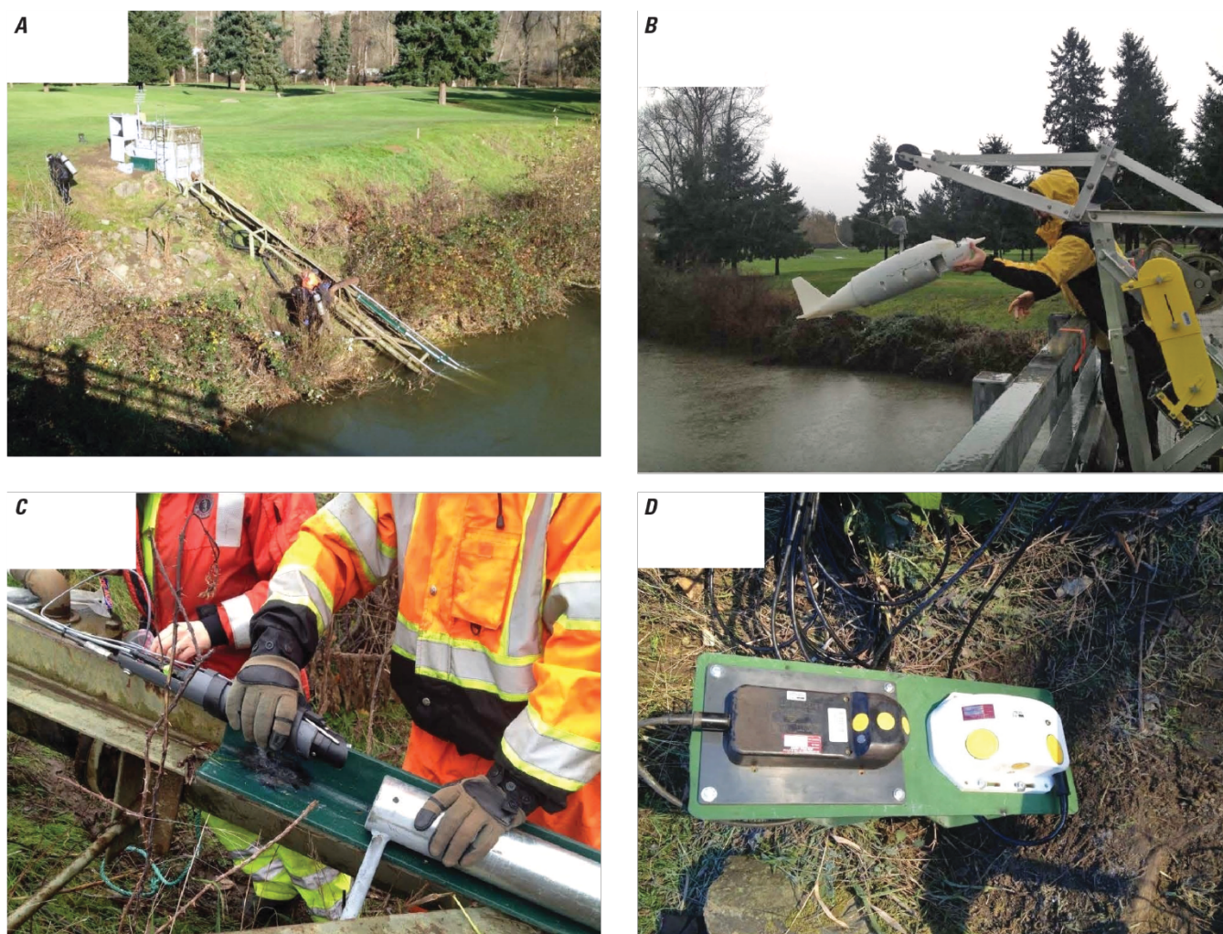
Figure 3. Photographs of (A) U.S. Geological Survey streamgage 12113390 (Duwamish River at Golf Course at Tukwila, Washington), (B) US D-96 sampler for suspended-sediment water samples, (C) turbidity sensor, and (D) two acoustic Doppler velocity meters. Modified from Conn and Black (2015).
