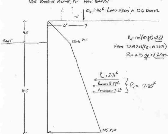
IF THE TRENCH WAS LOWNED along South SIDE of RIVER BRIVE WITHIN 6'OF 1570RY W/F HOUSE. The HOUSE WOULD PRODUCE A LINE LOND OF 1000 LB/ ALONG THE TRUNK This Would result in A Resultant Hore. Force of 0.5 Kips & a TOTAL Hire Force of 2.71 (Real) + 3.44(Rome) + 0.5 (Hour surcious) = 6.65 Kips
