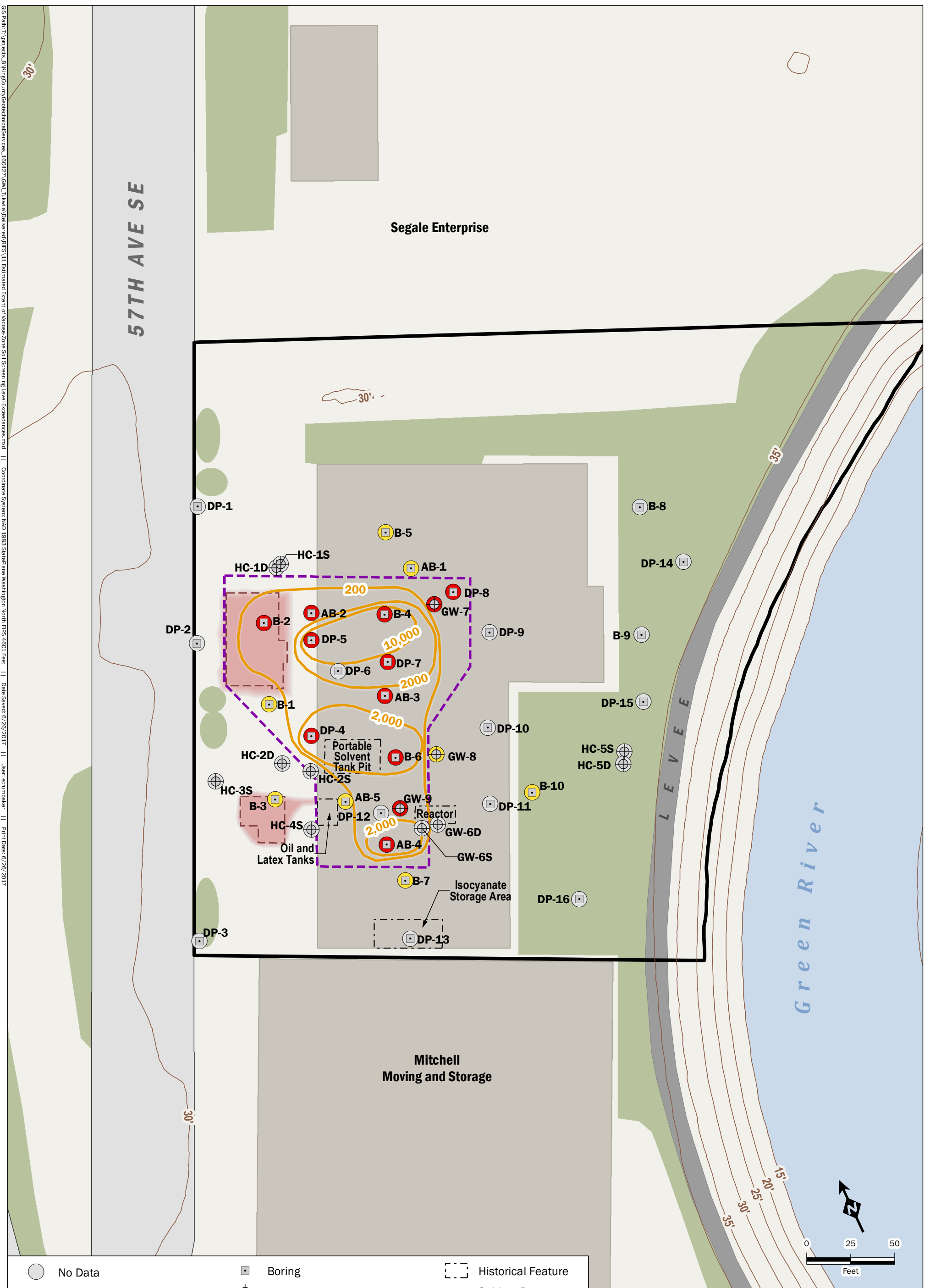
Estimated Extent of Vadose-Zone Soil Screening Level Exceedances Remedial Investigation and Feasibility Study GWI Tukwila Property 18700 Southcenter Parkway Tukwila, Washington
