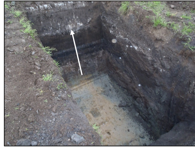
Photo 2. A view of Plot 15 Test Pit 2. Note the salt-and-pepper strata at 2 ft (arrow).
