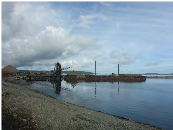
Comment: Loading EMNR material on barge with conveyor belt
