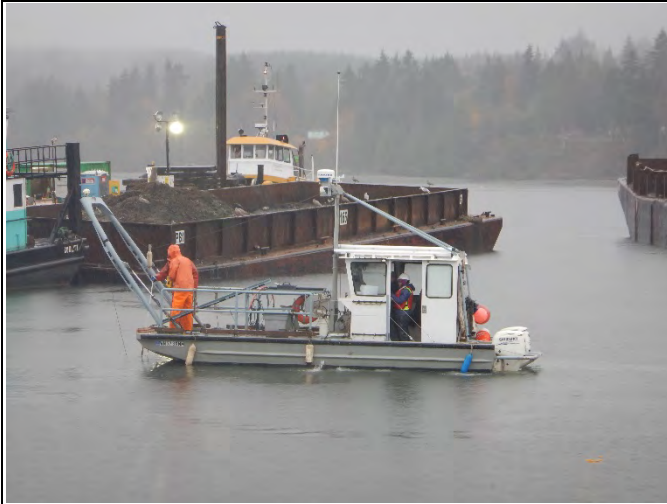
Comment: Collecting confirmatory sediment cores
