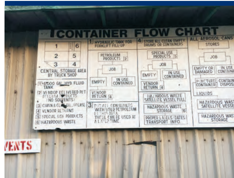
Photo 44 Sign on south side of hazardous material storage shed, showing storage organization and handling decision tree.
