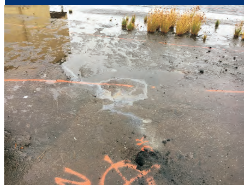
Photo 14 Sheen coming from dirt that came up in sample core from FC03.
