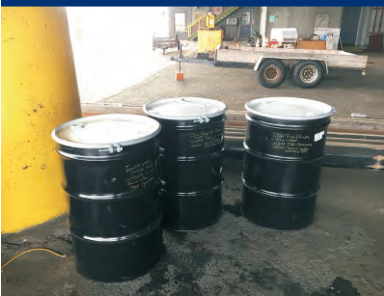
Photo 41 Labeled IDW drums, stored under cover.
