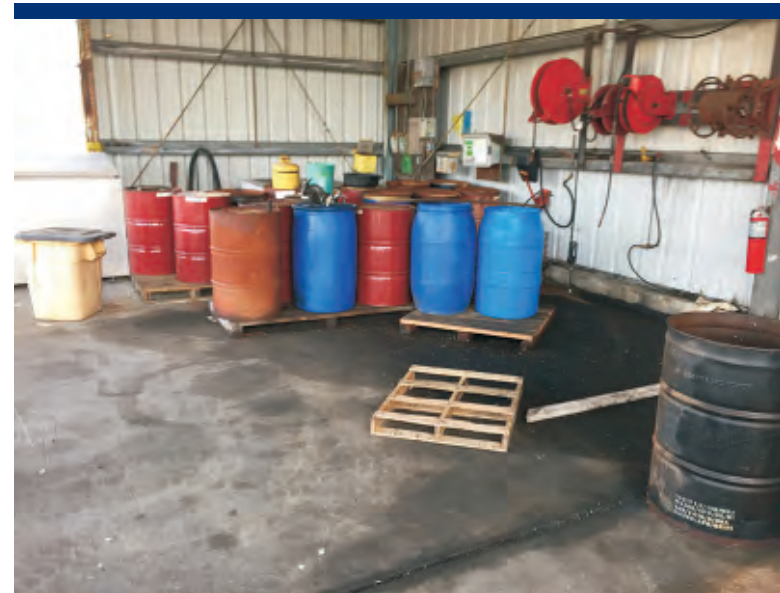
Photo 28 Drums and stained concrete within fuel and chemical storage building. All drums checked were not empty.
