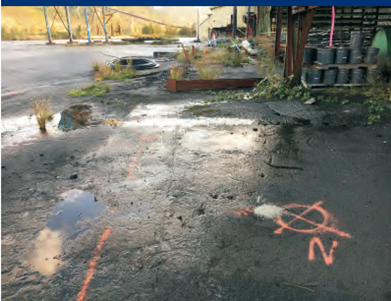
Photo 13 Boring location FC03, patched.
